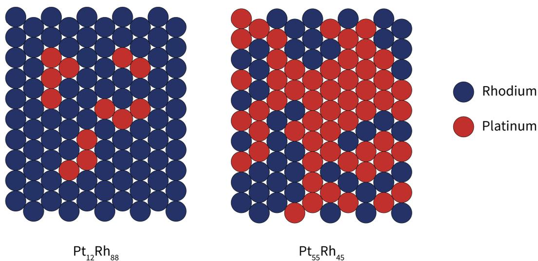
Fig. S7: 2D visualizations of the studied Pt<sub>12</sub>Rh<sub>88</sub> and Pt<sub>55</sub>Rh<sub>45</sub> nanoparticles.
