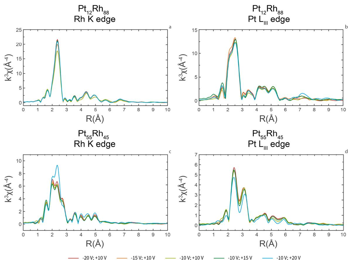
Fig. S1: EXAFS functions in R-space for the Rh K edge of Pt<sub>12</sub>Rh<sub>88</sub> particles (a), the Pt L<sub>III</sub> edge of Pt<sub>12</sub>Rh<sub>88</sub> particles (b), the Rh K edge of Pt<sub>55</sub>Rh<sub>45</sub> particles (c) and the Pt L<sub>III</sub> edge of Pt<sub>55</sub>Rh<sub>45</sub> particles (d), prepared at various potentials.
