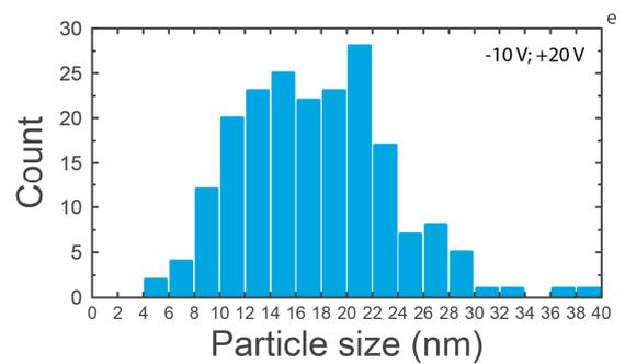
Fig. S5: Particle size distributions for studied Pt<sub>55</sub>Rh<sub>45</sub> nanoparticles.
