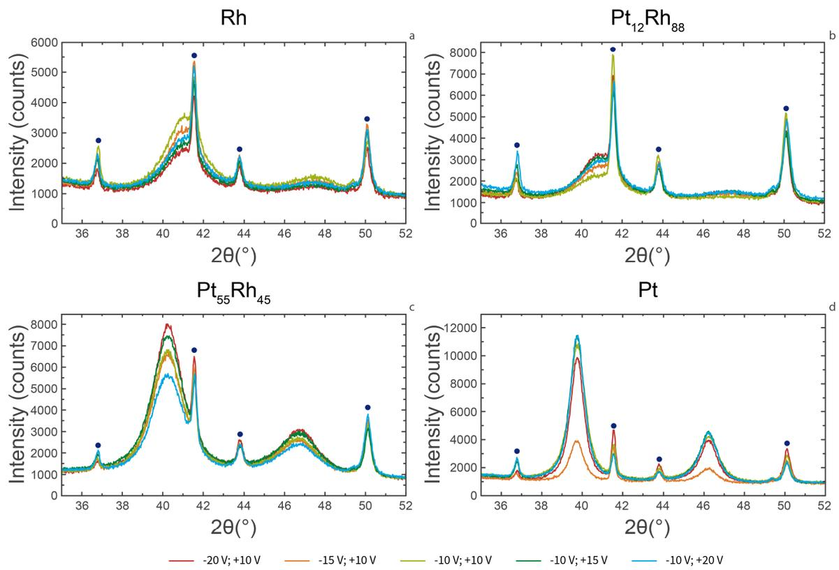
Fig. S2: X-ray diffraction patterns of Rh (a), Pt<sub>12</sub>Rh<sub>88</sub> (b), Pt<sub>55</sub>Rh<sub>45</sub> (c) and Pt (d) particles, prepared at various potentials. Peaks marked with a circle correspond to boron nitride reflections.
