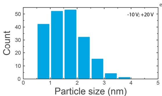
Fig. S3: Particle size distributions for studied Rh nanoparticles.
