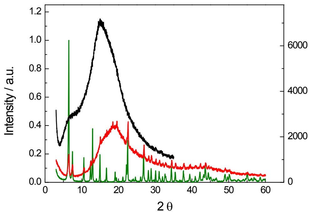
**Figure S4.** X-ray diffraction patterns of polycarbonate PC (black line), C153@Zr-NDC (green line), and C153@Zr-NDC/PC (red line).
