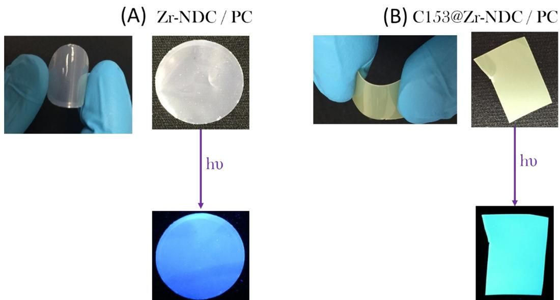
**Figure S3.** Photograph of the physical appearance before and after UV-irradiation of (A) Zr-NDC/PC and (B) C153@Zr-NDC/PC mixed matrix membranes.
