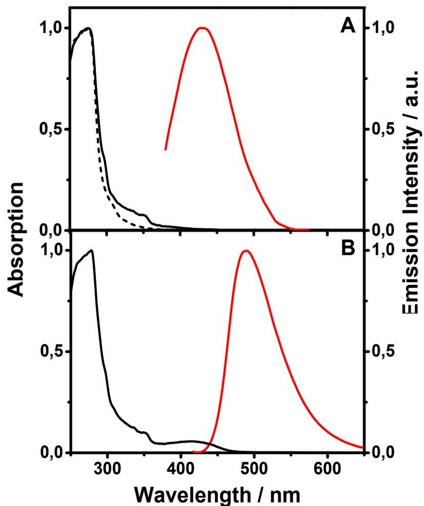
**Figure S5.** Normalized UV-visible absorption (black lines) and emission (red lines) spectra of (A) PC (dashed line) and 2,6-NDC/PC (solid lines), and (B) a mixture of C153/2,6-NDC/PC films. For emission the excitation wavelength was 370 nm.
