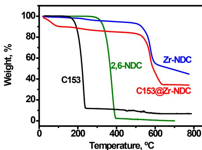
**Figure S1.** TGA curves for the organic linker 2,6-NDC (green), the laser dye C153 (black), Zr-NDC MOF (blue) and C153@Zr-NDC (red) composite material.
