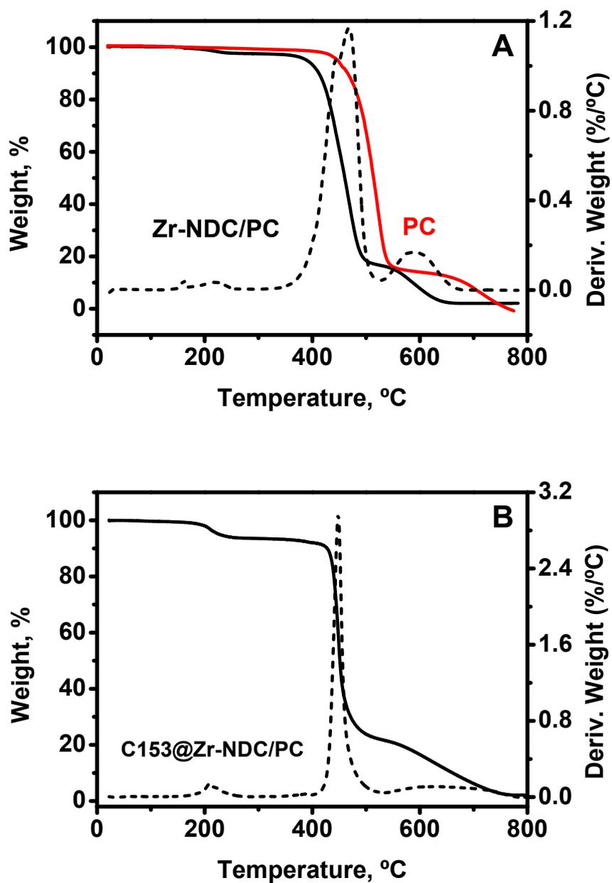
**Figure S2.** TGA curves for A) PC (red) and Zr-NDC/PC (black) films; and for B) C153@Zr-NDC/PC mixed matrix membrane.
