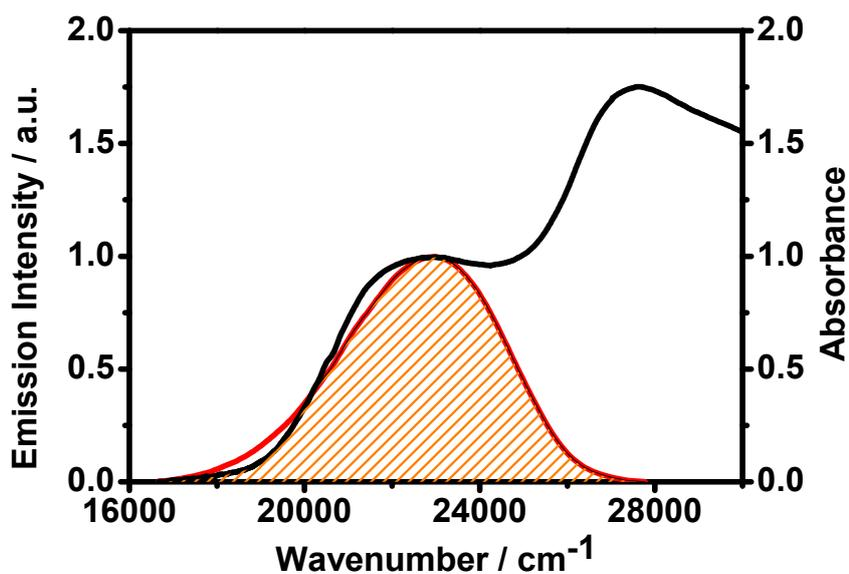
**Figure S6.** Representation of the spectral overlap between Zr-NDC/PC emission (red line) and C153@Zr-NDC/PC absorption (black line). Both spectra are normalized in a way to obtain a similar value at the maxima. For emission, the excitation wavelength was 370 nm.
