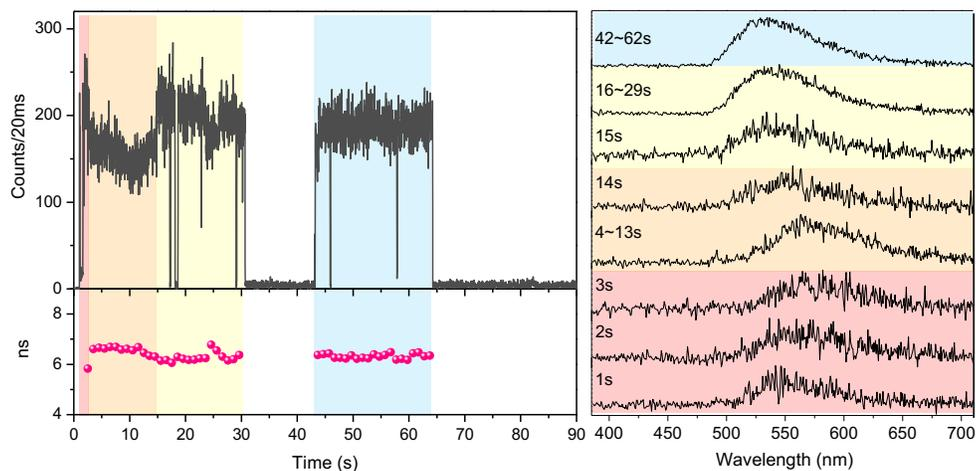
**Figure S3.** An example showing conformational change of a single **LPBI** molecule in hexane with changing the fluorescence lifetime and spectrum according to the fluorescence intensity fluctuations. The ratio of this case is 5.1%, 9.1%, and 12.8% in hexane, and 4.8%, 5.7%, and 6.2% in water for **SPBI**, **MPBI**, and **LPBI**, respectively.
