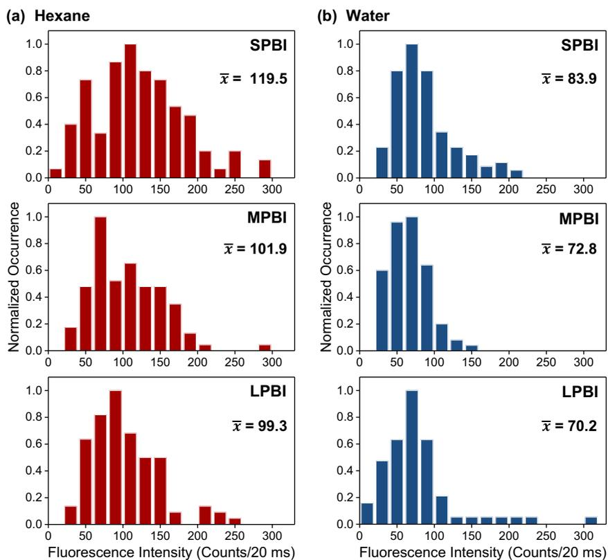
**Figure S4.** Comparison of the brightness of the PBI molecules by calculating the average fluorescence intensity at the first emissive level in their FITs. The brightness of **SPBI**, **MPBI**, and **LPBI** molecules in hexane (a) shows 1.4 times higher fluorescence level than in water (b).
