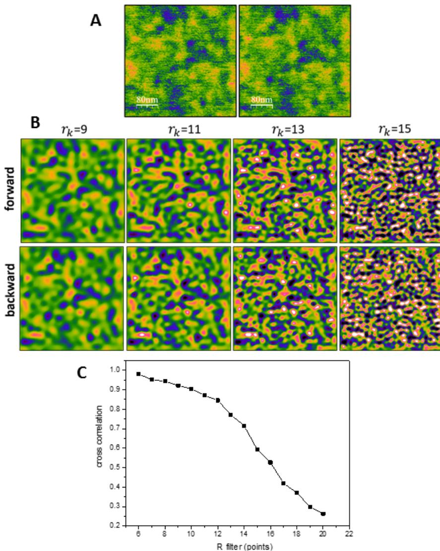
Figure S3: A) Forward and backward  $V_{\text{SKPM}}$  images acquired on PMMA. B) Forward and backward  $q(x, y)$  obtained from A) for different cut-off filter radii. C) Cross-correlation function of the forward and backward  $q(x, y)$  images as a function of the cut-off filter radii.
