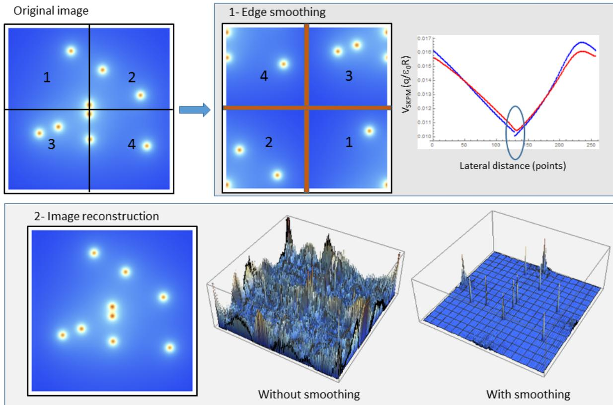
Figure S2: Step by step procedure to smooth the discontinuities at the border of the image. In the bottom panel the  $q(x, y)$  images obtained from the original  $V_{\text{SKPM}}$  without and with edge discontinuities removal are compared.
