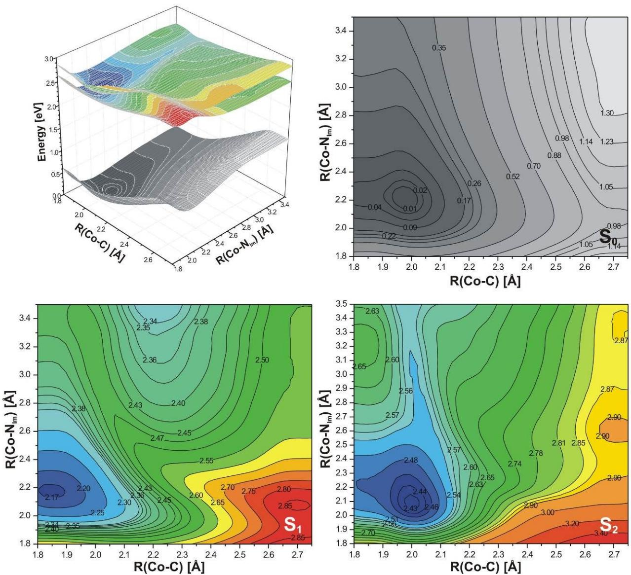
**Figure S2.** Potential energy surfaces (PESs) for ground state and two lowest excited states of Im-[Co<sup>III</sup>(corrin)]-EtPh<sup>+</sup> model complex together with vertical projections of PES for S<sub>0</sub>, S<sub>1</sub> and S<sub>2</sub> electronic states, plotted as a function of axial bond lengths calculated in water solution (COSMO) at BP86/TZVPP level of theory. The vertical projections plots have separate color scales.
