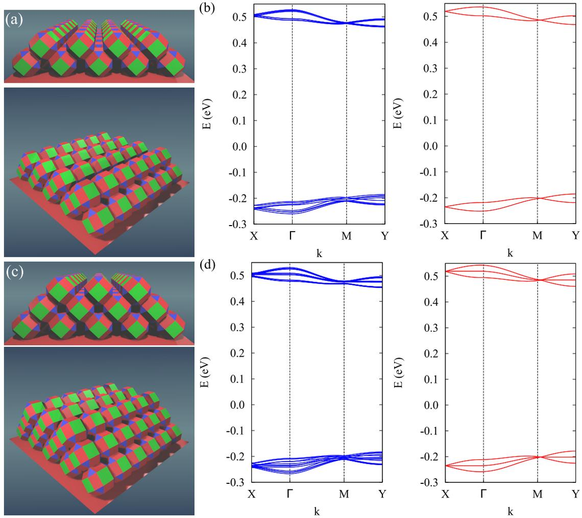
Figure 7: Complex systems that could be synthesized with their corresponding band structures. (a) 2D (110) lattice of NCs that consist of two layers following (110) direction. (c) The three-layer (110) lattice. (b) (d) The electronic band structures for the systems shown in (a),(c), respectively. The calculations are for PbSe and obtained with the atomistic tight-binding method (blue solid line) and with the LEGO Hamiltonian (red solid line).
