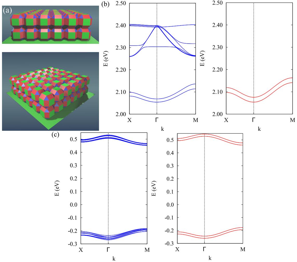
Figure 3: Experimentally synthesized multilayer systems with their corresponding band structures. (a) Bilayer square lattice of NCs that consist of two layers following (100) direction. (b) The electronic band structure of the bilayer square lattice of CdSe NCs obtained with the atomistic tight-binding calculations (blue solid line) and with the LEGO Hamiltonian (red solid line). (c) Same as (b) but for PbSe.
