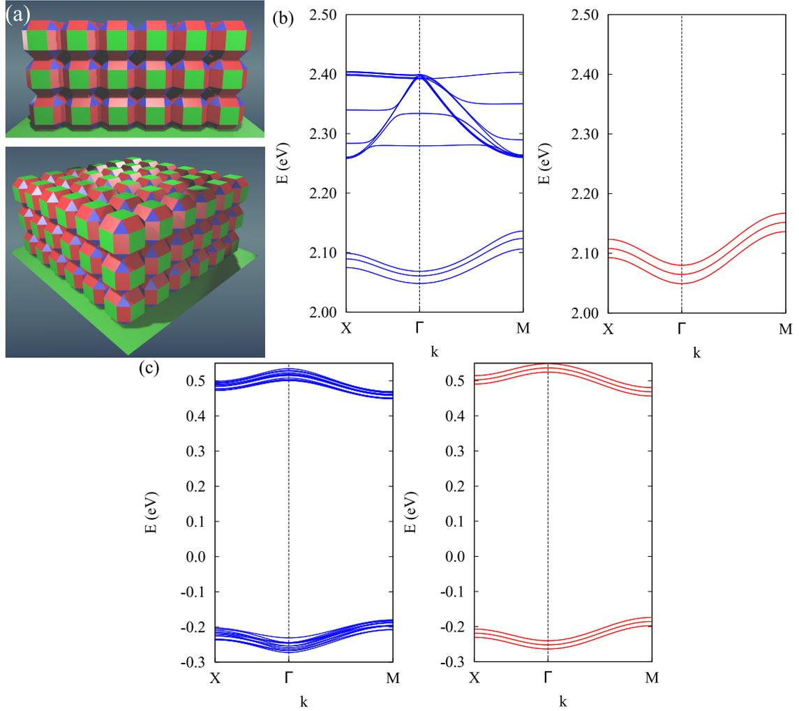
Figure 4: Experimentally synthesized multilayer systems with their corresponding band structures. (a) Trilayer square lattice of NCs that consist of three layers following (100) direction. (b) The electronic band structure of the trilayer square lattice of CdSe NCs obtained with the atomistic tight-binding calculations (blue solid line) and with the LEGO Hamiltonian (red solid line). (c) Same as (b) but for PbSe.
