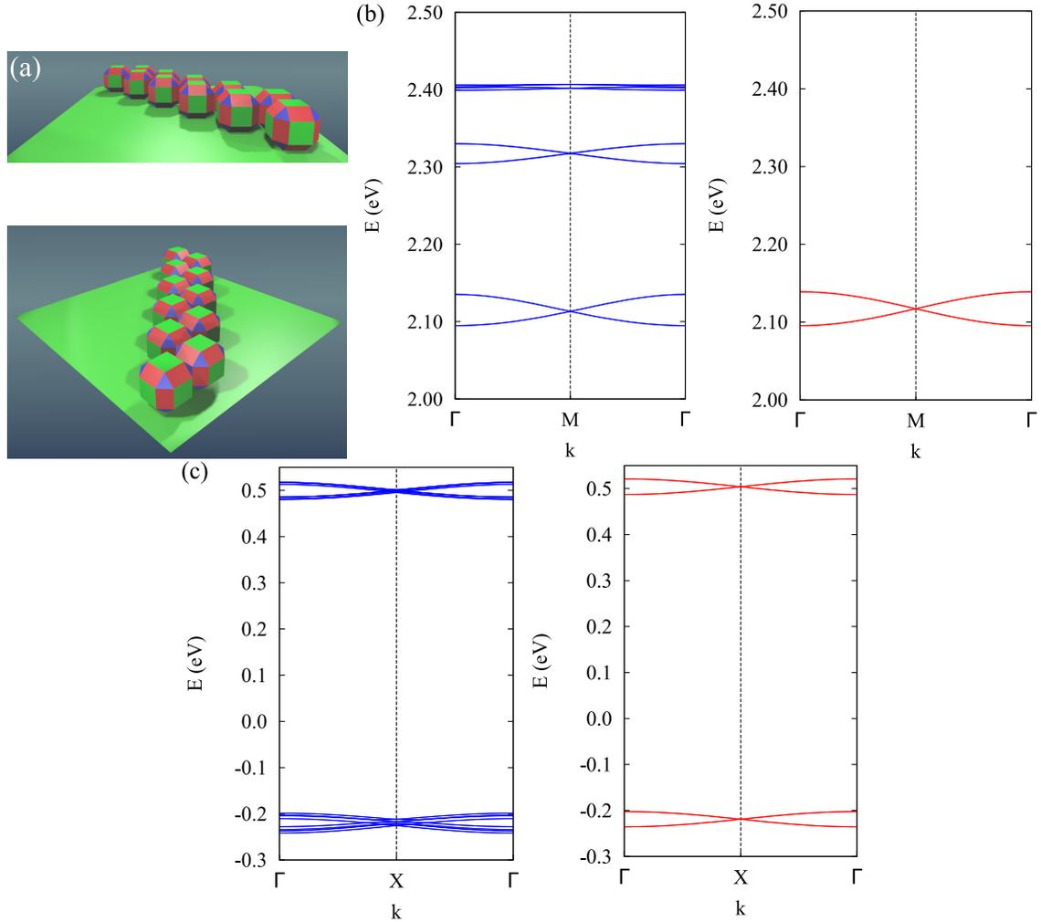
Figure 2: Experimentally synthesized 1D systems with their corresponding band structures. (a) Zigzag chain of NCs along a  $\langle 110 \rangle$  direction. (b) The electronic band structure of the zigzag chain of CdSe NCs obtained with the atomistic tight-binding calculations (blue solid line) and with the LEGO Hamiltonian (red solid line). (c) Same as (b) but for PbSe.
