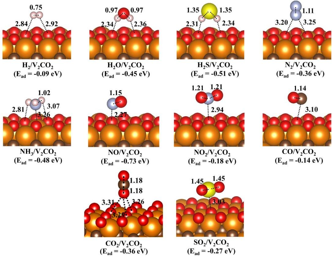
**Fig. S6** The most preferable structures of gas on V<sub>2</sub>CO<sub>2</sub> and E<sub>ad</sub> calculated by PBE-D3
