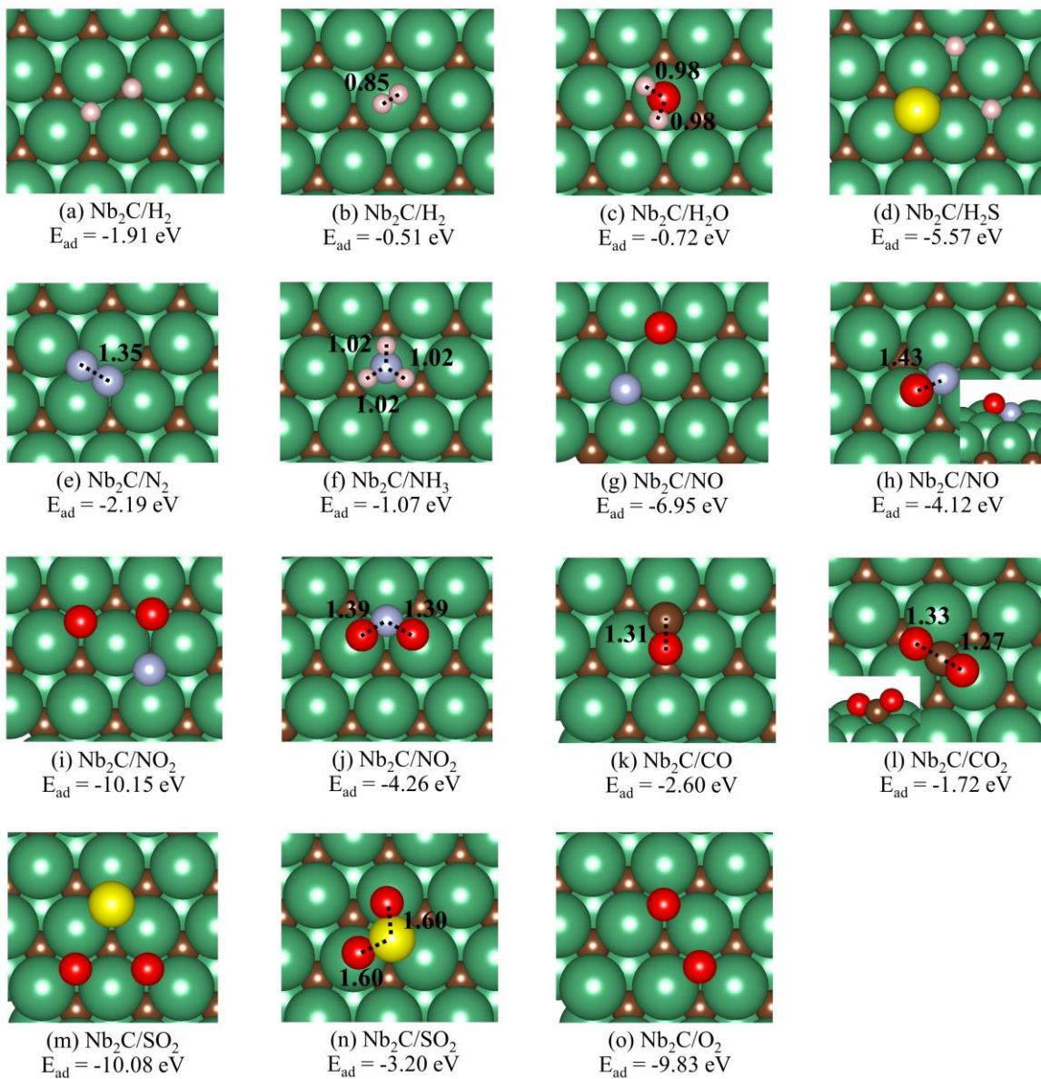
**Fig. S3** The structures of gas adsorption on  $\text{Nb}_2\text{C}$  and  $E_{\text{ad}}$  calculated by PBE
