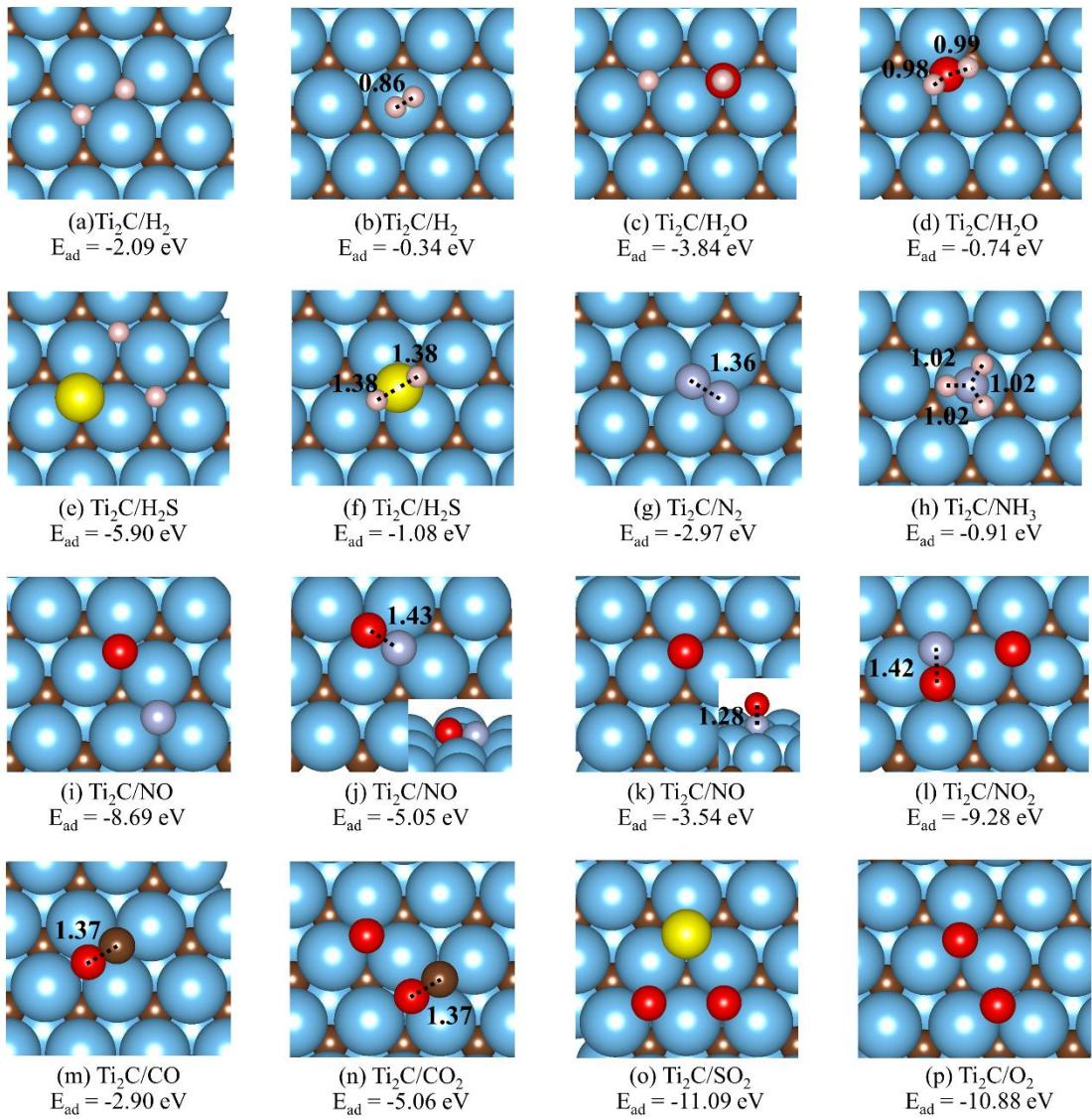
**Fig. S1** The structures of gas adsorption on  $\text{Ti}_2\text{C}$  and  $E_{\text{ad}}$  calculated by PBE
