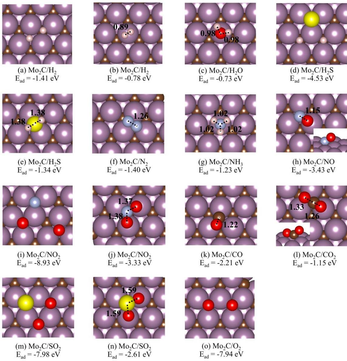
**Fig. S4** The structures of gas adsorption on  $\text{Mo}_2\text{C}$  and  $E_{\text{ad}}$  calculated by PBE
