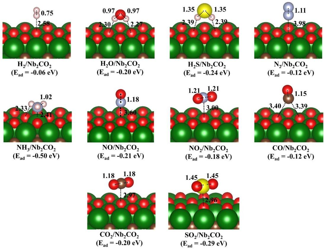
**Fig. S7** The most preferable structures of gas on  $\text{Nb}_2\text{CO}_2$  and  $E_{ad}$  calculated by PBE-D3
