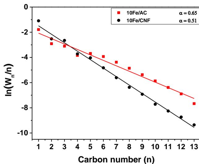
**Fig. S15.** ASF plots of FT products obtained over the AC and CNF supported iron catalysts.
