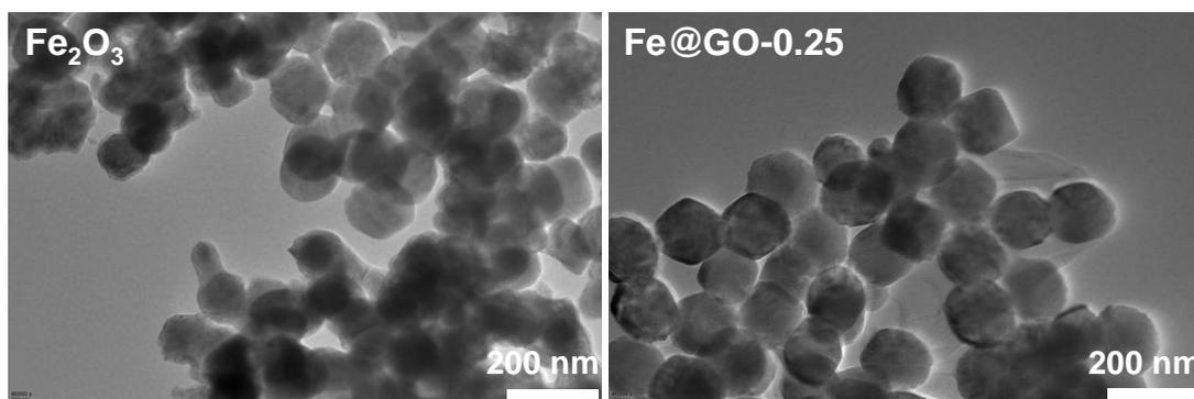
**Fig. S6.** TEM images of the reduced  $\text{Fe}_2\text{O}_3$  and Fe@GO-0.25 catalysts.
