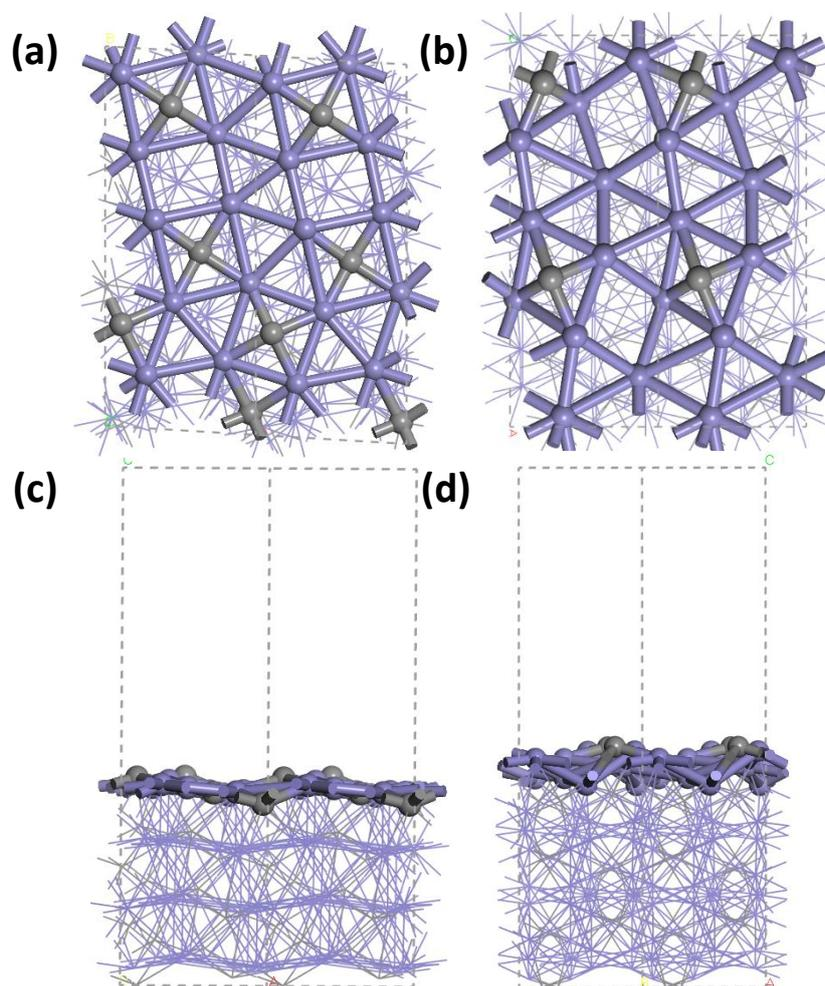
**Fig. S1.** Top views of (a)  $\chi$ - $\text{Fe}_5\text{C}_2$  (510) and (b)  $\chi$ - $\text{Fe}_5\text{C}_2$  (-202) surfaces, and side views of (c)  $\chi$ - $\text{Fe}_5\text{C}_2$  (510) and (d)  $\chi$ - $\text{Fe}_5\text{C}_2$  (-202) surfaces (blue: Fe atoms; grey: C atoms).
