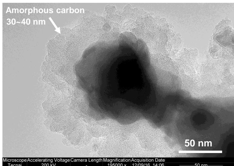
**Fig. S11.** TEM image of spent  $\text{Fe}_2\text{O}_3$  (340 °C) catalyst. Reaction conditions: catalyst = 0.1 g,  $\text{H}_2/\text{CO} = 1.0$ ,  $\text{GHSV} = 22.2 \text{ L}_{\text{gcat}}^{-1}\text{h}^{-1}$ , 1.0 MPa.
