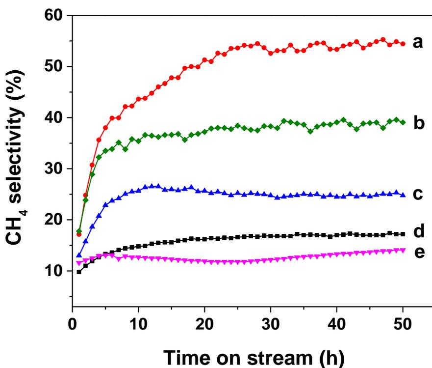
**Fig. S12.** Time on steam evolution of methane selectivity over unmodified and modified  $\text{Fe}_2\text{O}_3$  catalysts. (a)  $\text{Fe}_2\text{O}_3$  NPs (340 °C), (b)  $\text{Fe}@$ PAA-0.25 (340 °C), (c)  $\text{Fe}@$ PVP-0.25 (340 °C), (d)  $\text{Fe}_2\text{O}_3$  NPs (300 °C) and (e)  $\text{Fe}@$ GO-0.25 (340 °C). Reaction conditions: catalyst = 0.1 g,  $\text{H}_2/\text{CO} = 1.0$ ,  $\text{GHSV} = 22.2 \text{ L}_{\text{gcat}}^{-1}\text{h}^{-1}$ , 1.0 MPa.
