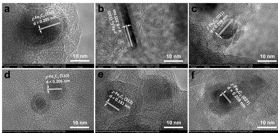
**Fig. S14.** HRTEM images of spent (a-c) 10Fe/AC and (d-f) 10Fe/CNF catalysts.
