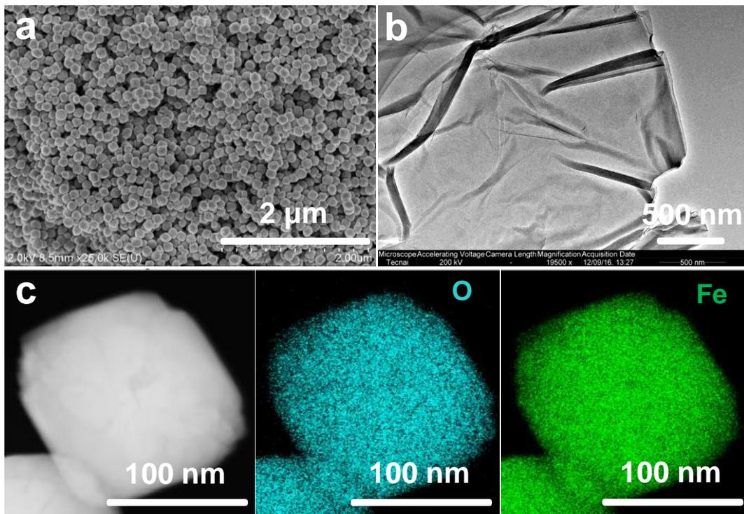
**Fig. S4.** (a) SEM image of  $\text{Fe}_2\text{O}_3$  NPs, (b) TEM image of GO, and (c) original STEM image of  $\text{Fe}_2\text{O}_3$  NPs and corresponding STEM-EDX elemental mapping of Fe and O on the  $\text{Fe}_2\text{O}_3$  NPs.
