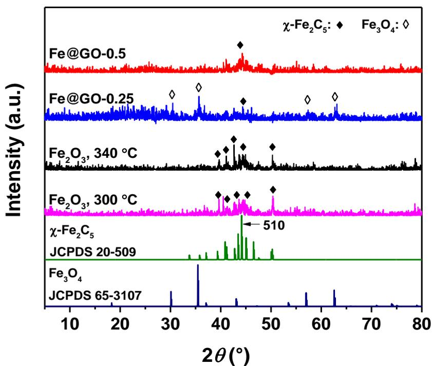
**Fig. S8.** XRD patterns of spent Fe<sub>2</sub>O<sub>3</sub> and Fe@GO catalysts.
