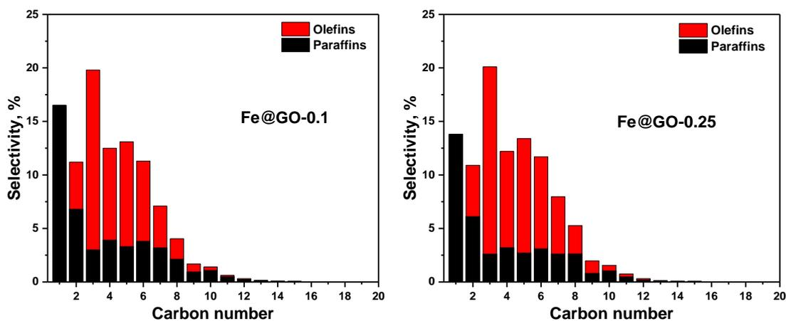
**Fig. S2.** The product distribution obtained over GO modified  $\text{Fe}_2\text{O}_3$  catalysts after 50 h reaction. The selectivities to higher olefins (total olefins) for Fe@GO-0.1 and Fe@GO-0.25 catalysts are 24.5% (54.4%), and 29.5% (60.7%), respectively. Reaction conditions: catalyst = 0.1 g,  $\text{H}_2/\text{CO} = 1.0$ ,  $\text{GHSV} = 22.2 \text{ L g}_{\text{cat}}^{-1}\text{h}^{-1}$ ,  $340 \text{ }^\circ\text{C}$ , 1.0 MPa, 50 h.
