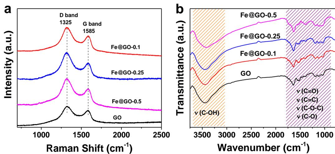
**Fig. S5.** (a) Raman spectra of GO and GO modified  $\text{Fe}_2\text{O}_3$  catalysts; (b) FTIR spectra of GO and GO modified  $\text{Fe}_2\text{O}_3$  catalysts.
