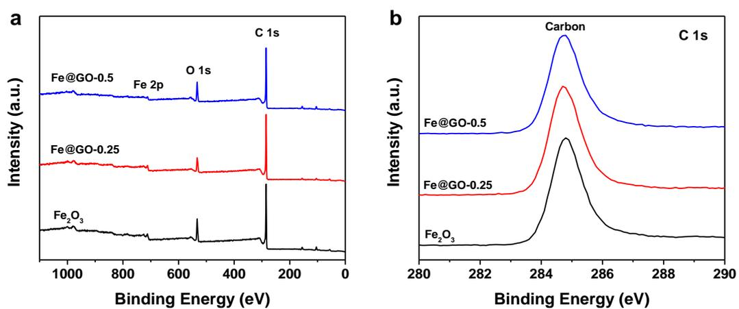
**Fig. S10.** The XPS spectra of spent  $\text{Fe}_2\text{O}_3$  and Fe@GO catalysts: a) survey spectra, b) C 1s spectra.
