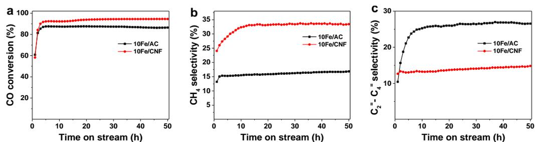
**Fig. S13.** Catalytic performance of different carbon material supported and sulfur promoted catalysts. (a-c) Time on stream evolution of CO conversion, methane selectivity and lower olefins selectivity over AC and CNF supported iron catalysts.
