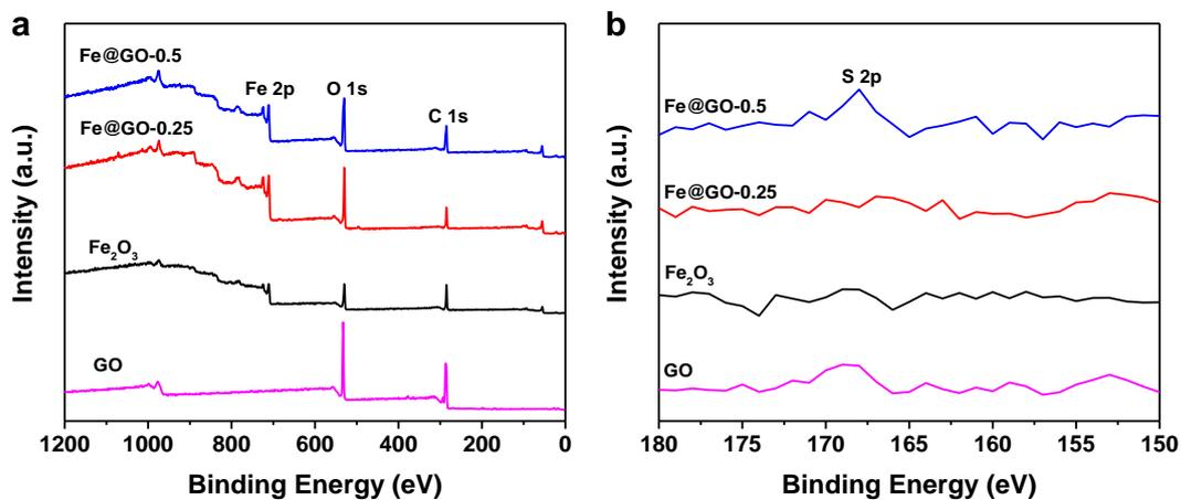
**Fig. S3.** The XPS spectra of fresh GO and Fe@GO catalysts: a) the full spectra, b) the S 2p spectra.
