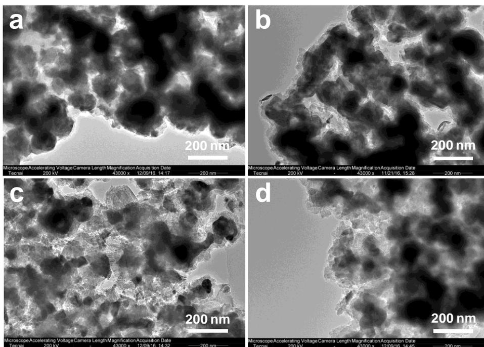
**Fig. S7.** TEM images of catalyst after reaction for 50 h. (a) Fe<sub>2</sub>O<sub>3</sub> NPs (300 °C), (b) Fe<sub>2</sub>O<sub>3</sub> NPs (340 °C), (c) Fe@PAA-0.25 (340 °C), (d) Fe@PVP-0.25 (340 °C). Reaction conditions: catalyst = 0.1 g, H<sub>2</sub>/CO = 1.0, GHSV = 22.2 L g<sub>cat</sub><sup>-1</sup>h<sup>-1</sup>, 1.0 MPa.
