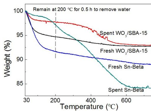
Figure S11 TG curves of the fresh and spent catalysts
