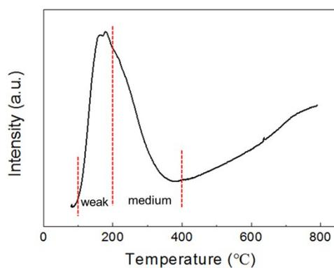
Figure S6 NH<sub>3</sub>-TPD profiles of 0.20-WO<sub>3</sub>/SBA-15-700.
