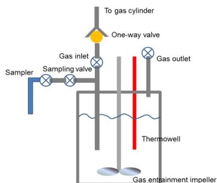
Figure S1 The reactor and sampling system
