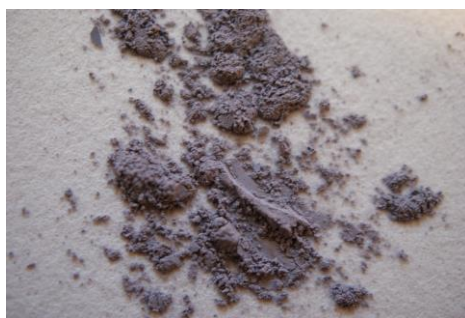
Figure S8. Photo of AuNP/KNbO 3 catalyst synthesized using NaBH 4 as a chemical reducing agent.
