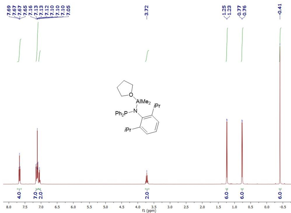
**Figure S2.**  $^1\text{H}$  NMR spectrum of  $\text{Ph}_2\text{P}(\text{DIPP})\text{NaIMe}_2 \cdot \text{THF}$  in  $\text{C}_6\text{D}_6$ .
