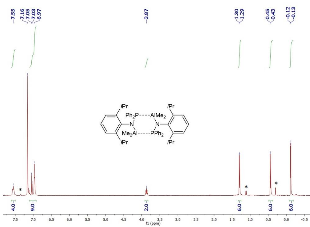
**Figure S1.**  $^1\text{H}$  NMR spectrum of  $[\text{Ph}_2\text{P}(\text{DIPP})\text{NaIMe}_2]_2$  in  $\text{C}_6\text{D}_6$ . The complex is very poorly soluble in aromatic solvents. Impurities marked by \* are due to DIPP-NH<sub>2</sub> and silicon grease.
