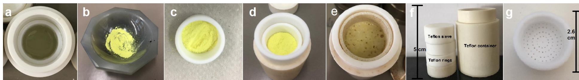
Figure S3 Pictures of sample preparation (a-e) and used Teflon objects for DGC (f and g).
