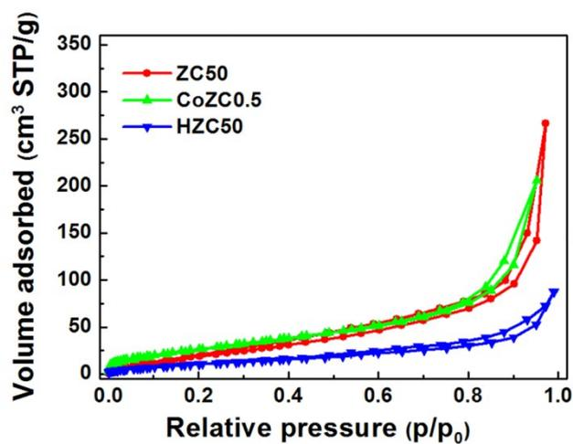
**Fig. S5.** Nitrogen adsorption/desorption isotherms of the  $Zn_{0.5}Cd_{0.5}S$  samples (HZC50: prepared with hydrothermal; ZC50 and CoZC50 represent the sample derived from ZIF-8 and CoZn-ZIF (Co=0.5 at%), respectively). Thanks to the highly porous precursors, ZC50 and CoZC-0.5 exhibits much larger  $N_2$  adsorption volume and  $S_{BET}$  (87.4 and 68.9  $m^2/g$  respectively) than that of HZC50 (17.3  $m^2/g$ ).
