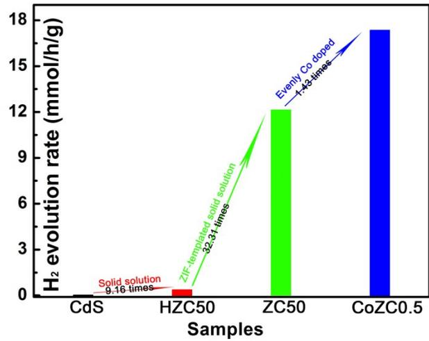
**Figure S9.** The comparison results of the photocatalytic hydrogen production rate of CdS, Zn<sub>0.5</sub>Cd<sub>0.5</sub>S derived from hydrothermal method (HZC50), ZIF-8 (ZC50) and ZnCo-ZIF (CoZC0.5).
