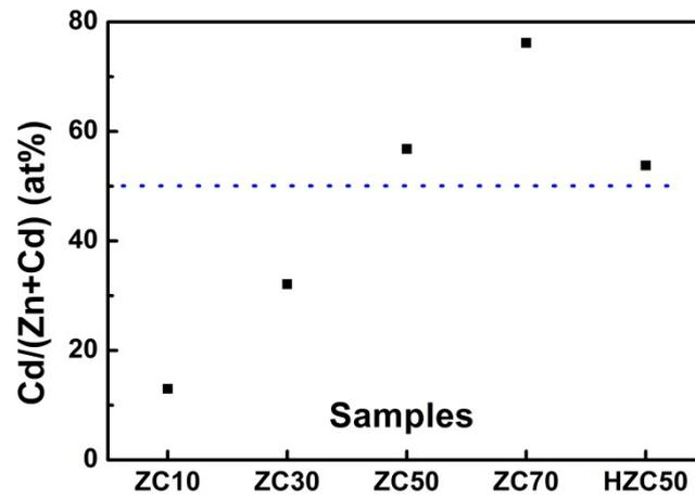
**Fig. S4.** Inductively coupled plasma (ICP) results for the samples prepared with different Cd content. There was no dramatically variation between the setting and tested Cd and Co concentration.
