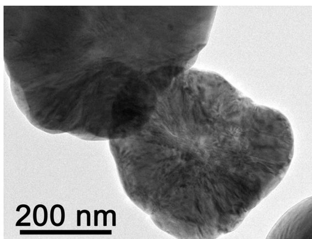
**Fig. S8.** Transmission electron microscope image of CoZC0.5 after the photocatalytic reaction over 30 h.
