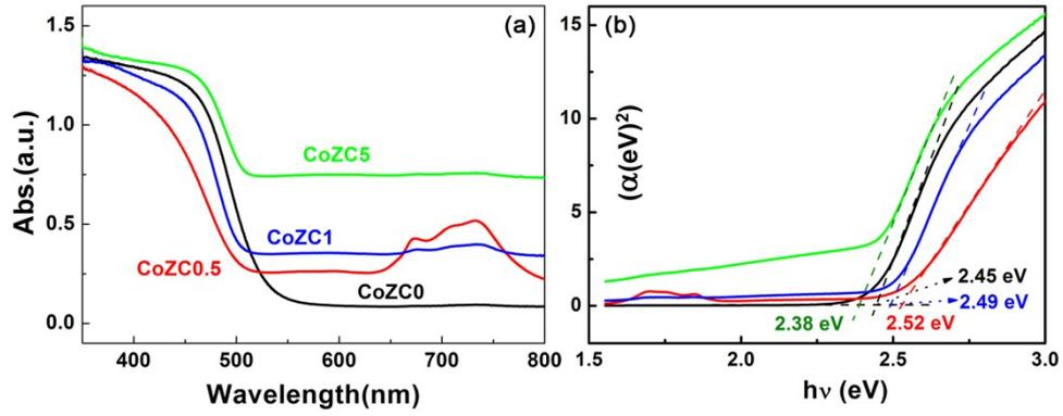
**Fig. S3.** The (a) UV–visible diffuse reflection spectra and (b) the band gaps of the  $\text{Zn}_{1-x}\text{Cd}_x\text{S}$  solid solutions with different Co concentration.
