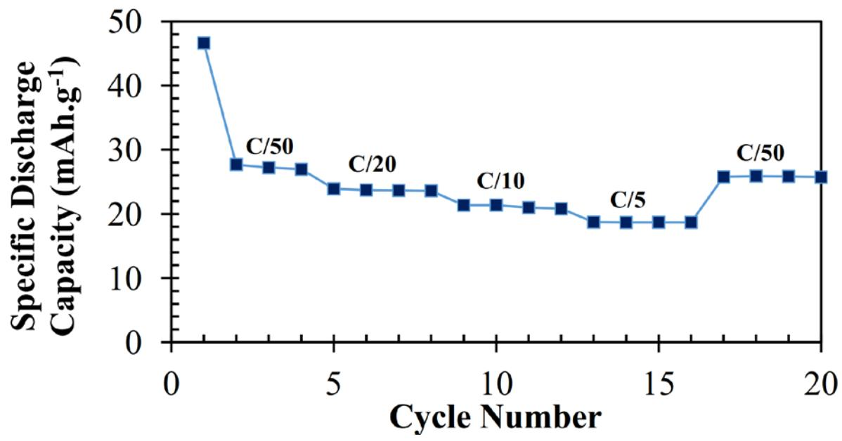
Figure S1: Test of cycle life showing capacity retention at various C-rates for  $\text{Li}_5\text{Fe}_2(\text{PO}_4)\text{F}_8$  cathode.
