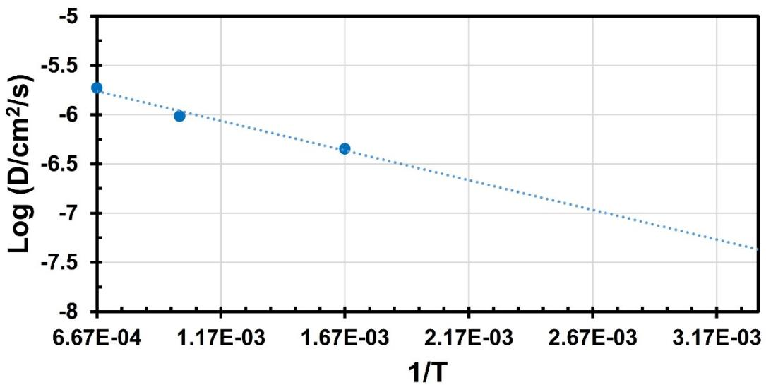
Figure S4. Arrhenius plot of Li<sup>+</sup> diffusivity vs. temperature as obtained from ab initio molecular dynamic (AIMD) simulations.
