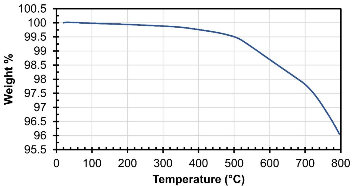
Figure S3. TGA curve of  $\text{Li}_5\text{Fe}_2\text{PO}_4\text{F}_8$  under  $\text{N}_2$  flow at  $10 \text{ }^{\circ}\text{C}.\text{min}^{-1}$  heating rate.
