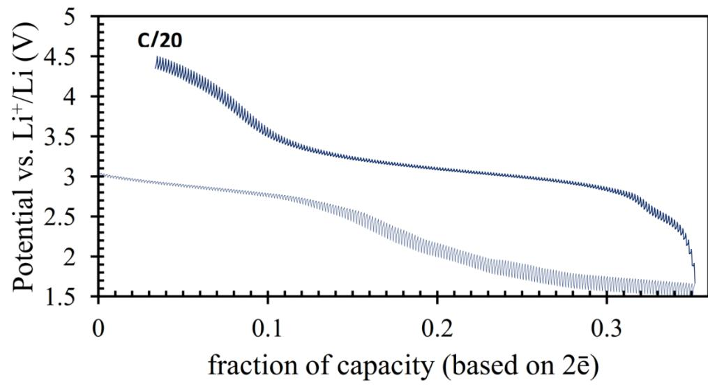
Figure S2. Charge-discharge GITT curves for  $\text{Li}_5\text{Fe}_2(\text{PO}_4)\text{F}_8$
