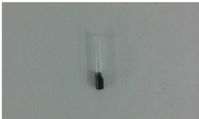
Figure S8. Quartz capillary loaded with the viscous complex 2 for EPR studies.
