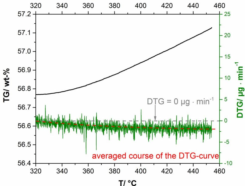
**Figure S 7.** Excerpt of the thermal analysis in the range between 320 °C and 450 °C, the oxidation of Cu<sub>2</sub>O is indicated by the increase of the mass of the residue (TG curve, black line) and by the negative DTG values (green line, red trend line).
