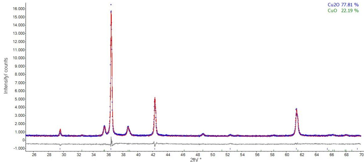
**Figure S 6.** Quantitative phase analysis of the residue of the thermal decomposition of the 1-2-0 phase after heating the sample up to 450 °C.
