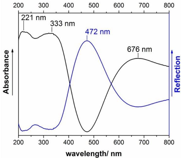
**Figure S 5.** UV/VIS reflectance spectrum of the 1-2-0 phase.
