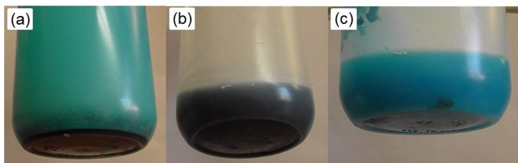
**Figure S 3.** Photographs of the polypropylene vessels in which freshly precipitated Cu(OH)<sub>2</sub> was reacted with copper(II)-acetate solutions for 40 d, (a) reaction with 0.05 m Cu(CH<sub>3</sub>COO)<sub>2(aq)</sub>, (b) reaction with 0.15 m Cu(CH<sub>3</sub>COO)<sub>2(aq)</sub>, (c) reaction with 0.35 m Cu(CH<sub>3</sub>COO)<sub>2(aq)</sub>, the black color indicates the presence of CuO.
