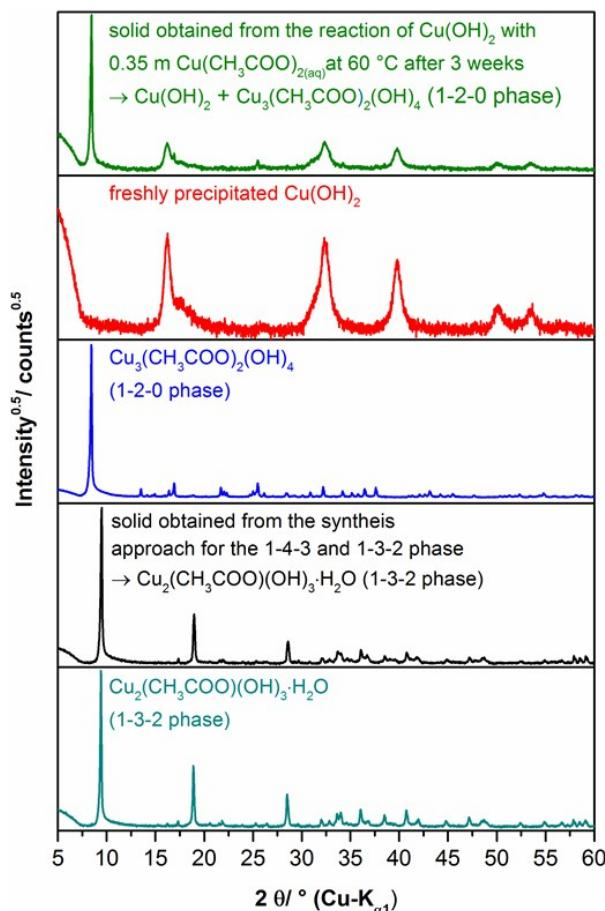
**Figure S 2.** XRPD patterns of various solid products and intermediates of the synthesis approaches for basic copper acetates.
