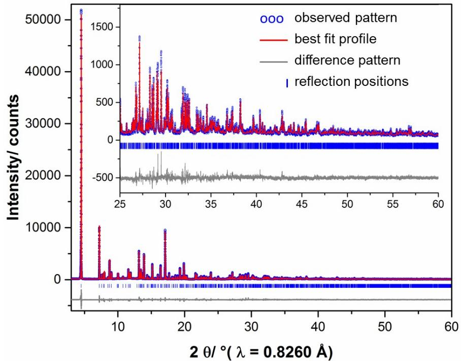
**Figure S 1.** Scattered X-ray intensities of the 1-2-0 phase at 303 K as a function of diffraction angle  $2\theta$ . The observed pattern (circles) measured in Debye-Scherrer geometry, the best Rietveld fit profiles (line) and the difference curve between the observed and the calculated profiles (below) are shown. The high angle part starting at  $25.0^\circ$  in  $2\theta$  is enlarged for clarity.
