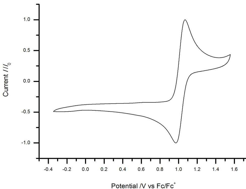
*1,1'-Di(butylmethylsulfonium)ferrocene di{bis(trifluoromethanesulfonyl)imide}* ( $10 \text{ mV s}^{-1}$  in [EMIM]TFSI)
