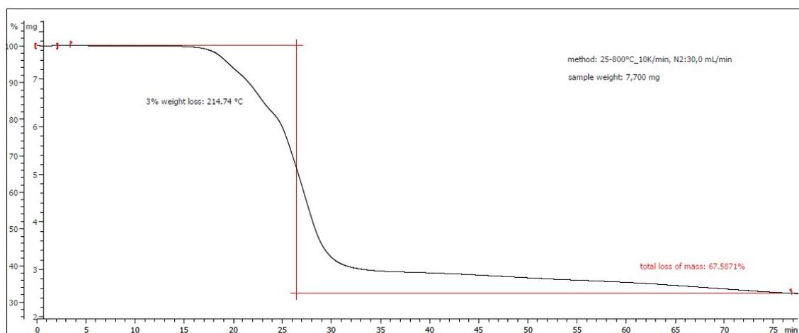
***Diferrocenylmethylsulfonium tetrafluoroborate*** (sDTA above, TGA below, each 10 K min<sup>-1</sup>)
