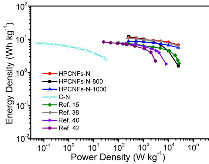
**Fig. S15** Ragone plots of HPCNFs-N, the control samples and other carbon-based devices.
