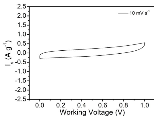
**Fig. S14** CV curve of N-CNFs at the scan rate of 10.0 mV s<sup>-1</sup>.
