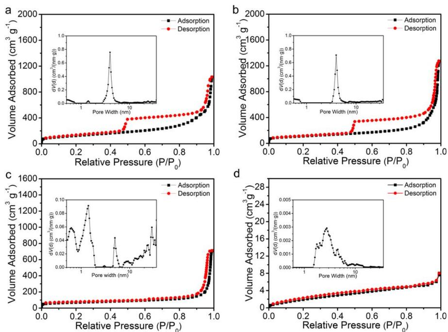
**Fig. S10** N<sub>2</sub> adsorption/desorption isotherms and the corresponding pore-size-distribution curves of the control samples. (a) HPCNFs-N-800, (b) HPCNFs-N-1000, (c) C-N and (d) N-CNFs.
