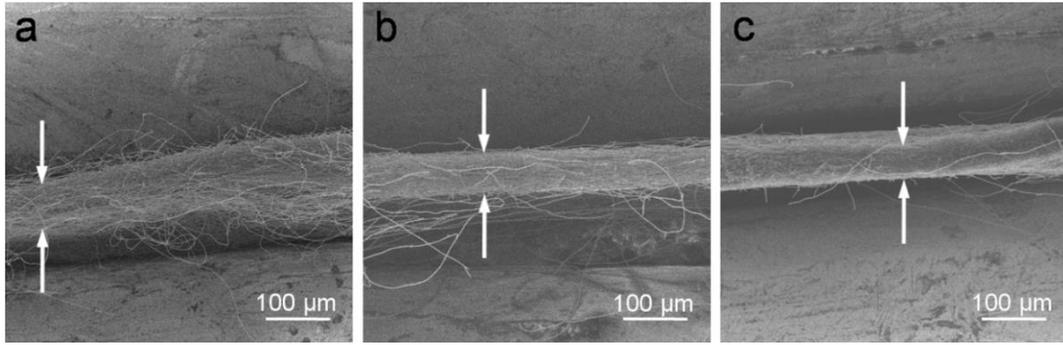
**Fig. S5** FESEM characterizations. The cross-section FESEM images of (a) HPCNFs-N-800, (b) HPCNFs-N and (c) HPCNFs-N-1000.
