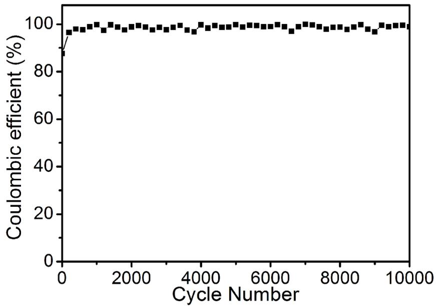
**Fig. S16** The Coulombic efficiency of HPCNFs-N during the cycling test at a current density of 5.0 A g<sup>-1</sup>.
