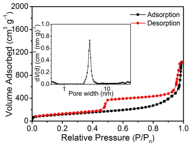
**Fig. S9** N<sub>2</sub> adsorption/desorption isotherms and the corresponding pore-size-distribution curve of HPCNFs-N.
