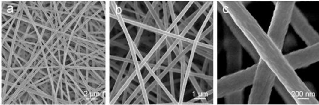
**Fig. S1** FESEM characterizations of the PAN nanofibers without the addition of ZIF-8 particles.
