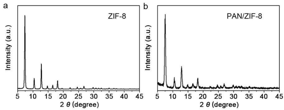
**Fig. S2** XRD patterns of the ZIF-8 particles and PAN/ZIF-8 nanofibers.
