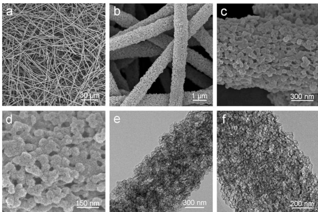
**Fig. S17** FESEM and TEM characterizations of the HPCNFs-N electrode after 10000 discharge/charge cycles at  $5.0 \text{ A g}^{-1}$ .
