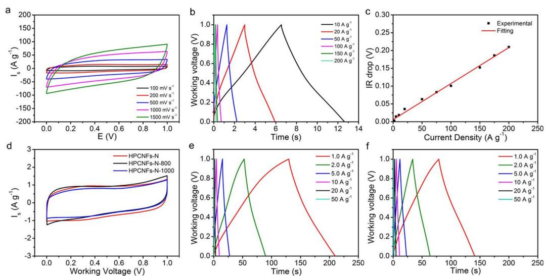
**Fig. S12** (a) CV curves at different scan rates, (b) galvanostatic charge-discharge curves at different current densities and (c)  $IR$  drop at different current densities of HPCNFs-N. (d) CV curves of different samples at a current density of  $10.0 \text{ mV s}^{-1}$ . Galvanostatic charge-discharge curves at different current densities of (e) HPCNFs-N-800 and (f) HPCNFs-N-1000.
