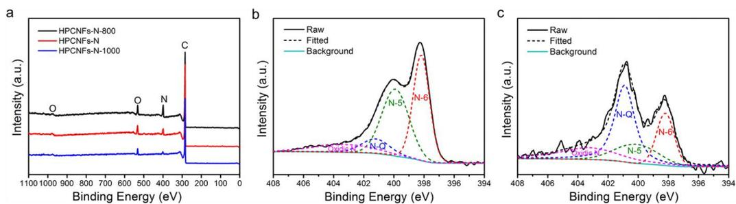
**Fig. S8** (a) XPS survey spectra of HPCNFs-N and the control samples. High resolution spectra of N 1s for (b) HPCNFs-N-800 and (c) HPCNFs-N-1000.
