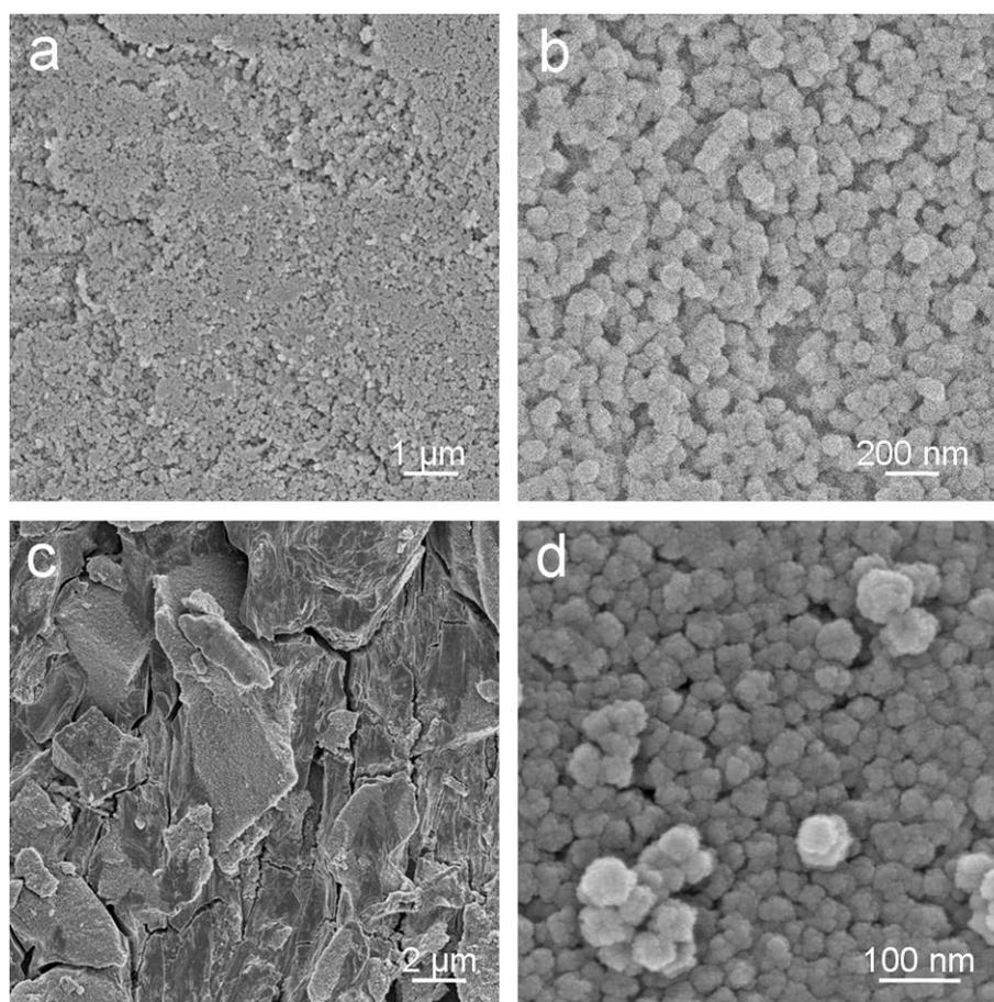
**Fig. S4** FESEM characterizations. FESEM images of (a,b) ZIF-8 nanoparticles and (c,d) the resultant N-doped carbon (C-N) after carbonization process.
