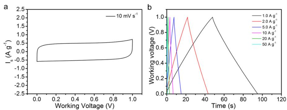
**Fig. S13** Supercapacitive performance of C-N. (a) CV curve at the scan rate of 10.0 mV s<sup>-1</sup>. (b) Galvanostatic charge-discharge curves at different current densities.
