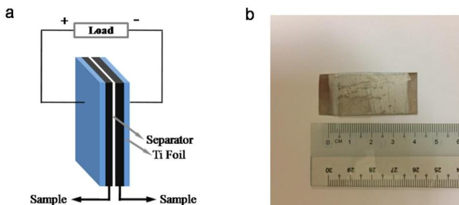
**Fig. S11** Two-electrode system for measuring supercapacitive performance. (a) Schematic diagram of the two-electrode configuration. (b) Photograph of a supercapacitor with as-synthesized samples as the electrodes.
