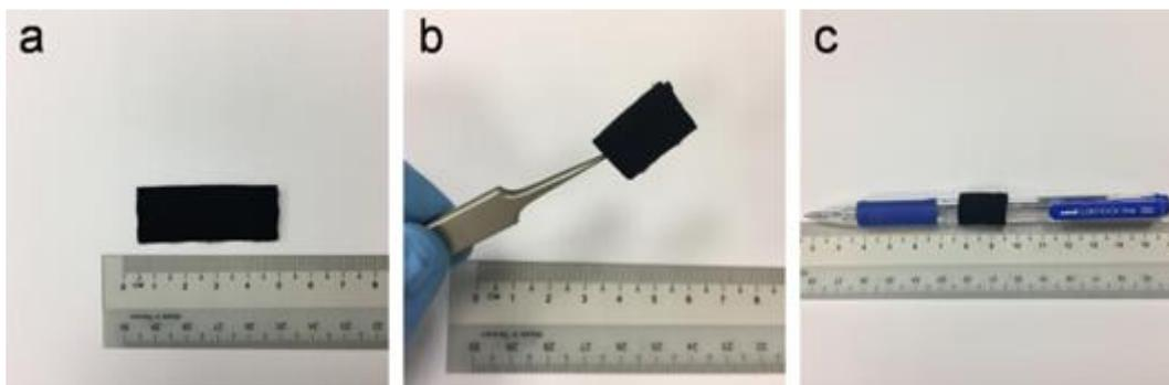
**Fig. S3** Representative photographs showing the flexibility of the HPCNFs-N sample.
