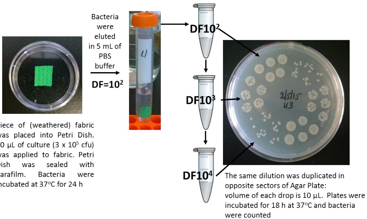
Figure S7: Outline of experimental procedures used to determine efficacy of Ag textile.
