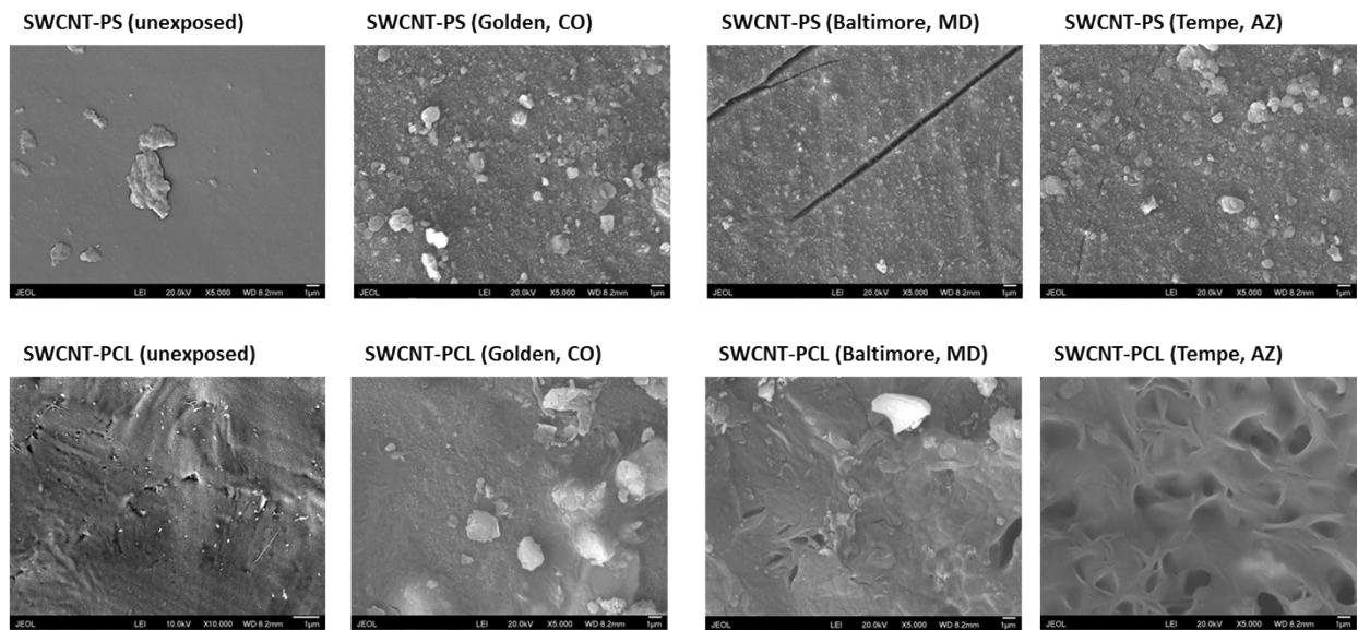
Figure S5: SEM imaging of SWCNT-PNC samples before and after weathering reveals no CNT accumulation at the surface of any PNC type or at any of the location.
