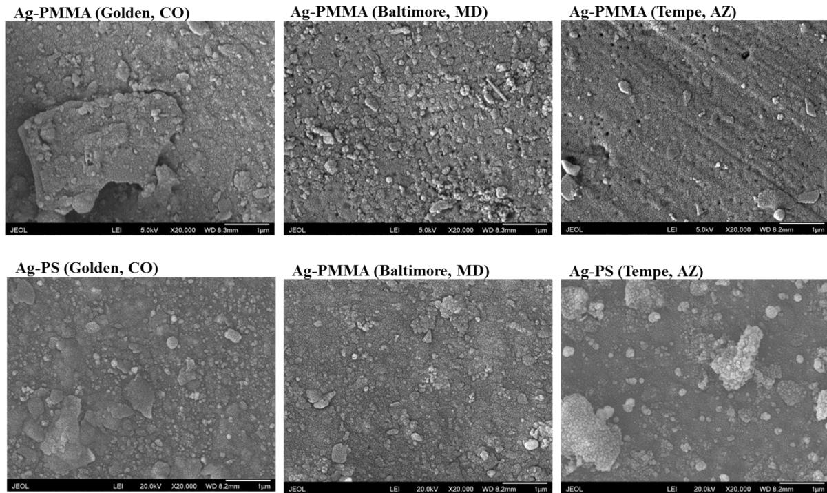
Figure S4: SEM images of Ag-PNC samples following weathering reveals no Ag nanoparticles remain visible at the surface for either PNC type, at all three locations.
