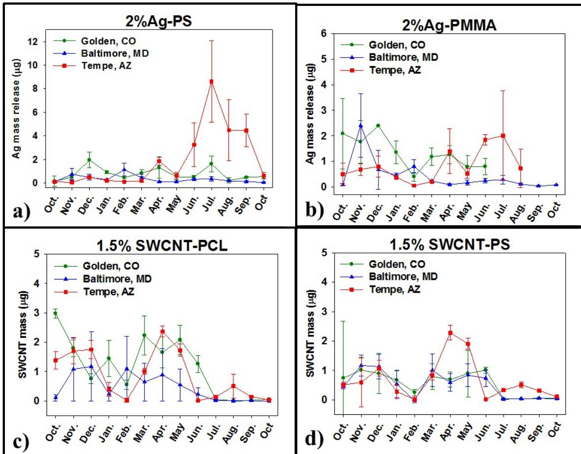
Figure S10: (a,b) Monthly Ag release mass measurements comparing Ag-PNCs located at all three sites. (c,d) Monthly SWCNT mass release measurements from SWCNT-PNCs located at all three sites. Error bars represent standard deviation of release mass measured from triplicate samples at each location. Release data demonstrates SWCNT and Ag release, however as it is shown in monthly increments, overall release trends are difficult to discern.
