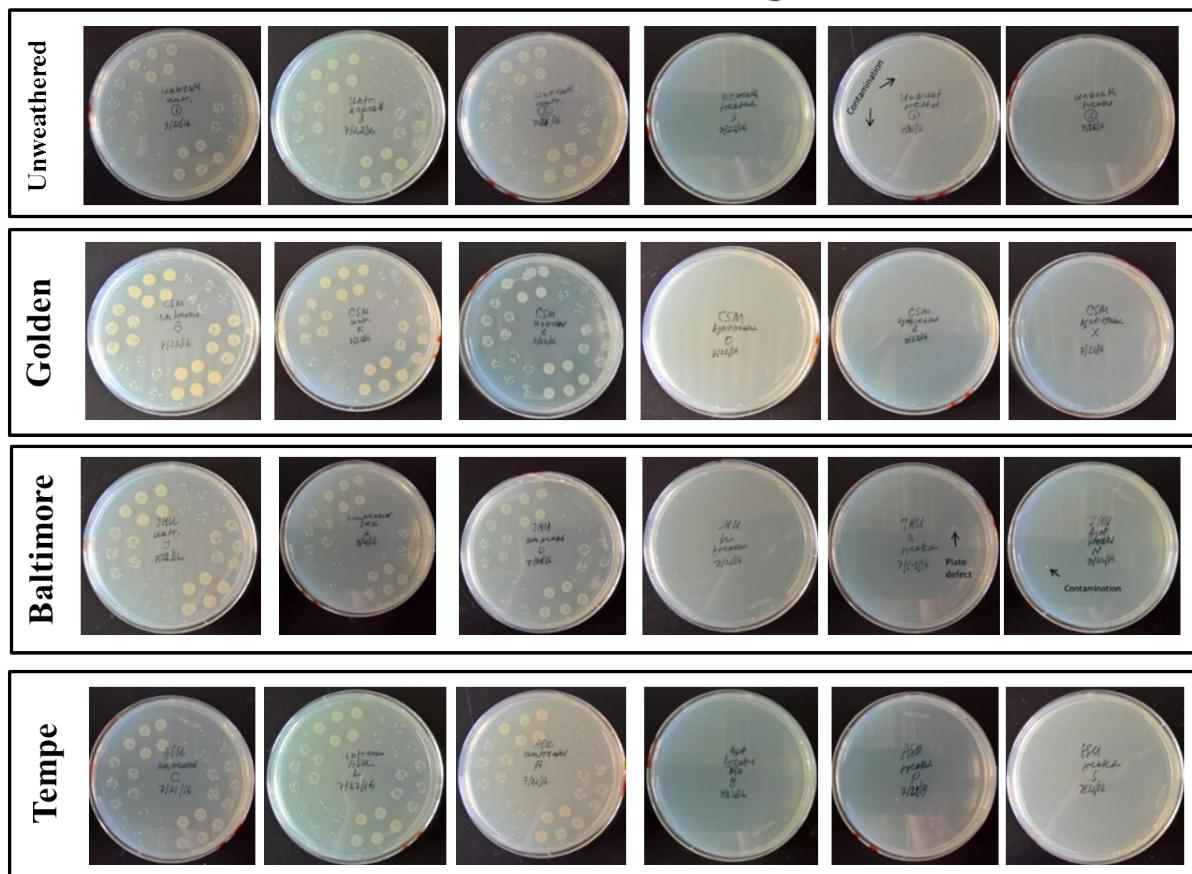
Figure S11: Pictures captured of triplicate antimicrobial efficacy test results, for each location. Images show that anti-microbial efficacy is maintained for all Ag treated textile samples in each location and that weathering has no impact on the antimicrobial efficacy of the untreated textile samples weathered in each location.
