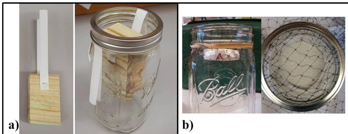
Figure S9: (a) Pressure treated lumber is used, as purchased, with the only alteration being cut down in size to fit within the collection jar and affixed to Teflon straps so it may hang freely and weather passively. (b) TX Active Cement puck provided by Lehigh Heidelberg Cement Group is held in place with thin nylon netting.
