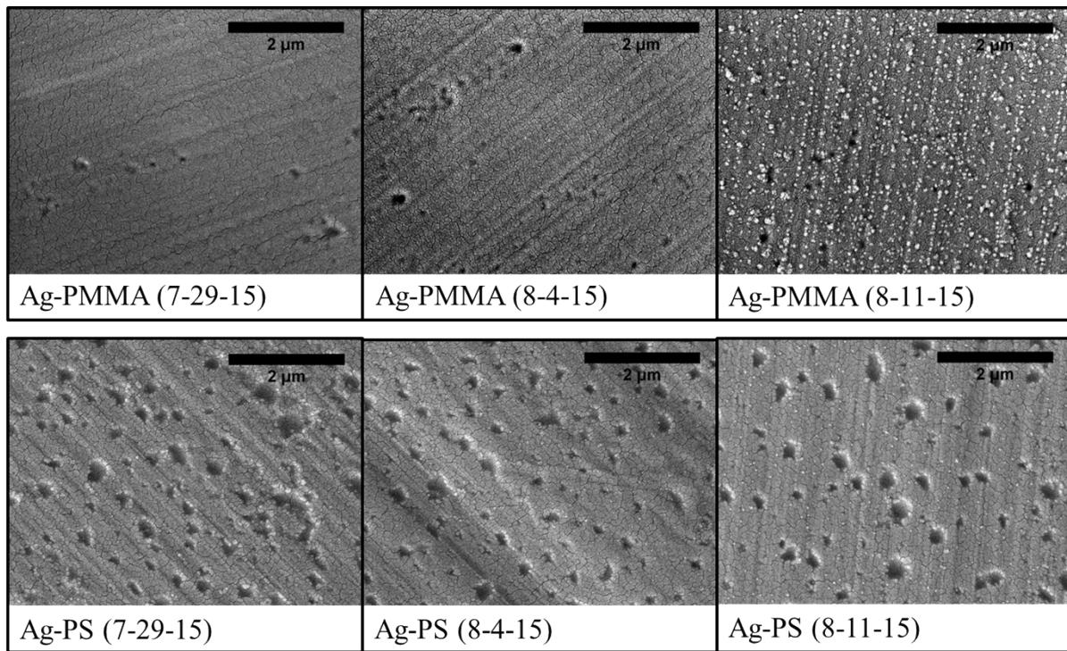
Figure S1: Representative SEM image of silver nanocomposites from each batch used in the study (Polystyrene – PS, Poly (methyl methacrylate) – PMMA). Silver nanoparticles appear as white dots in images collected and are approximately 20nm in diameter, when monodispersed.
