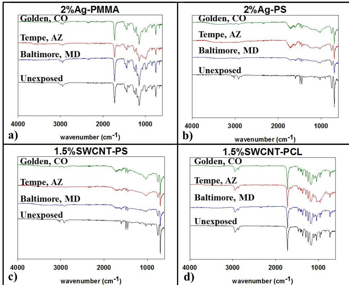
Figure S3: ATR-FTIR spectra of PNCs following weathering finds that the spectra collected of samples weathered at each location are consistent with each other, suggesting that samples weathered at each location experienced similar, shallow, depths of photodegradation.
