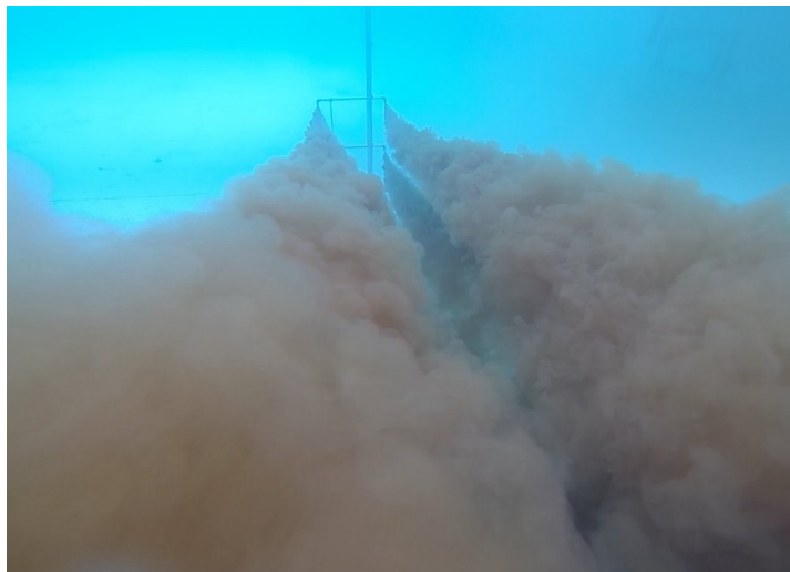
Movie S3. Oil plume frame view – orientation 1. Oil plume (ANS crude) as viewed underwater with the camera situated directly next to the foam pad frame. Movie is shown in real-time.
