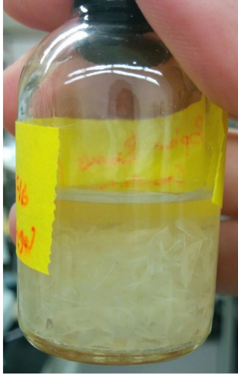
Figure S.1. Typical preparation of anaerobic batch culture bottle of cryotome transverse-sectioned poplar stem in MTC media loaded at 10g biomass/L.
