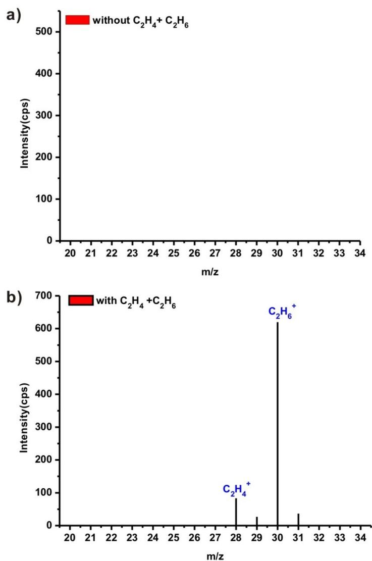
Fig.S1 The mass spectra of the standard mix gas of ethylene and ethane with the same concentration of 10ppm(b) and its blank(a) in our homogeneous system.
