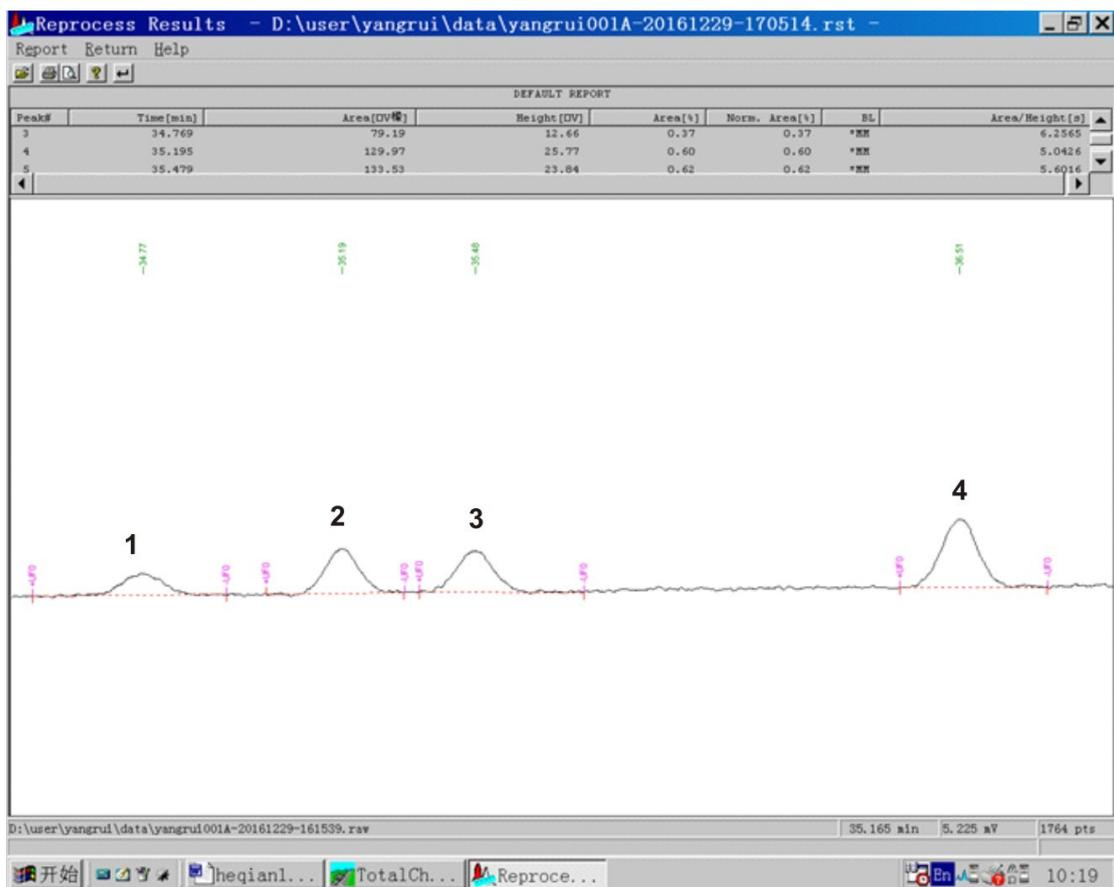
Fig.S4 The GC chromatogram of the standard mix gas of methane, ethylene, ethane and propylene with the same concentration.
