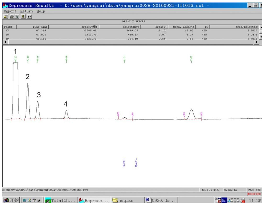
Fig.S7 The GC chromatogram of methane/Se mixture in DBD system.
