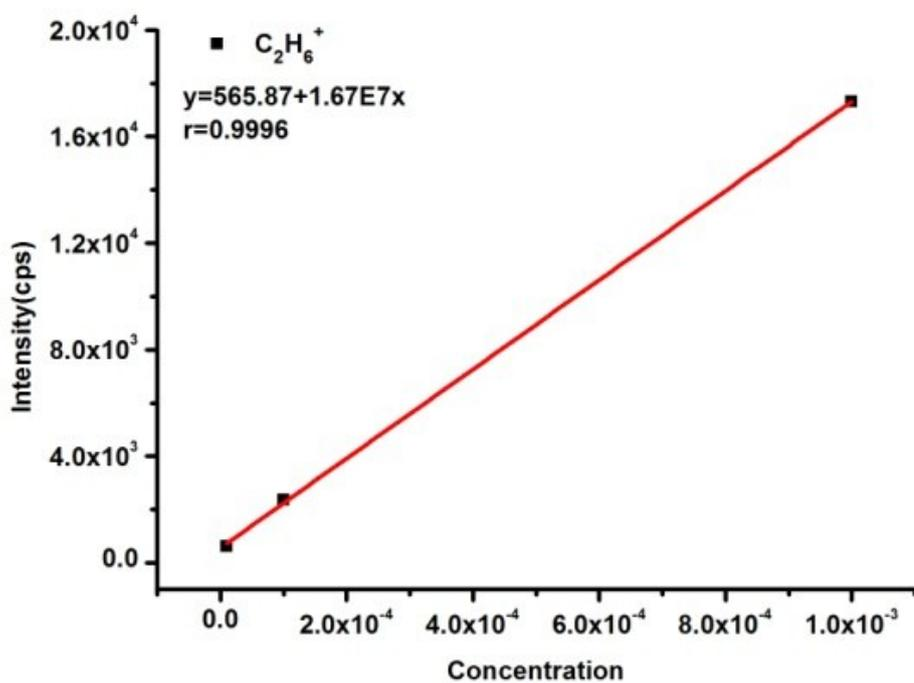
Fig.S3 The relationship between the MS intensities (m/z 30) and the concentrations of C<sub>2</sub>H<sub>6</sub> in ICP-QQQ-MS system.
