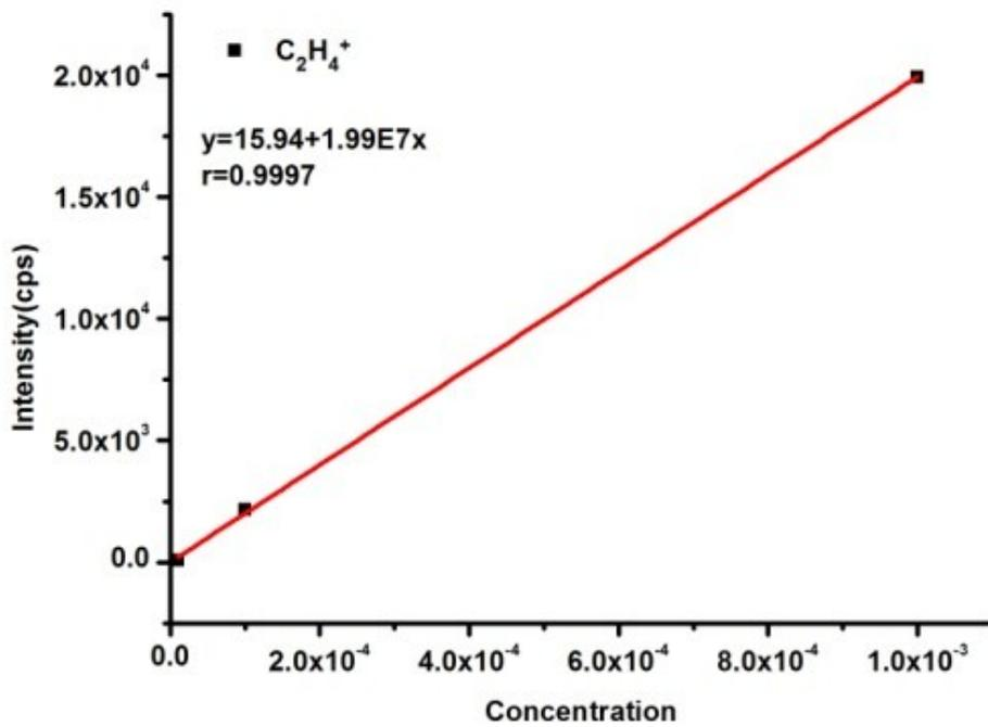
Fig.S2 The relationship between the MS intensities (m/z 28) and the concentrations of C<sub>2</sub>H<sub>4</sub> in ICP-QQQ-MS system.
