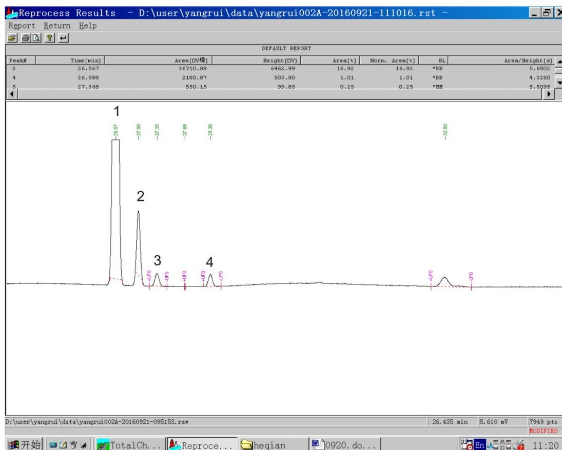
Fig.S6 The GC chromatogram of methane in DBD system.
