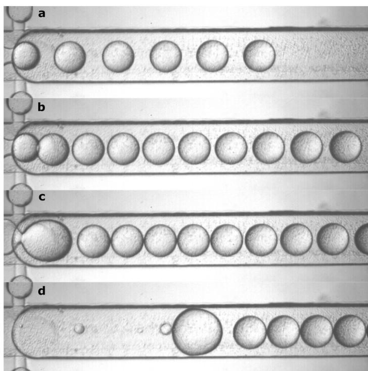
Fig. S2 Formation of the emulsion at 1.0 % (w/w) fluorosurfactant at flow rate of 6 ml/h. a) Droplets generated from the front of the mother droplet do not interfere with each other. b) Droplets generated from the rear end of the mother droplet interfere with each other. c) At a critical point, the neck does not break. d) One large droplet and multiple small droplets are generated in the final stage of the emulsification process.
