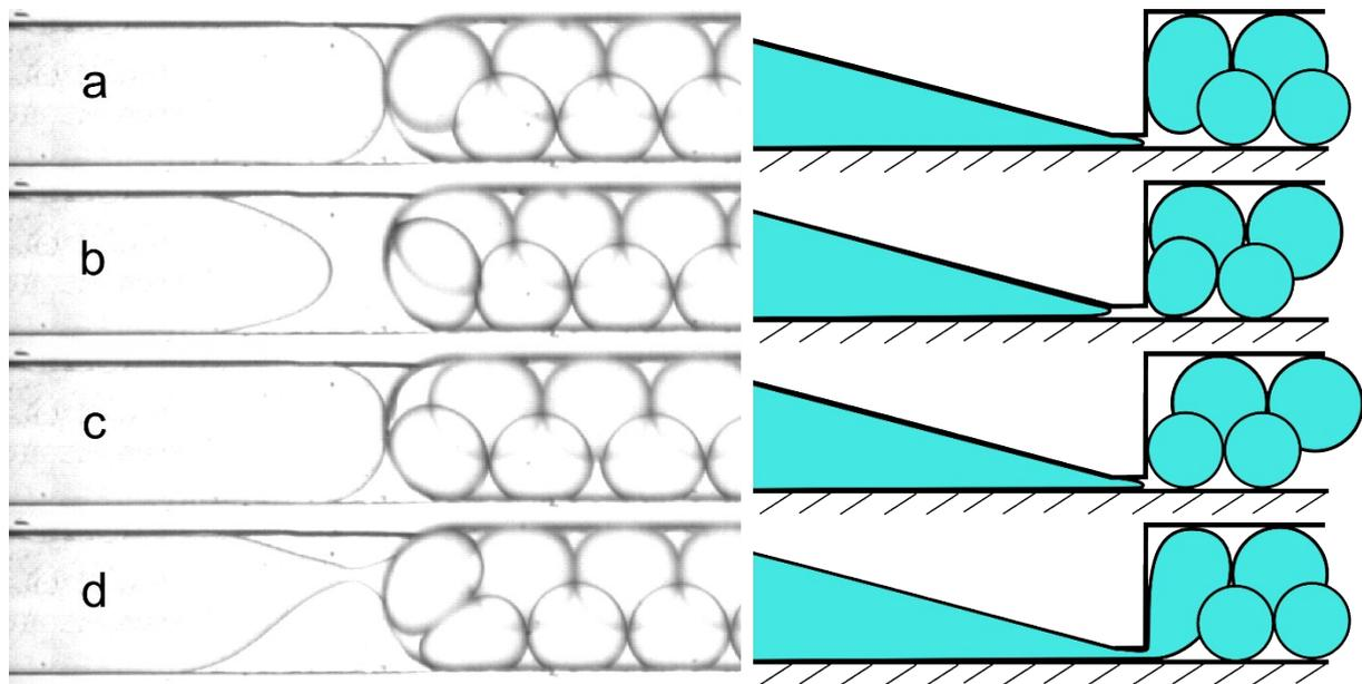
Fig. S3 a) A large droplet is situated above the step. b) A new droplet fills the available space close to the step, becoming a small droplet. c) A small droplet leaves more space for the new droplet. d) A new droplet fills the available space above the step, and becomes a large droplet. Cartoons on the right portrait the side view of the process at the step.
