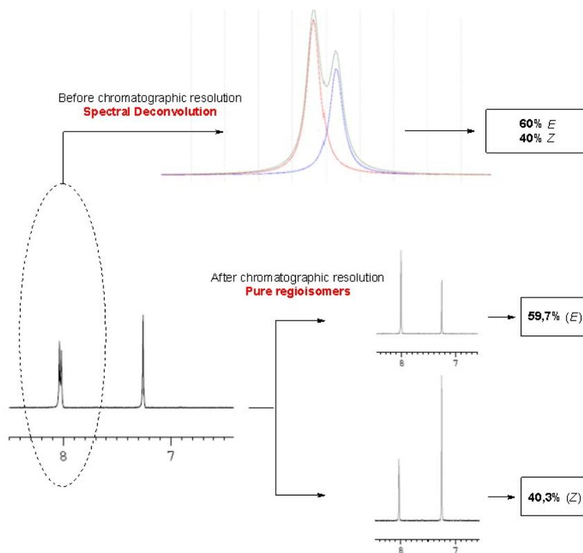
**Figure S2** Chromatographic resolution of products.  $^1\text{H}$  NMR signal of triazolic proton. The deconvolution spectra allow us to calculate the ratio between regioisomers.
