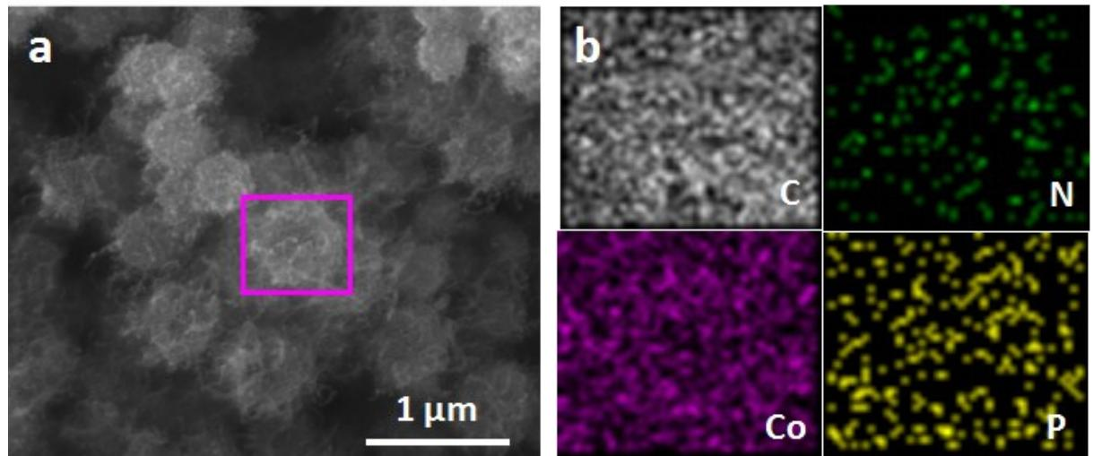
**Fig. S4** The EDS mapping of Co/CoP-HNC.
