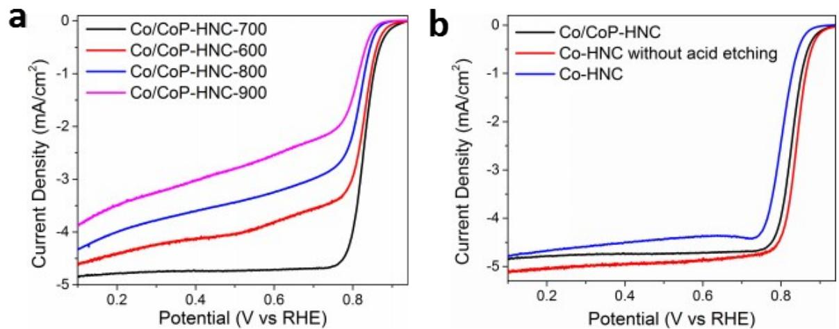
**Fig. S5** The ORR evaluation for (a) Co/CoP-HNC with different pyrolysis temperature and (b) Co/CoP-HNC, Co-HNC pre, Co-HNC.
