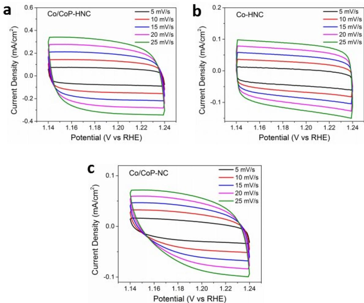
**Fig. S6** The CV plots of (a) Co/CoP-HNC, (b) Co-HNC and (c) Co/CoP-NC with different scan rates.
