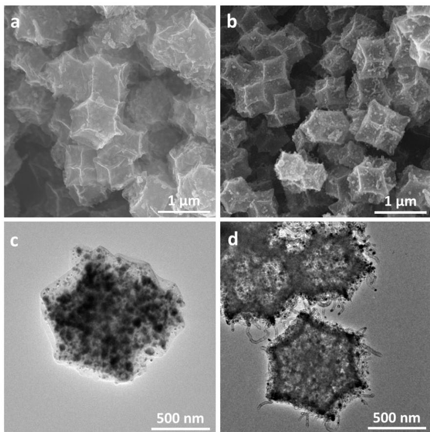
**Fig. S3** The SEM images and their corresponding TEM images of Co/CoP-NC (a, c), Co-HNC (b, d).
