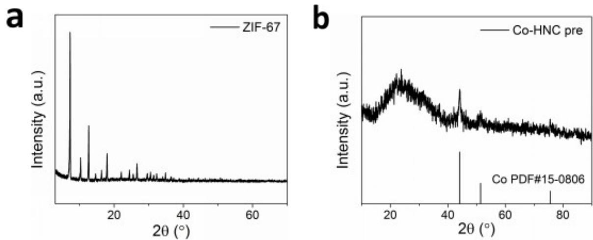
**Fig. S2** The XRD spectra of (a) ZIF-67 and (b) Co-HNC pre.
