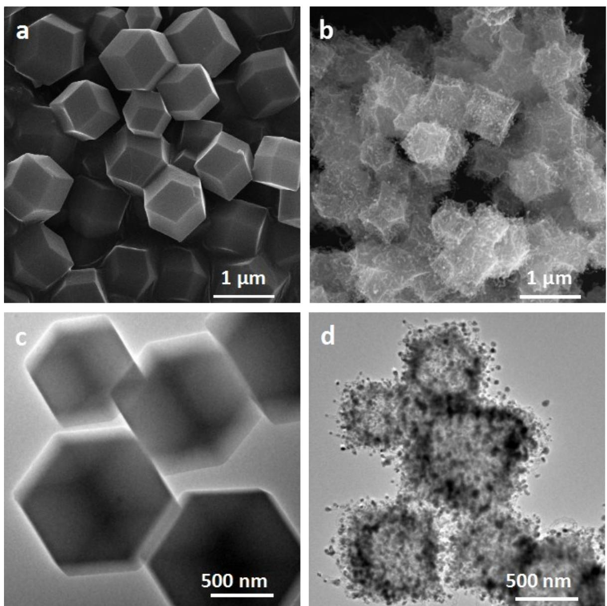
**Fig. S1** The SEM images and corresponding TEM images of ZIF-67 (a, c) and Co-HNC pre (b, d).
