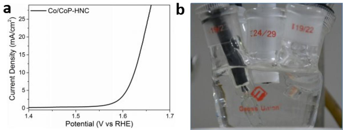
**Fig. S7** (a) The OER performance of Co/CoP-HNC on GC in 0.1 M KOH. (b) A bubble was observed on GC after 400 s under a constant potential of 1.56 V.
