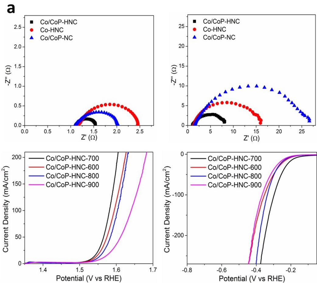
**Fig. S8** The EIS spectra of Co/CoP-HNC, Co-HNC and Co/CoP-NC for (a) OER and (b) HER. The performance of Co/CoP-HNC with different pyrolysis temperature for (c) OER and (d) HER.
