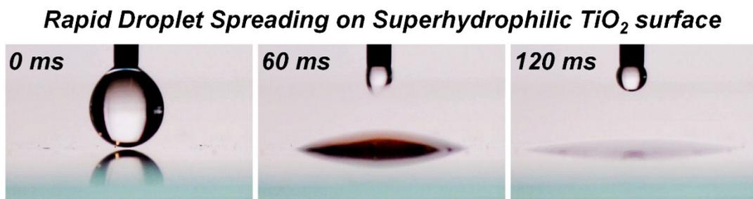
Fig. S2. The rapid droplet spreading on the superhydrophilic  $\text{TiO}_2$  based surface.
