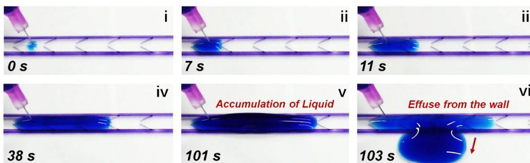
Fig. S3. The unidirectional liquid spreading on a patterned glass slide without superhydrophilic titania coating. The directionality is effective in one or more joint; however, the long-ranged delivery is not available due to the overlarge motion resistance. The massively accumulated liquid should effuse from the channel walls, resulting in the failure of delivery.
