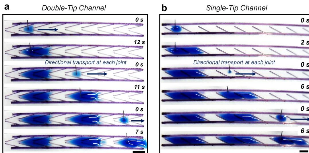
Fig. S4. The discontinuous water charging process clearly demonstrates the consistency of the directionality of water spreading in each joint of channel.
