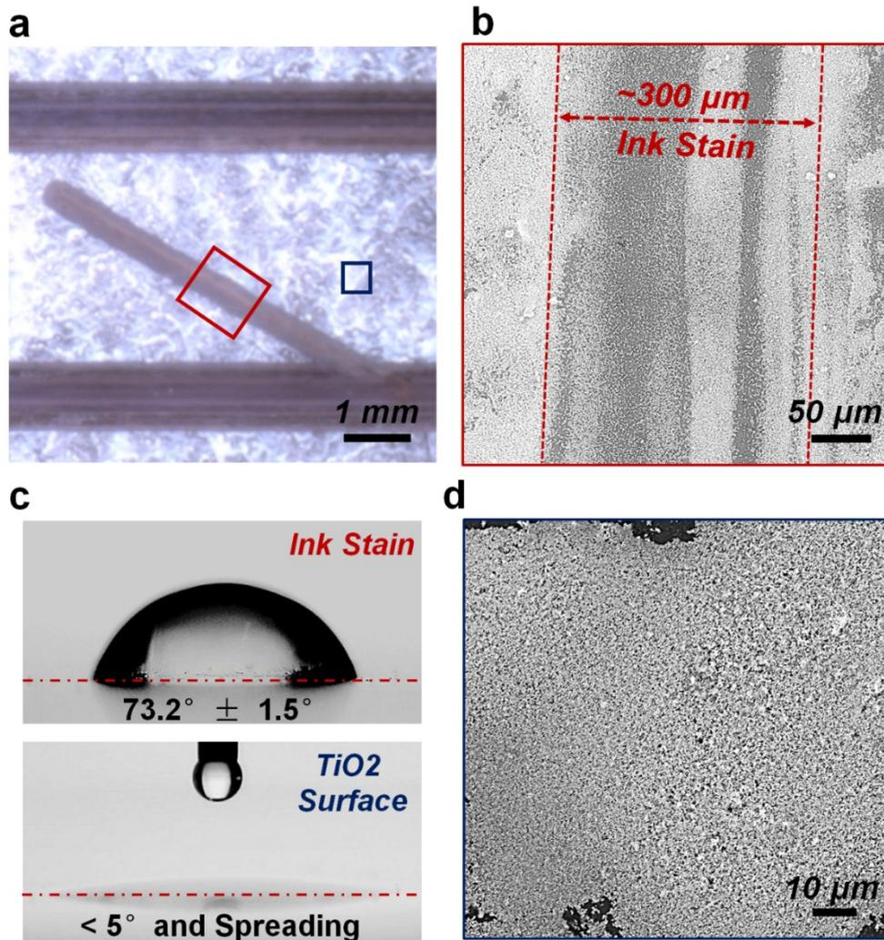
Fig. S1. (a) Optical image of unidirectional liquid spreading surface with 2D wettability patterns. The SEM image of (b) the hydrophobic marker pen stain and (d) the  $\text{TiO}_2$  micro-particles coated surface with superhydrophilic property. (c) The contact angles of the hydrophobic ink stain and the superhydrophilic  $\text{TiO}_2$  surface.
