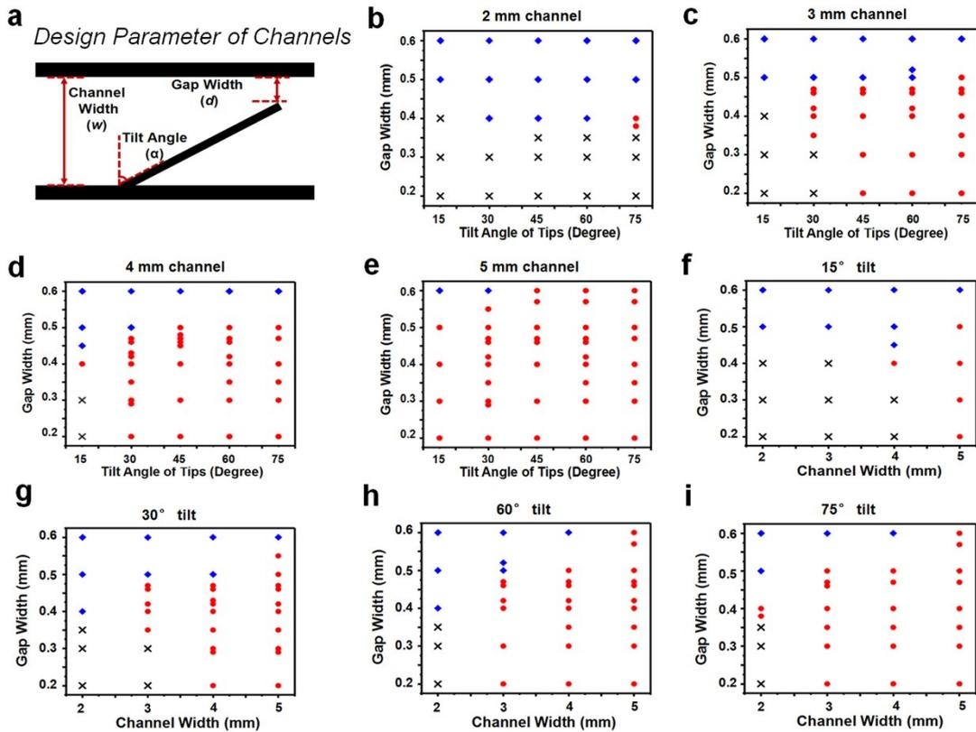
Fig. S6. The phase diagram of the directionality of single-spine channel. (a) The design parameters of the channel. (b) to (e) for the channel width from 2 to 5 mm, and (f) to (i) for the spine with a tilt angle from 15° to 75°. The similar trend was noticed as well as that of the double-spine channels.
