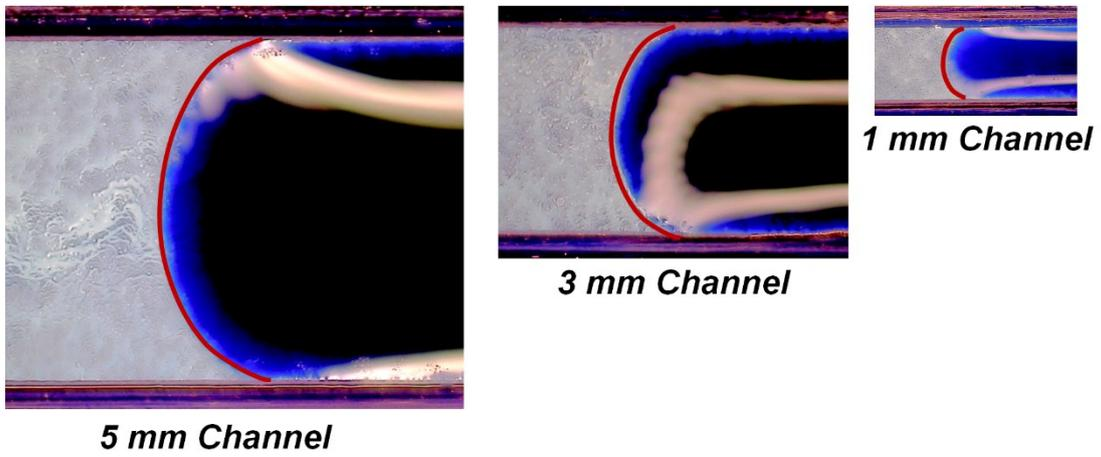
Fig. S7. The front surface of liquid flow keeps semi-circular during the liquid spreading.
