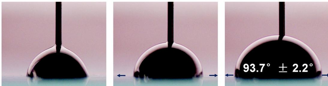
Fig. S8. The advancing angle measurement of hydrophobic ink coated surface.
