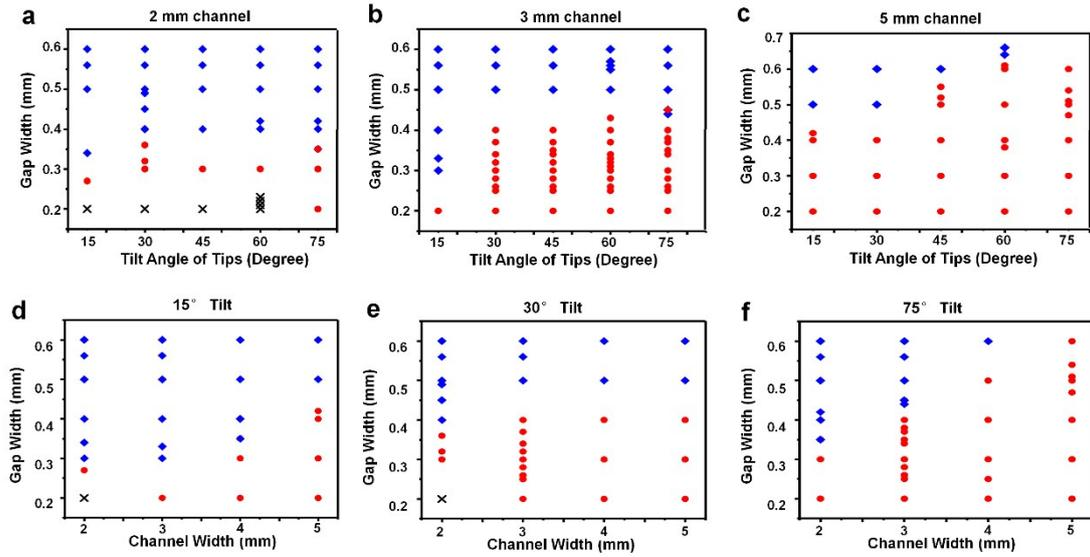
Fig. S5. The additional phase diagram of the directionality of double-spine channel. (a) 2 mm, (b) 3 mm, and (c) 5 mm channels. The spine with a tilt angle of (d) 15°, (e) 30°, and (f) 75°.
