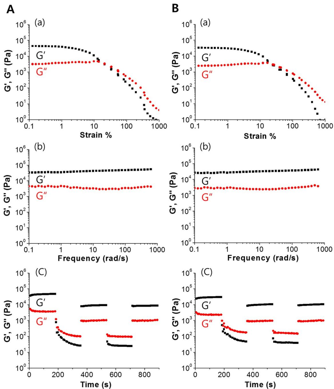
**Fig. S13** Rheological properties of **hydrogel-3S-Fe** prepared in (A) NaCl 50 mM and (B) NaCl 100 mM; (a) strain sweep tests at 0.1-1000%, (b) frequency sweep tests at 0.1-1000  $\text{rad s}^{-1}$  and strain 0.1 and (c) continuous step strain test at 0.1 and 100. All experiments were conducted at 25  $^{\circ}\text{C}$ .
