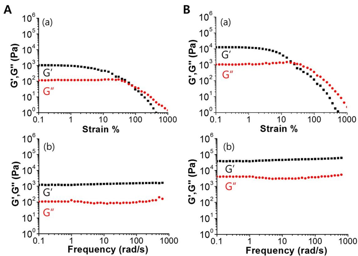
**Fig. S14** Rheological properties of (A) **organogel-Fe** and (B) **hydrogel-Fe** prepared in H<sub>2</sub>O; (a) strain sweep tests at 0.1-1000% and (b) frequency sweep tests at 0.1-1000 rad s<sup>-1</sup> and strain 0.1.
