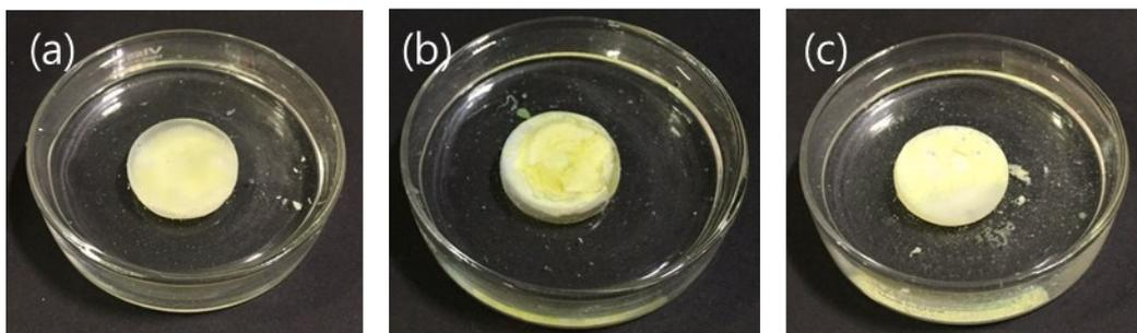
**Fig. S5** The photographs of (a) **hydrogel-1**, (b) **hydrogel-3** and (c) **hydrogel-3S-Fe** prepared by solvent exchange in the presence of 100 mM NaCl.
