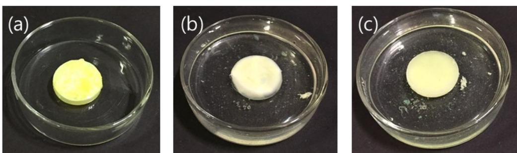
**Fig. S6** The photographs of (a) **hydrogel-1**, (b) **hydrogel-3** and (c) **hydrogel-3S-Fe** prepared by solvent exchange in the presence of 200 mM NaCl.
