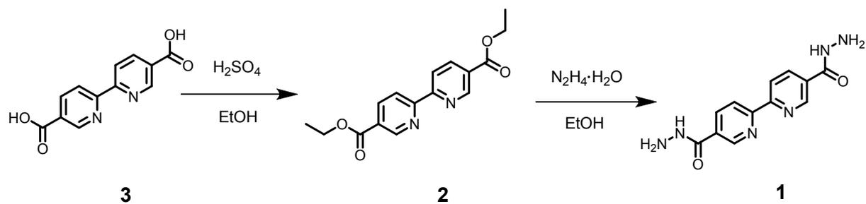
**Fig. S1** Scheme of synthetic methods for building block 1.
