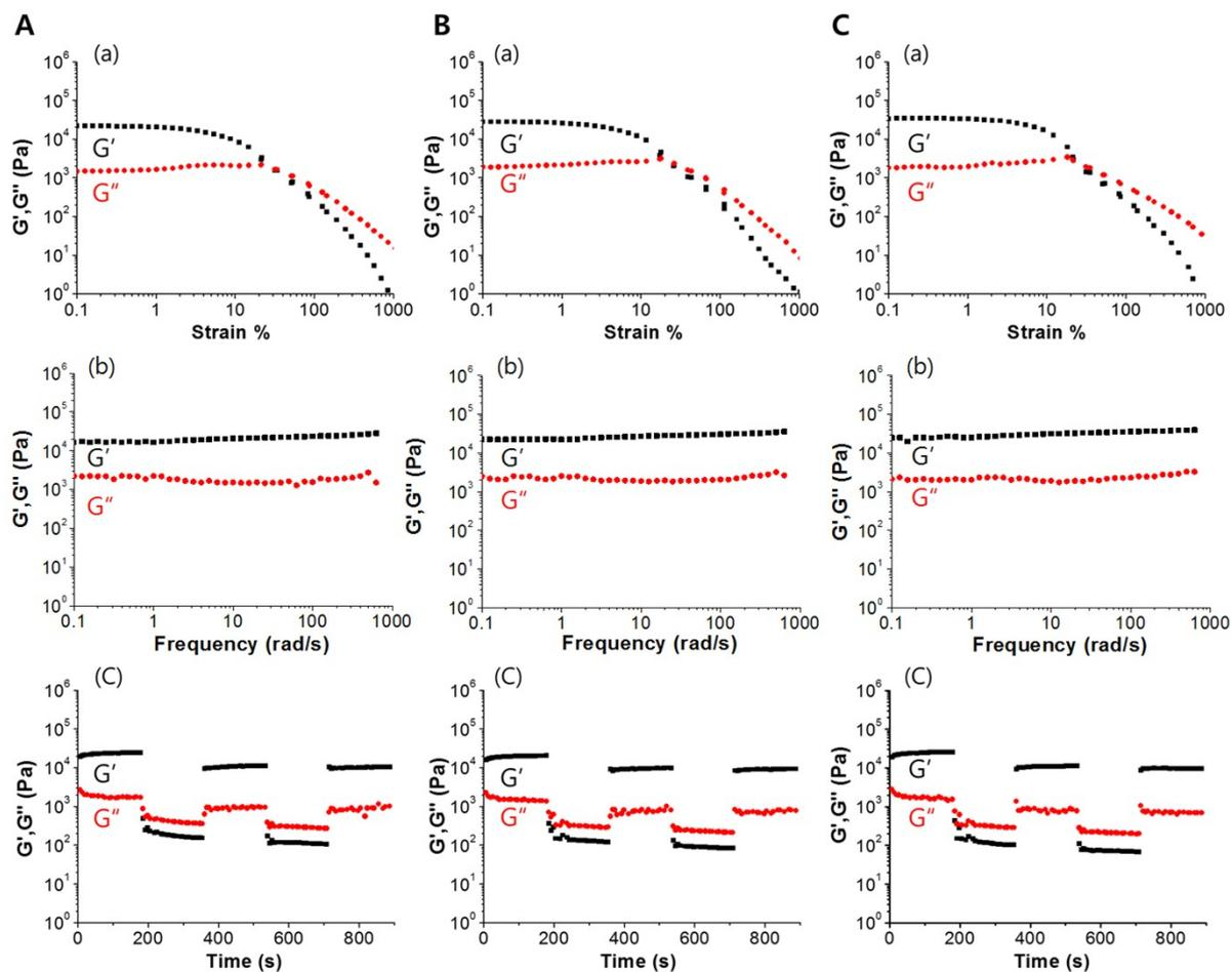
**Fig. S12** Rheological properties of (A) **hydrogel-1**, (B) **hydrogel-3S** and (C) **hydrogel-3S-Fe** prepared in NaCl (100 mM); (a) strain sweep tests at 0.1-1000%, (b) frequency sweep tests at 0.1-1000 rad s<sup>-1</sup> and strain 0.1 and (c) continuous step strain test at 0.1 and 100. All experiments were conducted at 25 °C.
