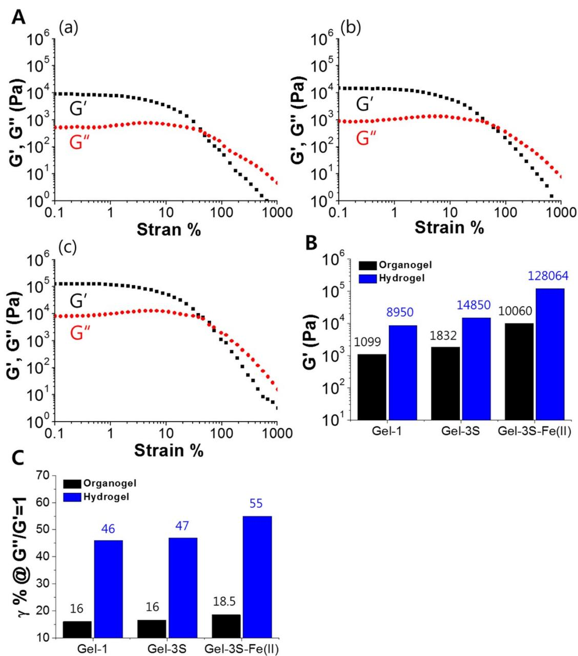
**Fig. S9** (A) Rheological properties of (a) **hydrogel-1**, (b) **hydrogel-3S** and (c) **hydrogel-3S-Fe**. (B)  $G'$  values of organogels (black) and hydrogels (blue) at  $\gamma = 0.1\%$  in A (a-c). (C)  $\gamma\%$  of organogels (black) and hydrogels (blue) at  $G''/G'=1$  in A (a-c).
