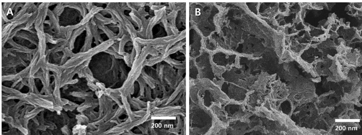
**Fig. S18** SEM images of (A) **organogel-Fe** and (B) **hydrogel-Fe**.
