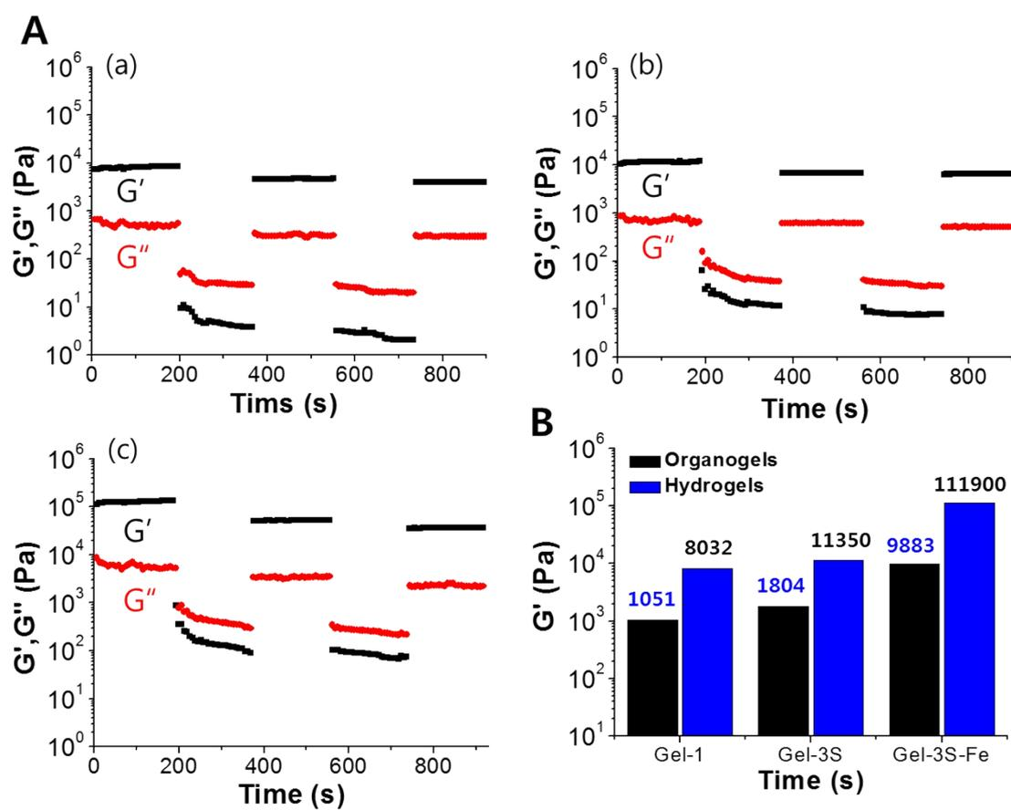
**Fig. S11** Rheological properties of (a) hydrogel-1, (b) hydrogel-3S and (c) hydrogel-3S-Fe; (A) continuous step strain test at 0.1 and 100. All experiments were conducted at 25 °C. (B) Graph of  $G'$  of organogels (black) and hydrogels (blue) at  $\gamma = 0.1\%$  in A (a–c).
