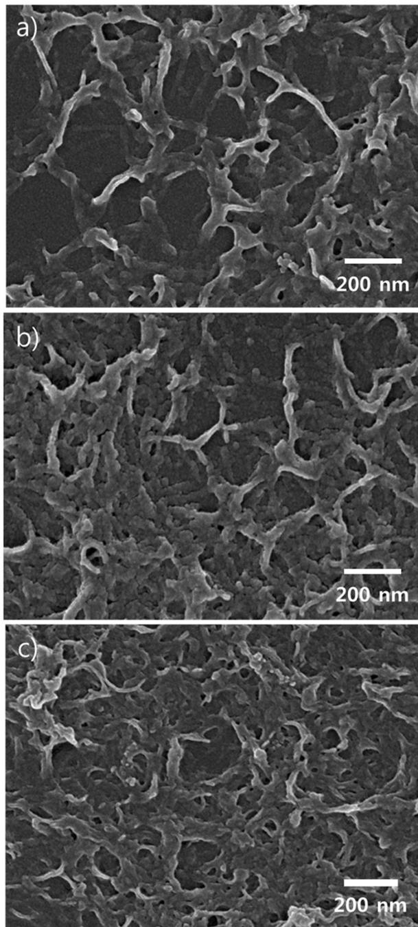
**Fig. S17** SEM images of (a) **hydrogel-1**, (b) **hydrogel-3S** and (c) **hydrogel-3S-Fe** prepared with NaCl (100 mM).
