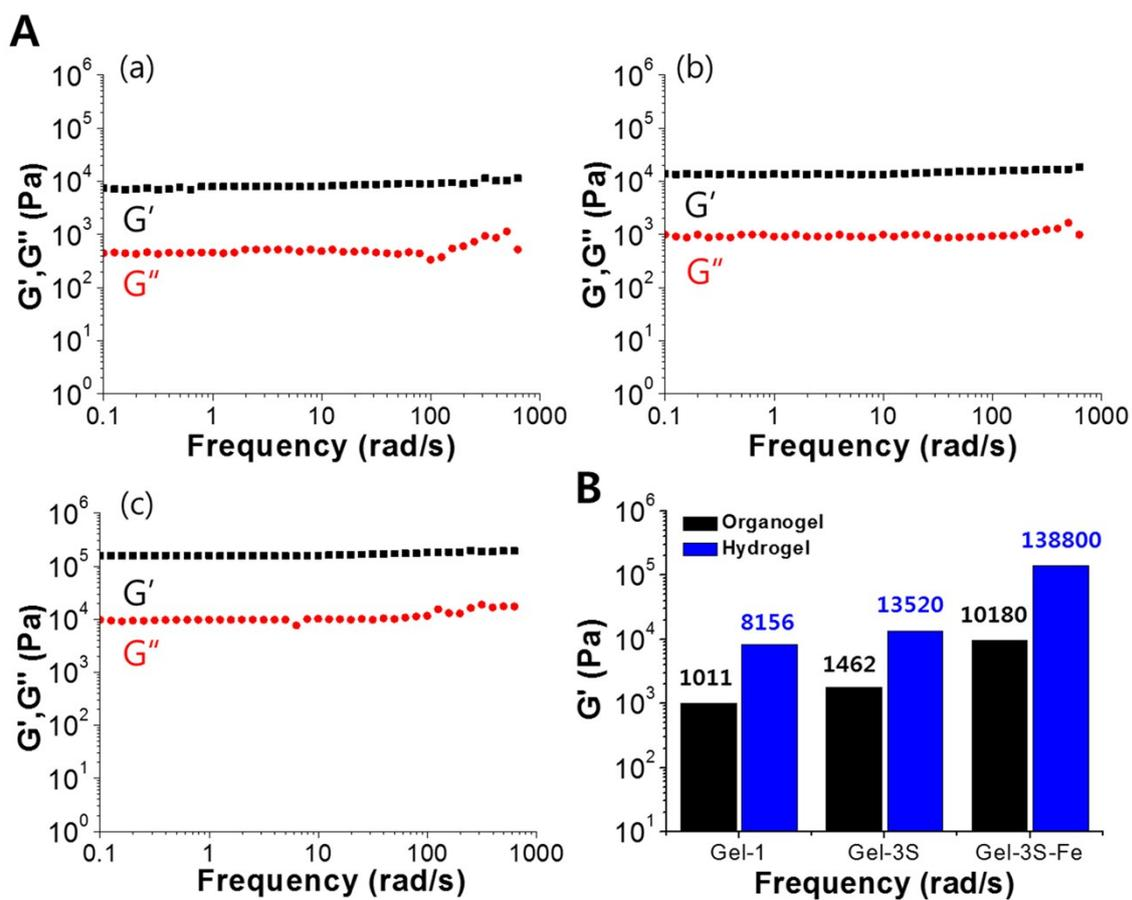
**Fig. S10** (A) Rheological properties of (a) **hydrogel-1**, (b) **hydrogel-3S** and (c) **hydrogel-3S-Fe**; (A) frequency sweep tests at 0.1-1000 rad s<sup>-1</sup> and strain 0.1. All experiments were conducted at 25 °C. (B) Graph of  $G'$  of organogels (black) and hydrogels (blue) at  $\gamma = 0.1\%$  in A (a-c).
