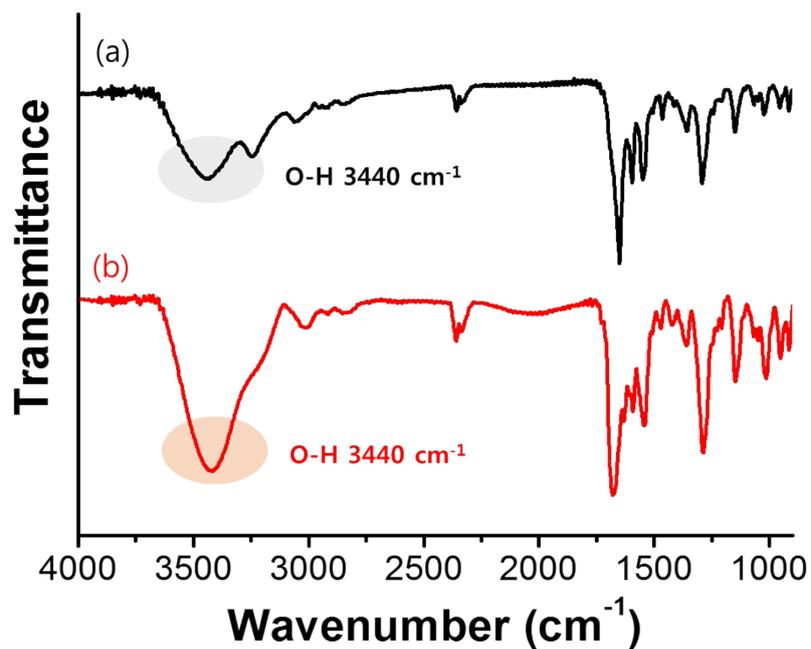
Fig. S15 FT-IR spectra of (a) organogel-1 and (b) hydrogel-1.
