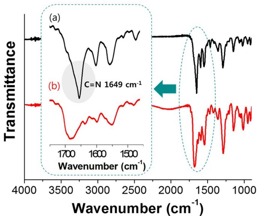
Fig. S16 FT-IR spectra of (a) organogel-1 and (b) hydrogel-1.
