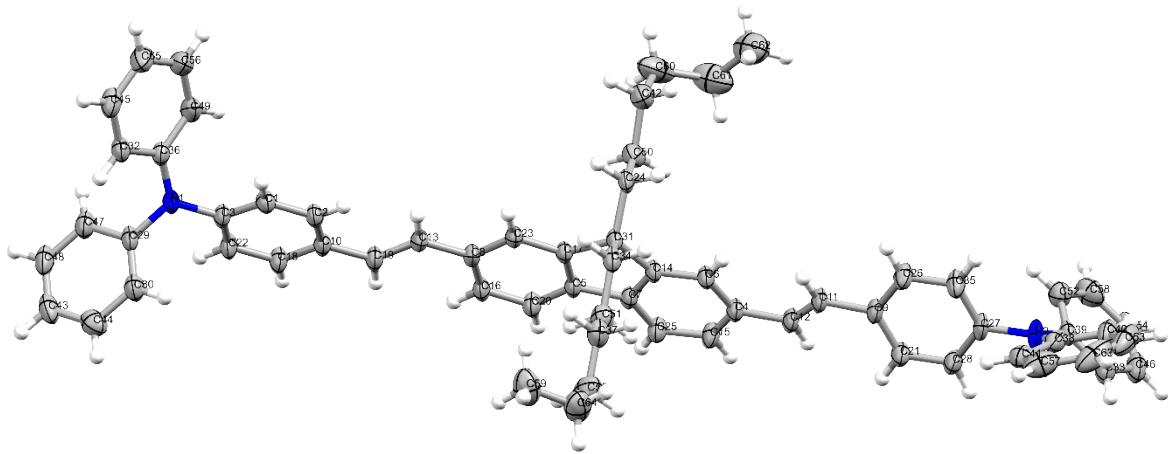
**Fig. SI-1** ORTEP view of **A1** crystal structure with ellipsoid at 50% probability.
