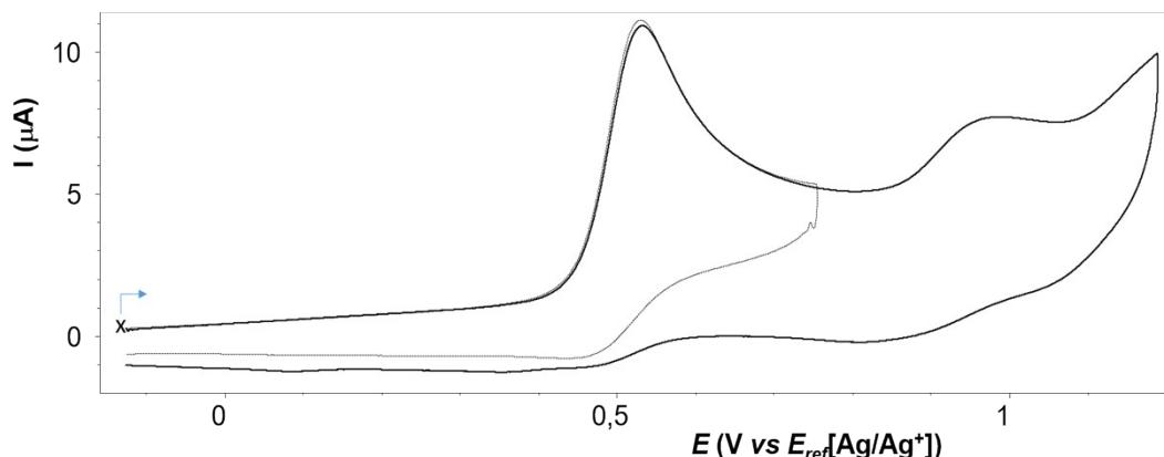
**Fig. SI-9** Voltammograms for **A3**, 1 mM in  $\text{CH}_2\text{Cl}_2$  (0.1 M TBAP) recorded under  $\text{N}_2$  (glove box); 3 mm Ø vitreous carbon working electrode,  $v = 100 \text{ mV/s}$ ,  $E$  vs  $E_{ref}[\text{Ag}/\text{Ag}^+]$ .
