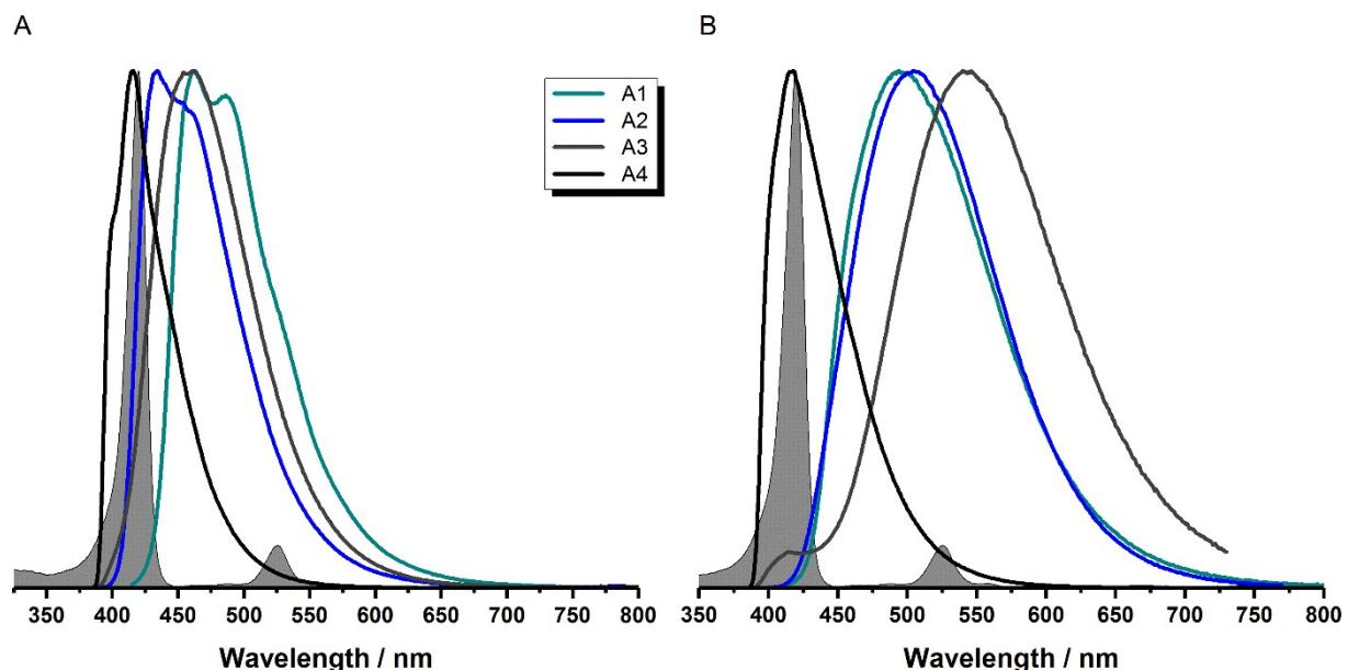
**Fig. SI-16** Absorption spectrum of C1 and emission spectra of antennae Ai (i=1-4) in A) CHCl<sub>3</sub> and B) DMF, showing the spectral overlap.
