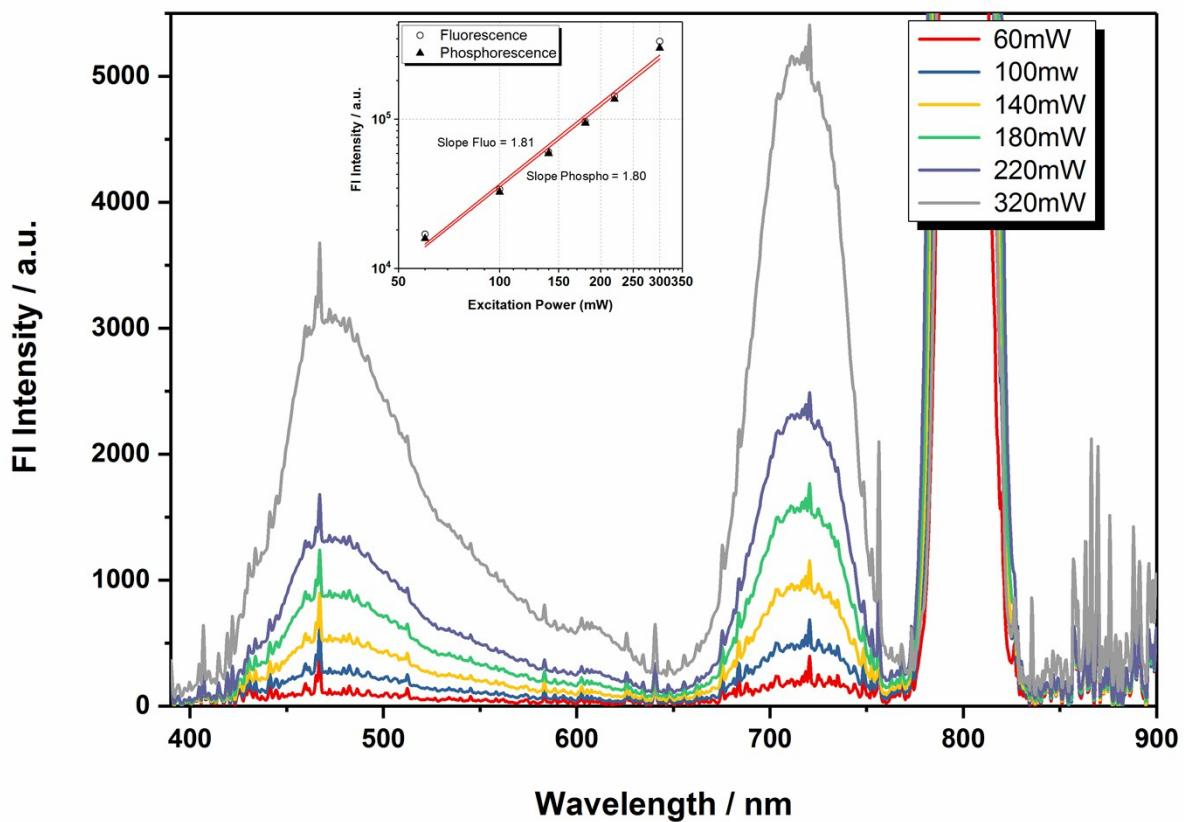
**Fig. SI-20** Emission spectra of **P1** upon two-photon excitation ( $\lambda_{\text{Laser}} = 800 \text{ nm}$ ) at different laser excitation powers. Emission spectra were recorded with a cut-off filter explaining the deformation of the red part of the phosphorescence signal. Inset: power dependence emission intensity vs laser excitation power for the residual fluorescence ( $\circ$ ) and the phosphorescence ( $\blacktriangle$ ) showing the quadratic dependence.
