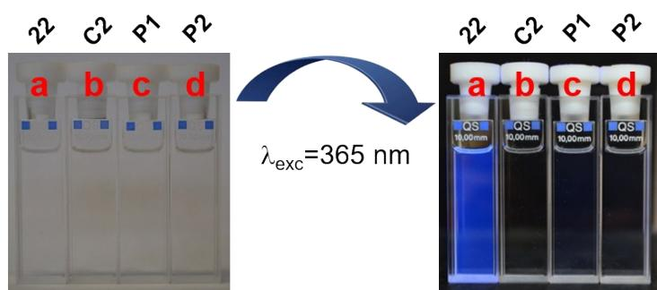
**Fig. SI-18** Picture showing the quenching of fluorescence in compounds **P1** and **P2** compared to **22**. Under a handled UV-lamp ( $\lambda_{\text{exc}} = 365 \text{ nm}$ ), the intense fluorescence of compound **22** can easily be seen (cell a), whereas compounds **P1** (cell c) and **P2** (cell d) are barely emissive. **C2** is added for comparison.
