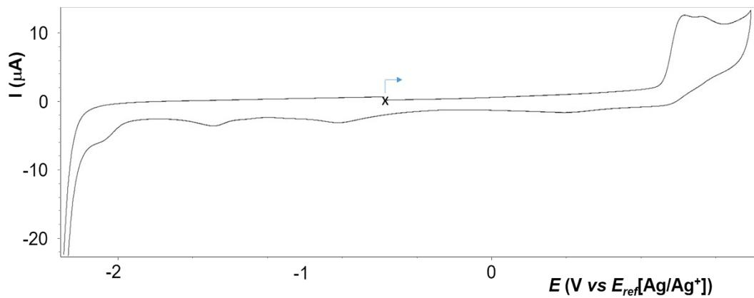
**Fig. SI-10** Voltammograms for **A4**, 1 mM in  $\text{CH}_2\text{Cl}_2$  (0.1 M TBAP) recorded under  $\text{N}_2$  (glove box); 3 mm Ø vitreous carbon working electrode,  $v = 100 \text{ mV/s}$ ,  $E$  vs  $E_{\text{ref}}[\text{Ag}/\text{Ag}^+]$ .
