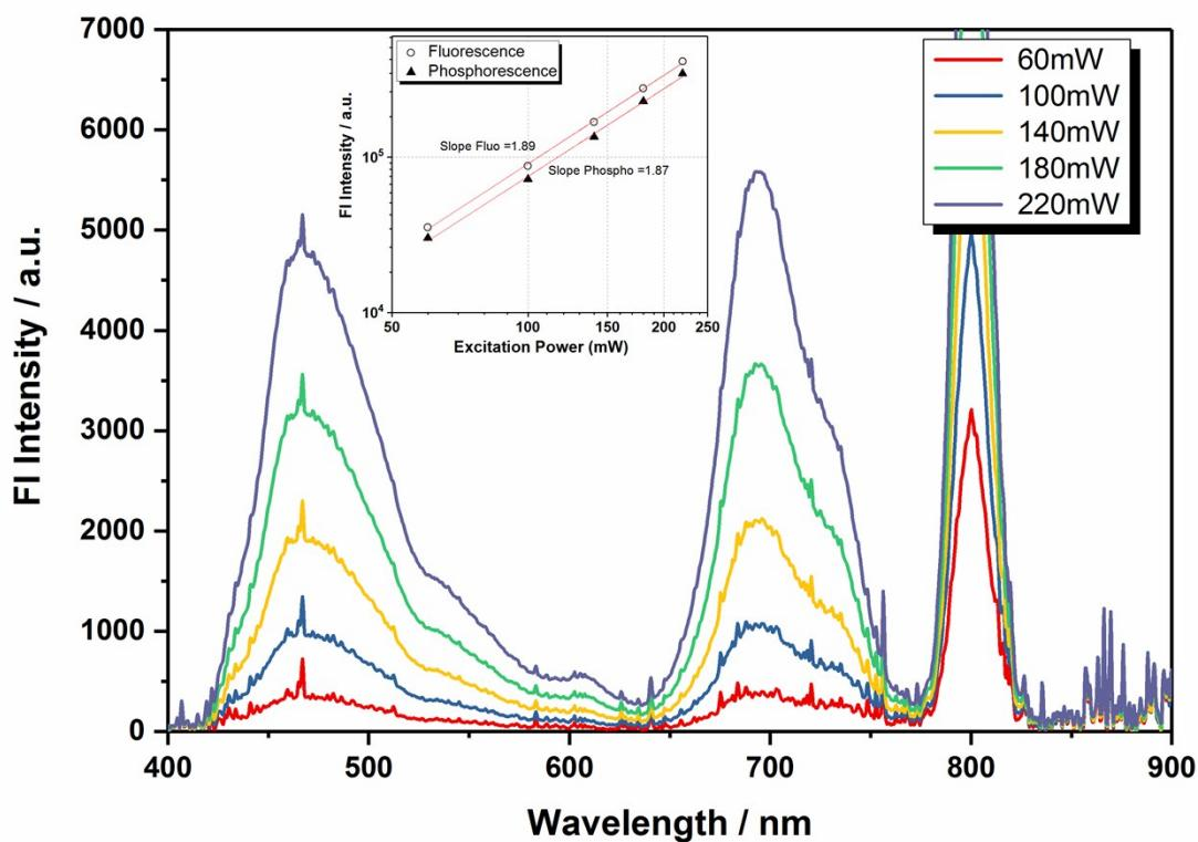
**Fig. SI-21** Emission spectra of **P1** upon two-photon excitation ( $\lambda_{\text{Laser}} = 800 \text{ nm}$ ) at different laser excitation powers. Emission spectra were recorded with a cut-off filter explaining the deformation of the red part of the phosphorescence signal. Inset: power dependence emission intensity vs laser excitation power for the residual fluorescence ( $\circ$ ) and the phosphorescence ( $\blacktriangle$ ) showing the quadratic dependence.
