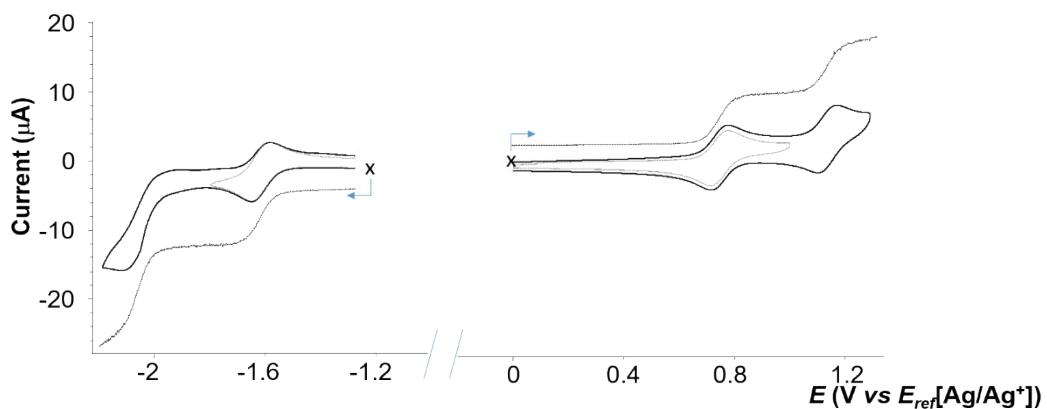
**Fig. SI-5** Voltammograms for **C1**, 1 mM in CH<sub>2</sub>Cl<sub>2</sub> (0.1 M TBAP) recorded under N<sub>2</sub> (glove box); 3 mm Ø vitreous carbon working electrode,  $v = 100$  mV/s,  $E$  vs  $E_{ref}$ [Ag/Ag<sup>+</sup>]. RDE 10 mV/S, 500 rd/min.
