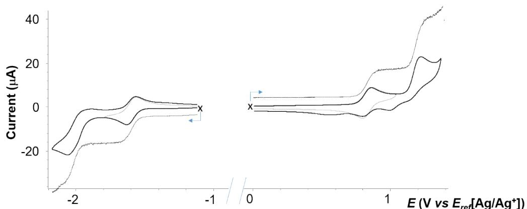
**Fig. SI-6** Voltammograms for **C2**, 1 mM in CH<sub>2</sub>Cl<sub>2</sub> (0.1 M TBAP) recorded under N<sub>2</sub> (glove box); 3 mm Ø vitreous carbon working electrode,  $v = 100$  mV/s,  $E$  vs  $E_{ref}$ [Ag/Ag<sup>+</sup>]. RDE 10 mV/S, 500 rd/min.
