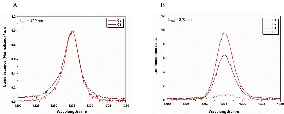
**Fig. SI-19** A) Singlet oxygen luminescence observed in aerated dichloromethane solution of **C1** and **C2** following irradiation in the Soret band at  $\lambda_{\text{exc}} = 420 \text{ nm}$ . B) Singlet oxygen luminescence observed in aerated dichloromethane solution of **P1** and **P2** following irradiation in the antenna at  $\lambda_{\text{exc}} = 370 \text{ nm}$ . Note that for this excitation wavelength the generation of singlet oxygen by **C1** and **C2** is negligible.
