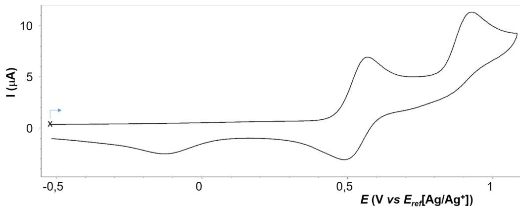
**Fig. SI-7** Voltammograms for **A1**, 1 mM in  $\text{CH}_2\text{Cl}_2$  (0.1 M TBAP) recorded under  $\text{N}_2$  (glove box); 3 mm Ø vitreous carbon working electrode,  $v = 100 \text{ mV/s}$ ,  $E$  vs  $E_{ref}[\text{Ag}/\text{Ag}^+]$ .
