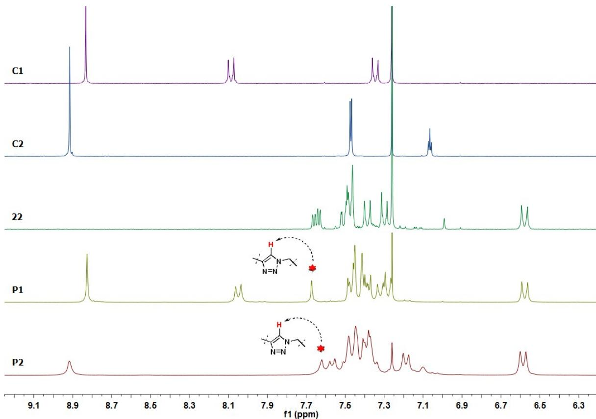
**Fig. SI-17** Comparative figure of the aromatic part of the <sup>1</sup>H NMR spectra (300 MHz) for **C1**, **C2**, **22**, **P1** and **P2** showing the appearing of the characteristic triazole proton for compound **P1** and **P2**.
