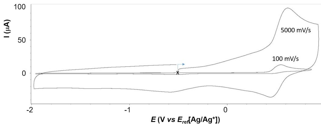
**Fig. SI-8** Voltammograms for **A2**, 1 mM in  $\text{CH}_2\text{Cl}_2$  (0.1 M TBAP) recorded under  $\text{N}_2$  (glove box); 3 mm Ø vitreous carbon working electrode,  $v = 100 \text{ mV/s}$ ,  $E$  vs  $E_{ref}[\text{Ag}/\text{Ag}^+]$ .
