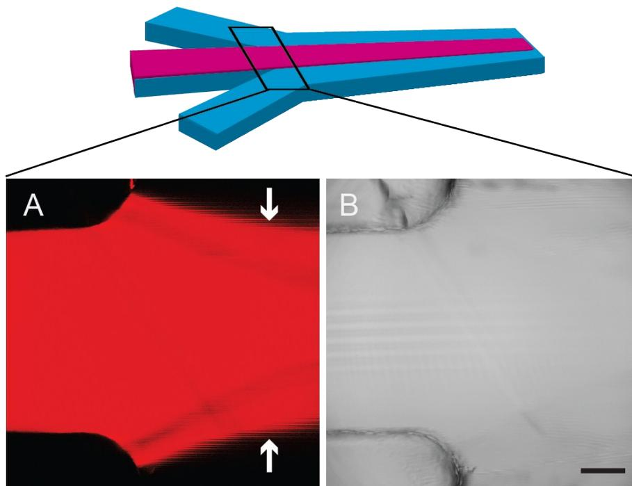
Figure S3. (A) confocal microscopy image; (B) corresponding bright field image of the section where flow from 3 inlets meets, the white arrows point to the phase boundary. The scale bar represents 200  $\mu\text{m}$ . Polymer/Nile red organic solution was injected through the middle inlet while aqueous solution was pumped in through 2 side inlets. Polymeric structures were formed at the periphery of the two phases.
