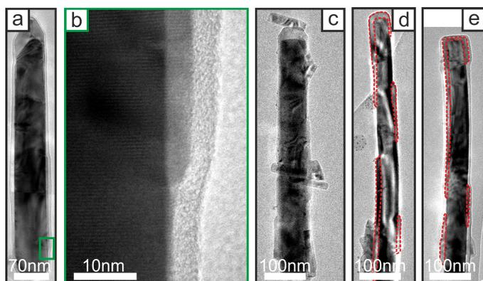
**Fig. 7** (a) Cross-sectional TEM image of a GaN-(Al,Ga)N core-shell NW with a thicker core diameter of 64 nm after 3' shell growth. (b) High magnification image of a distinct location along the NW side facet of (a). The outer amorphous layer is assigned to contamination due to the NW dispersion. (c) Cross-sectional TEM image of a core-shell NW showing a cracking of shell nuclei. (d,e) Different core-shell NWs with a thinner core.
