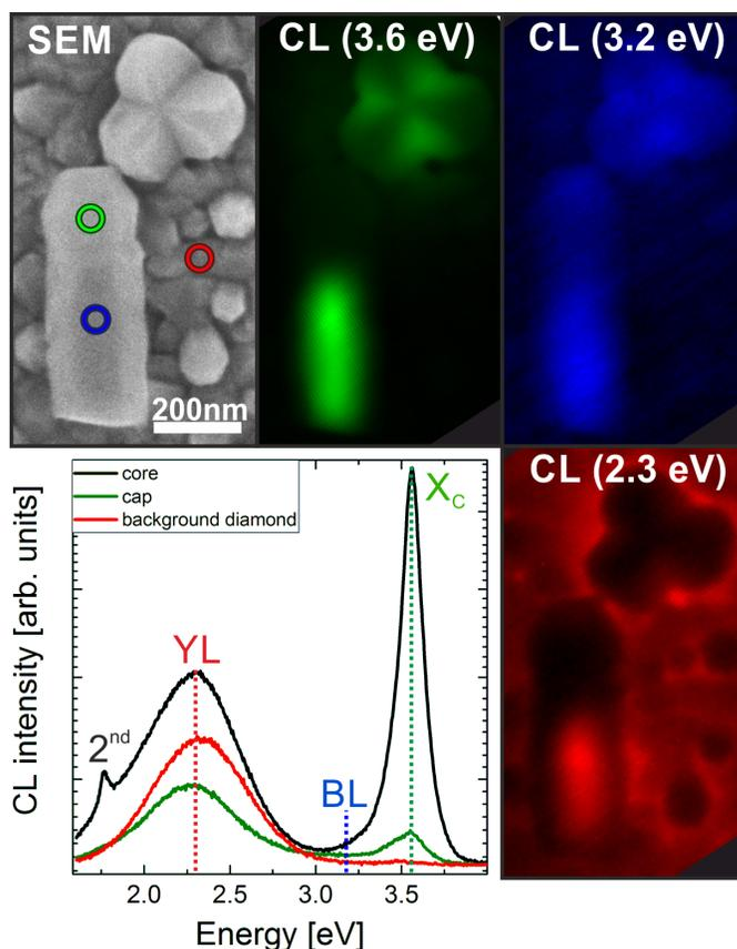
**Fig. 4** SEM image, CL maps and CL spectra of distinct sites along a GaN-(Al,Ga)N core-shell NW grown on diamond substrate. The colored circles in the SEM image indicates the sites where the CL spectra have been recorded. The CL maps are at an equivalent sites and refer to different spectral emissions. 'Green' refers to 3.6 eV, 'Blue' and 'red' correspond to 3.2 eV and 2.3 eV, respectively.
