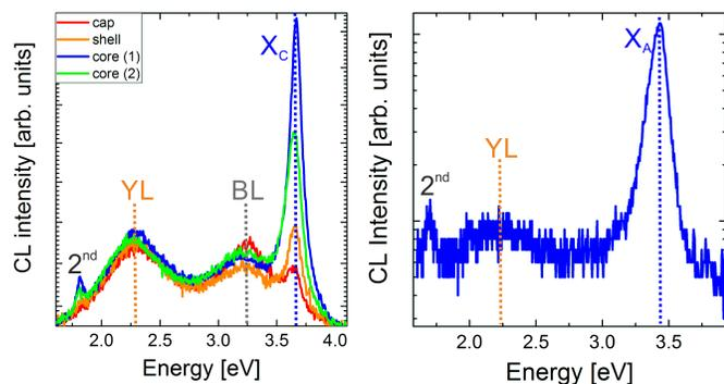
**Fig. 3** (Left) CL spectra of distinct sites along a GaN-(Al,Ga)N core-shell NW. The curves represent the vertically unshifted data of Figure 3b in the main article. (Right) CL spectrum of self-assembled GaN NWs on Si.
