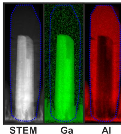
**Fig. 6** Cross-sectional STEM image of a GaN-(Al,Ga)N core-shell NW grown on Si substrate with corresponding false-colored EDX maps of the atomic species Ga (green) and Al (red). As a guide to the eye, the core-shell NW is indicated by blue dashed lines.
