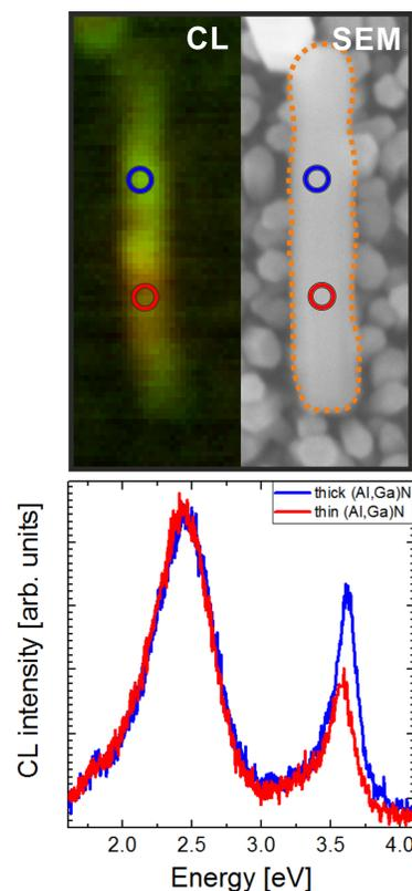
**Fig. 8** Room temperature CL spectra of a GaN-(Al,Ga)N core-shell NW thin and thick (Al,Ga)N shell segments along the growth direction with corresponding false-colored CL map and SEM image of the NW.
