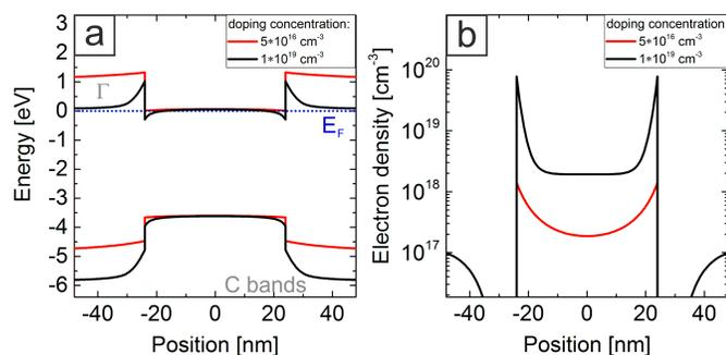
**Fig. 1** (a) Electronic band structure of the GaN-(Al,Ga)N core-shell NW cross section for different doping concentrations and (b) corresponding electron density.
