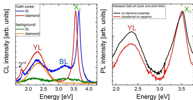
**Fig. 5** (Left) CL spectra of the GaN cores and the background signal of the substrates for GaN-(Al,Ga)N core-shell NWs grown on Si and diamond. (Right) PL spectra of GaN-(Al,Ga)N core-shell NWs lying on their original diamond substrate and of transferred NWs on sapphire.
