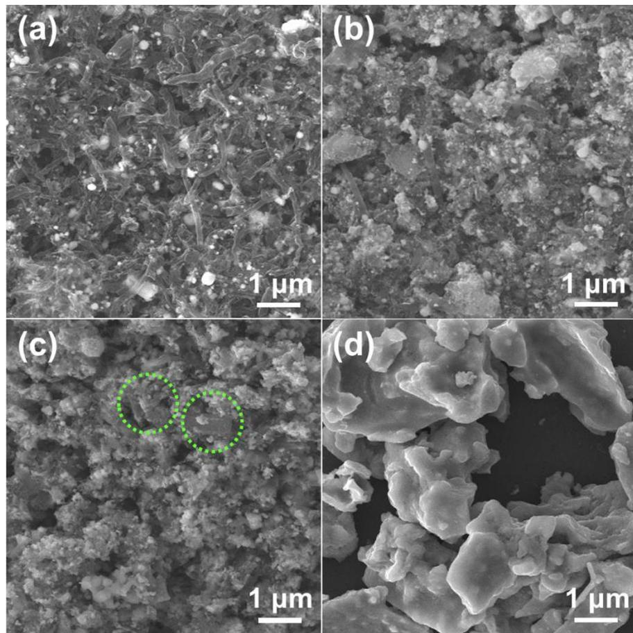
**Fig. S3** SEM images of sample (a)  $\text{Ni}_{2.0}\text{Mo}_0@\text{NC}$ , (b)  $\text{Ni}_{2.0}\text{Mo}_{0.13}@\text{NC}$ , (c)  $\text{Ni}_{2.0}\text{Mo}_{0.39}@\text{NC}$ , and (d)  $\text{Ni}_0\text{Mo}_{0.26}@\text{NC}$ .
