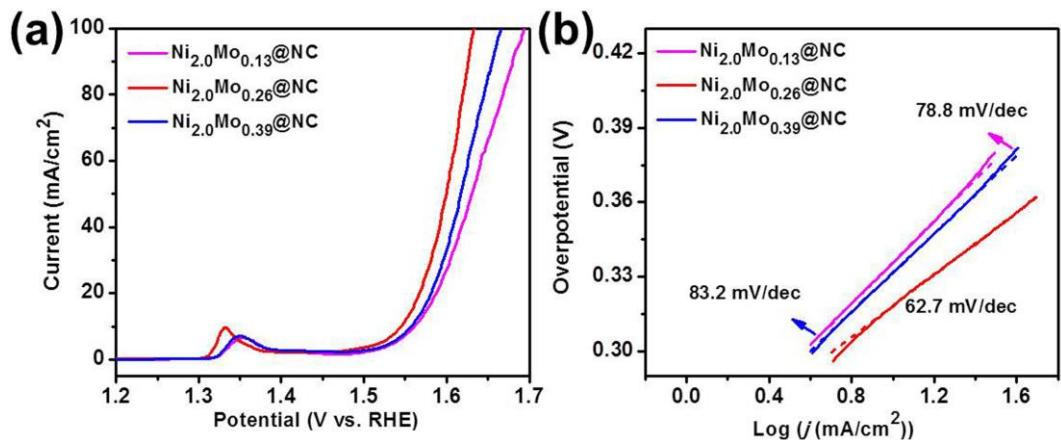
**Fig. S7** (a) LSV plots for different samples after  $iR$  compensation in 1 M KOH at a scan rate of  $5 \text{ mV s}^{-1}$  and a rotating speed of 1600 rpm. (b) Corresponding Tafel plots.
