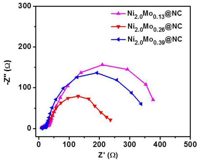
**Fig. S9** EIS plots of sample  $\text{Ni}_{2.0}\text{Mo}_{0.13}\text{@NC}$ ,  $\text{Ni}_{2.0}\text{Mo}_{0.26}\text{@NC}$  and  $\text{Ni}_{2.0}\text{Mo}_{0.39}\text{@NC}$ .
