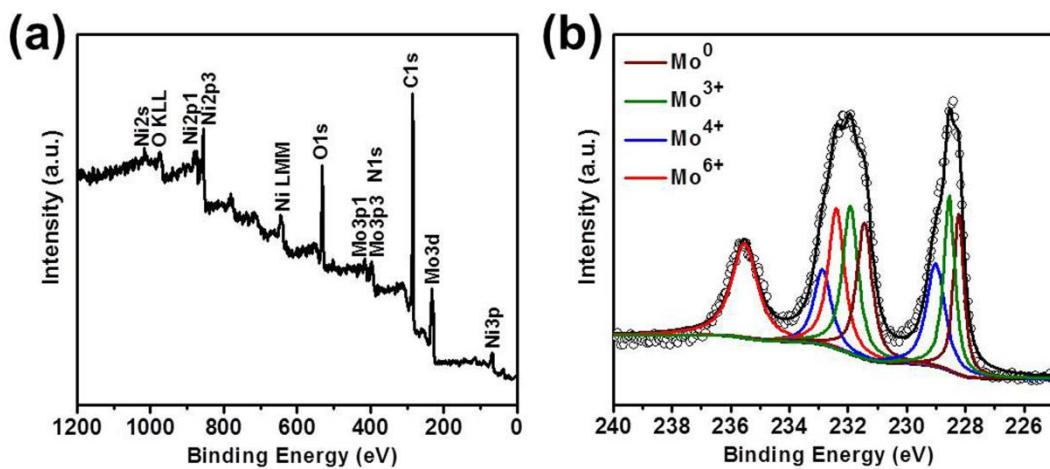
**Fig. S2** (a) XPS survey spectrum and (b) high-resolution XPS spectrum of Mo 3d for sample  $\text{Ni}_{2.0}\text{Mo}_{0.26}@\text{NC}$ .
