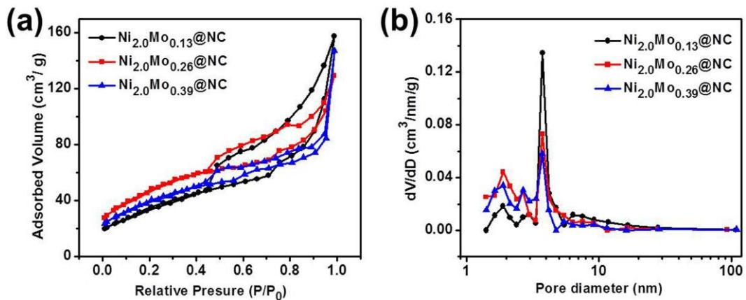
**Fig. S8** (a) Nitrogen adsorption and desorption isotherm and (b) BJH pore distribution of sample Ni<sub>2.0</sub>Mo<sub>0.13</sub>@NC, Ni<sub>2.0</sub>Mo<sub>0.26</sub>@NC and Ni<sub>2.0</sub>Mo<sub>0.39</sub>@NC.
