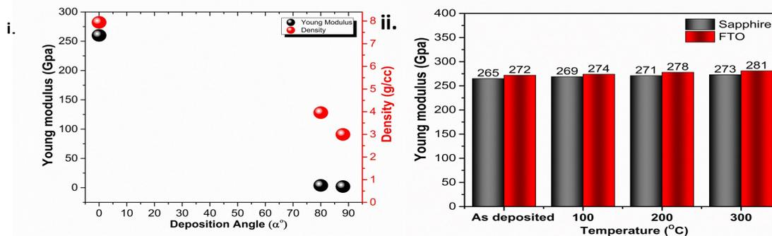
Figure S4. i) Young's Modulus and density variation as a function of deposition angle for asdeposited single layer  $\text{HfO}_2$  thin film ii) Graphical representation of calculated young modulus of as deposited and annealed films .
