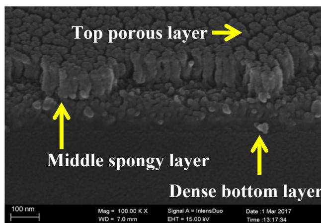
Figure S1: SEM image of TAR-H coating at tilt angle of 45°
