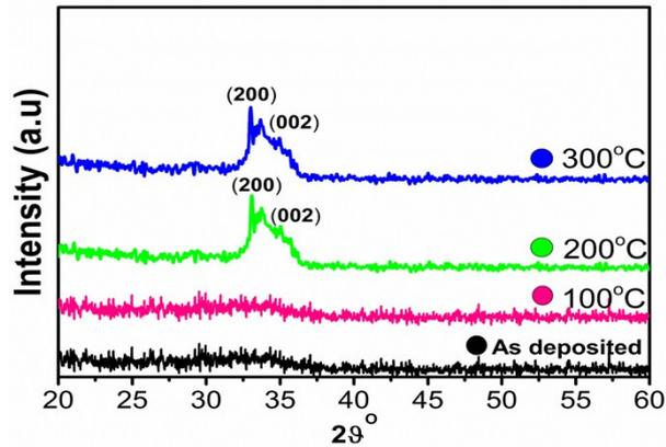
Figure S3. XRD analysis of annealed and asdeposited TAR-H
