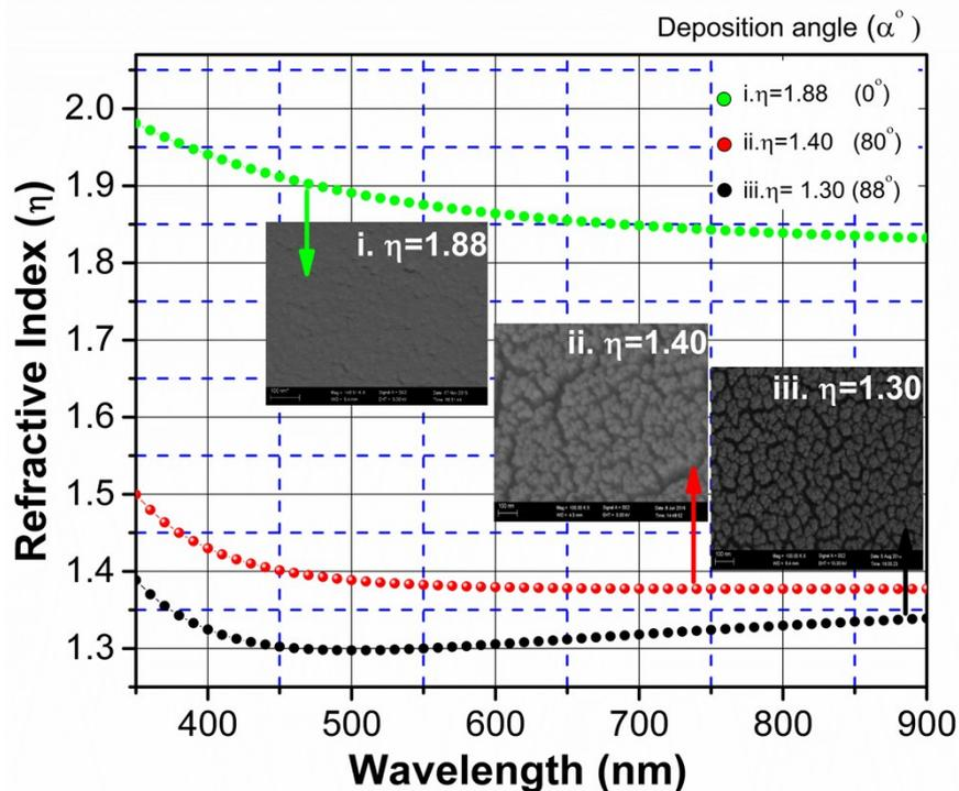
**Figure S2.** Refractive index ( $n$ ) of  $\text{HfO}_2$  single layers films measured as a function of wavelength at 550nm. Inset showing the top view image of individual hafnia layers deposit at different oblique angles.
