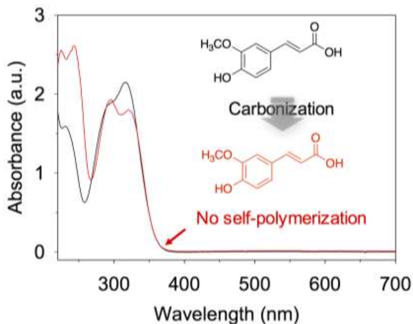
Figure S3. UV-Vis spectra of ferulic acid before (black) and after (red) sulfuric acid-based carbonization.
