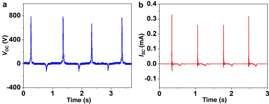
**Fig. S5** (a) Output voltage measured from two P-TENGs ( $10 \text{ cm} \times 15 \text{ cm}$  each) when they were connected in series. (b) Output current of these two P-TENGs when they were connected in parallel.
