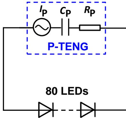
**Fig. S7** The equivalent circuit for powering 80 LEDs connected in series by the P-TENG.
