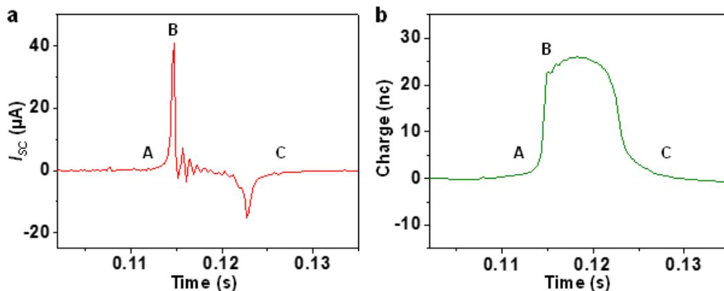
**Fig. S1** (a) Output current produced from one friction cycle of the P-TENG. (b) The corresponding induced charge calculated by the integral area of the  $I-t$  curve in (a).
