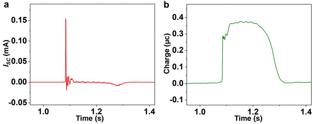
**Fig. S4** (a) One cycle output current of a P-TENG within the book. (b) The corresponding output charge calculated from the integral area of the  $I-t$  curve in (a).
