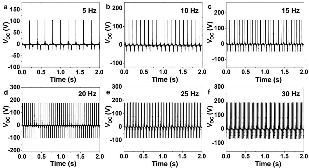
**Fig. S3** Output voltage signals of the P-TENG to a range of varying oscillation frequencies.
