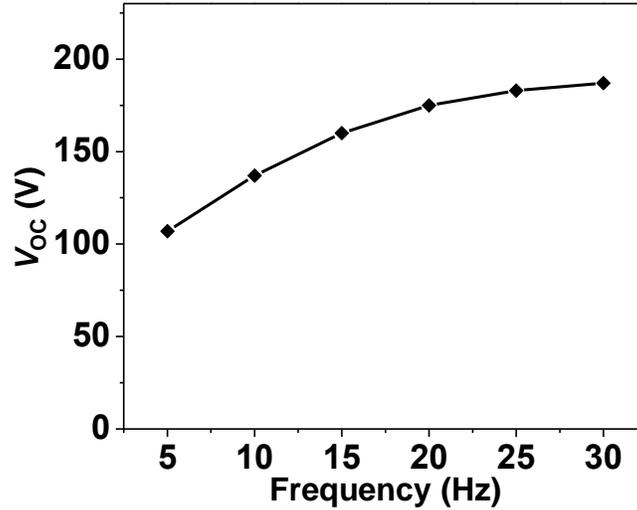
**Fig. S2** The peak  $V_{OC}$  of the P-TENG under oscillation frequencies from 5 to 30 Hz.
