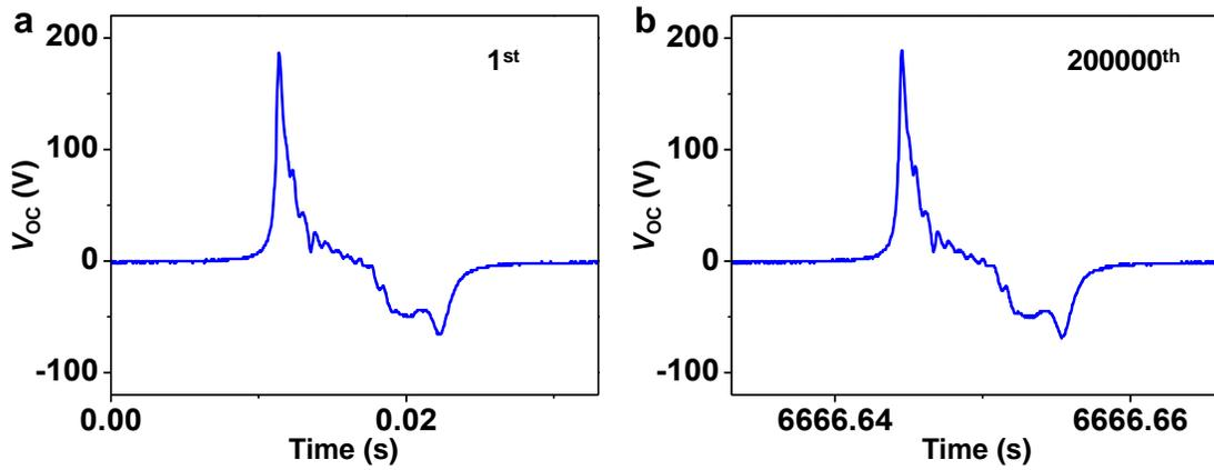
**Fig. S6** The enlarged voltage output patterns of the 1<sup>st</sup> and 200000<sup>th</sup> cycle in Fig. 4a.
