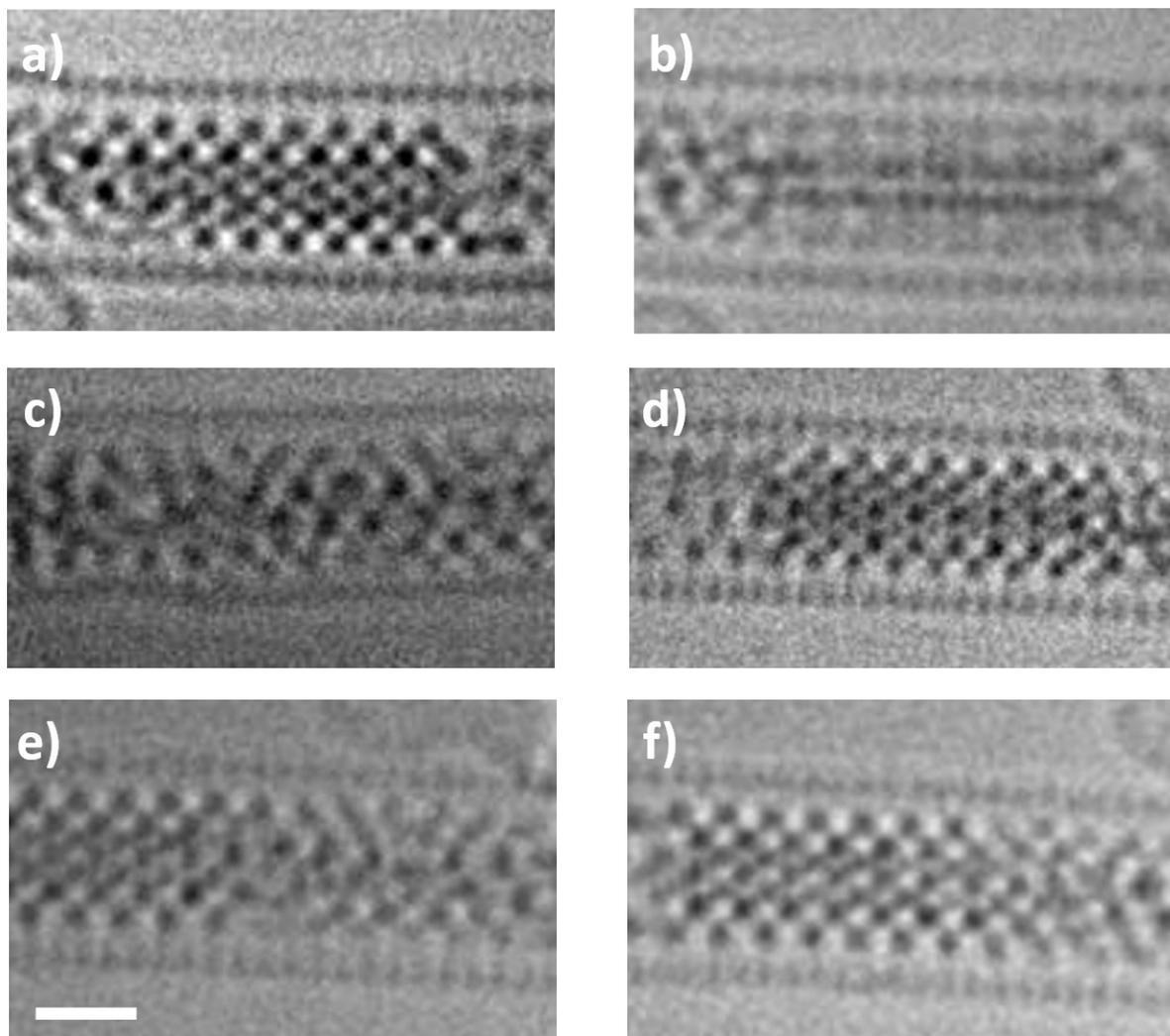
**Figure S-8: (a-f) AC-HRTEM images (80 kV) showing different projections of PtI<sub>2</sub>@SWNT. The scale bar is 0.5 nm.**
