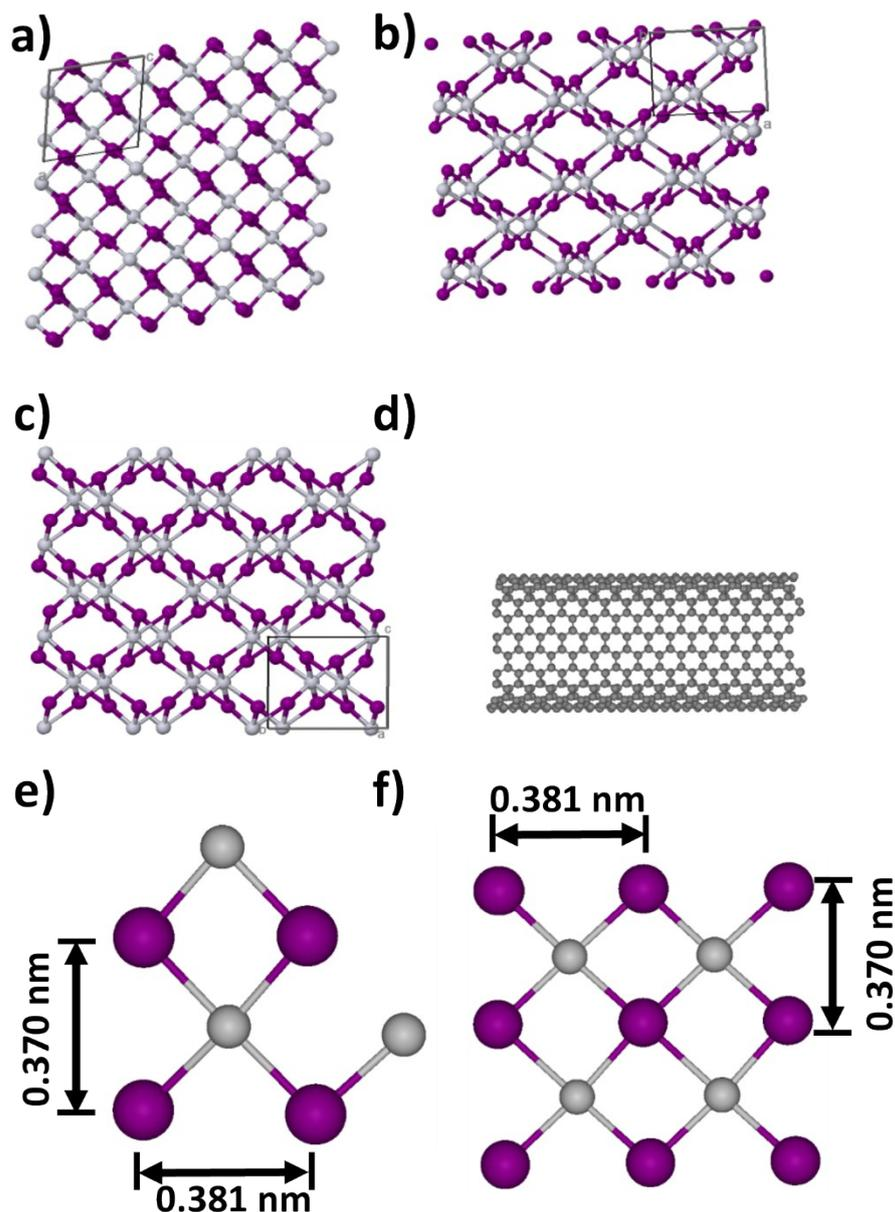
**Figure S-11: a-c) Extended crystal structure of bulk  $\text{PtI}_2$  in different orientations.  $\text{PtI}_2$  as a monoclinic unit cell with space group  $P2(1)/c$ ; d) A (11,11) SWNT has a diameter of ca. 1.5 nm and is shown for scale; The cubic structure from figure 5 b was derived from the asymmetric unit of  $\text{PtI}_2$  (e) which has been extended to form the basis of the cubic crystal plane (f).**
