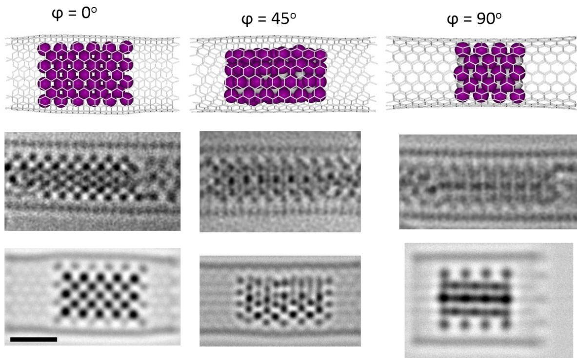
Figure S-7: Series showing a model of PtI<sub>2</sub>@SWNT (top row) with the corresponding HR-TEM image (80 kV, middle row) and image simulation (QSTEM, 20 slices per image, bottom row). The model has been tilted by 45° (middle column) and 90° (right column). The corresponding HR-TEM images and subsequent simulations are shown underneath each model.
