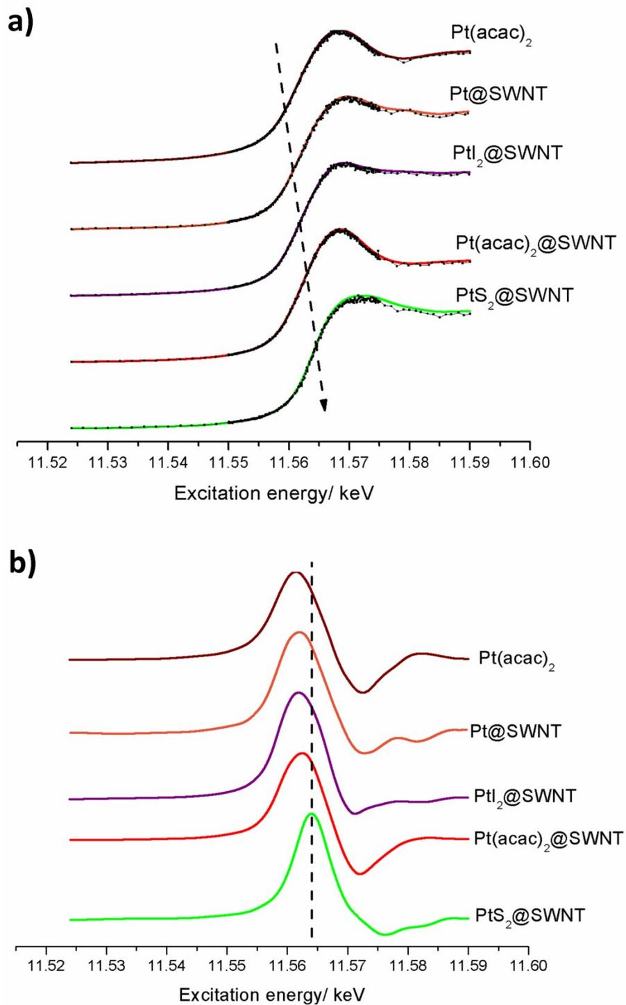
**Figure S-1: Pt L<sub>III</sub> edge spectra of Pt materials formed using a stepwise approach (a). The raw data is shown by the black plot, and the smoothed data is overlaid in colour in each case.**
