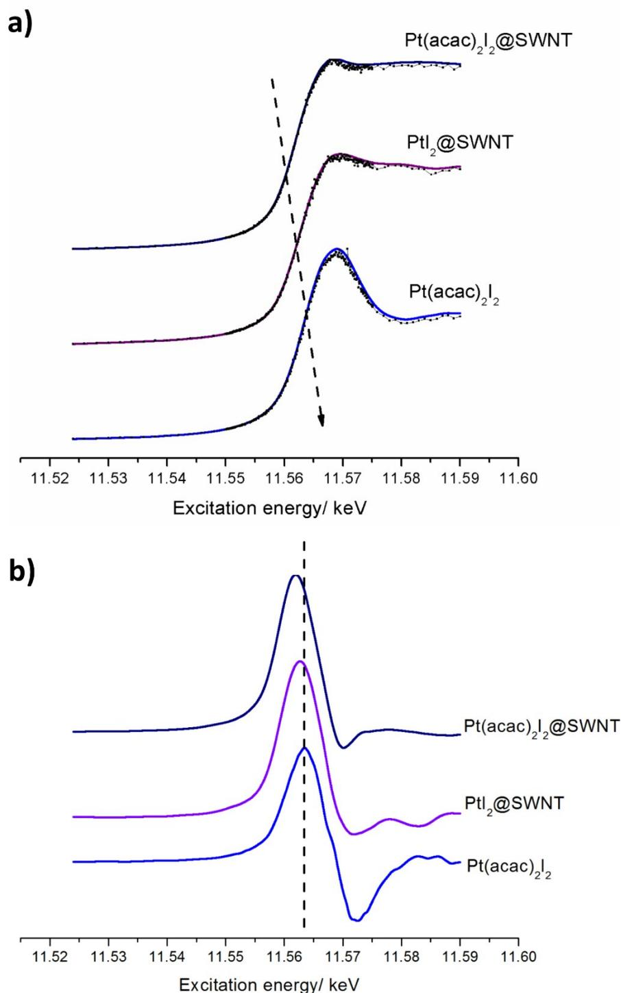
Figure S-2: Pt L<sub>III</sub> edge spectra of Pt and I containing materials formed using a one-pot filling approach (a). The raw data is shown by the black plot, and the smoothed data is overlaid in colour in each case. The first derivative (b) of each smoothed spectrum is shown, to determine the excitation edge position.
