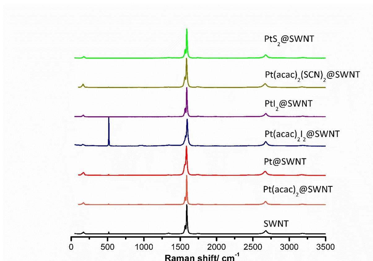
**Figure S-6: Raman Spectra of all synthesised materials to show differences from that of an empty SWNT. All spectra were recorded at room temperature using a HoribaJY LabRAM HR spectro-meter, laser wavelength 532 nm. Samples were recorded by dispersing in propan-2-ol and drop-casting onto silicon (100) supports. The additional peal at 520.7 cm<sup>-1</sup> in the spectrum of Pt(acac)<sub>2</sub>I<sub>2</sub>@SWNT is associated with the known optical phonon mode of the Si(100) support.**
