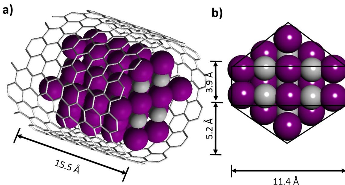
**Figure S-12: A model of  $\text{PtI}_2@SWNT$  showing how density was calculated. A crystal of  $\text{Pt}_{28}\text{I}_{56}$  of length  $15.5 \text{ \AA}$  is inside a SWNT (a); b) the surface area of the crystal face was approximated using simple geometrical units and multiplied by the length of the crystal ( $15.5 \text{ \AA}$ ). This gave a crystal volume of  $1607.35 \text{ \AA}^3$ , which equates to a density of  $11.60 \text{ gcm}^{-3}$ .**
