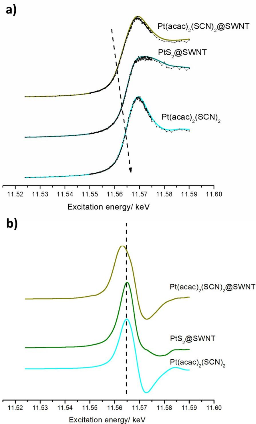
Figure S-3: Pt L<sub>III</sub> edge spectra of Pt and S containing materials formed using a one-pot filling approach (a). The raw data is shown by the black plot, and the smoothed data is overlaid in
