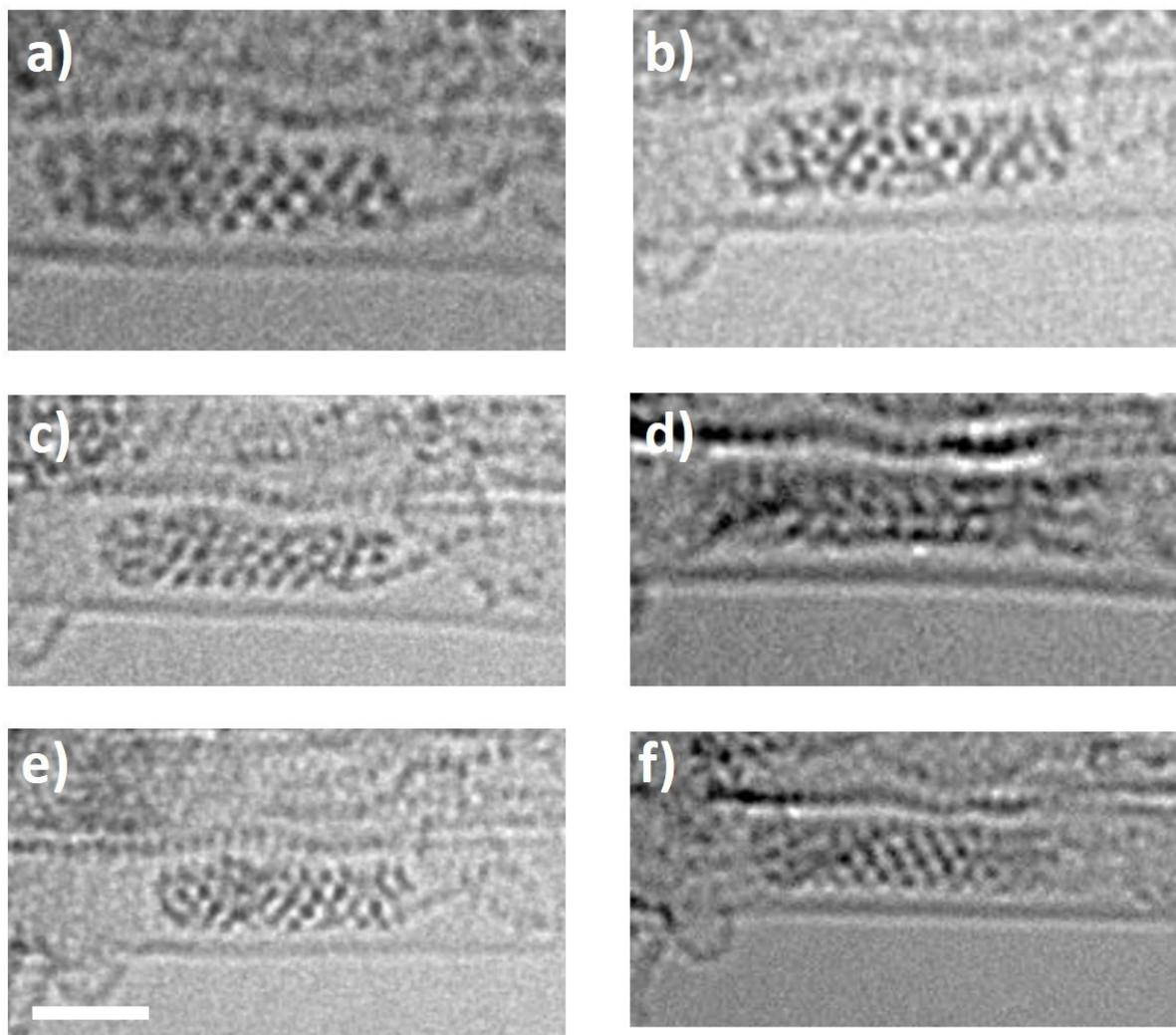
Figure S-9: (a-f) AC-HRTEM images (80 kV) showing different projections of PtS<sub>2</sub>@SWNT. The scale bar is 1 nm.
