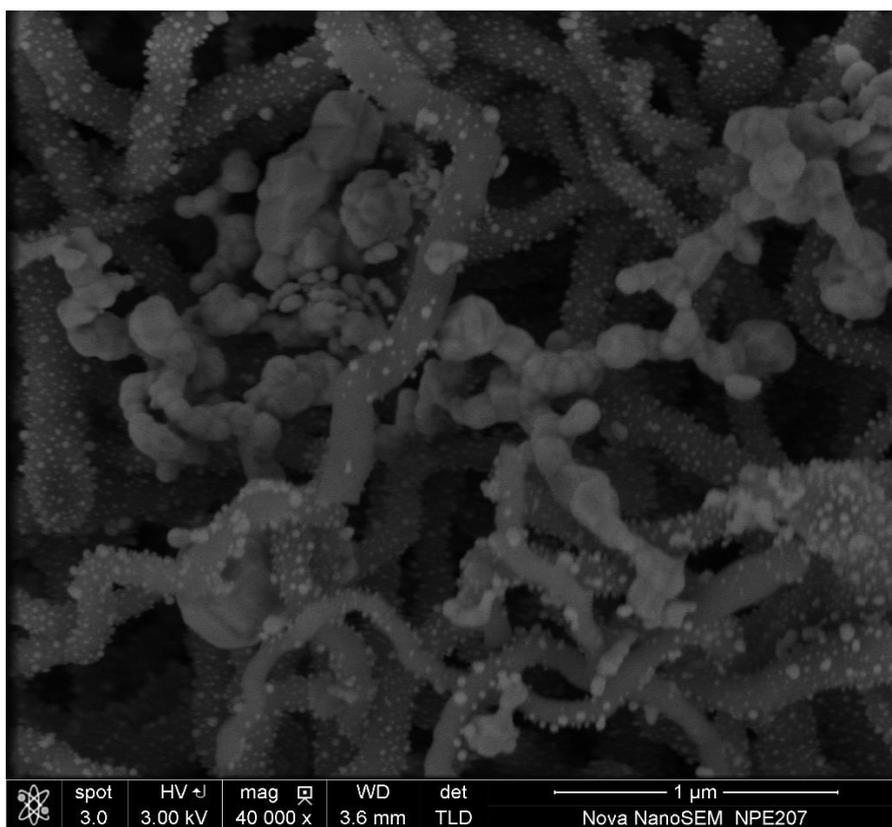
**Fig. S5** SEM image of the AgNPs-deposited SiO<sub>2</sub> NW membrane prepared with a AgNO<sub>3</sub> concentration of 1.5 mg mL<sup>-1</sup>.
