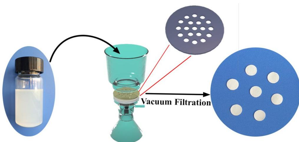
**Fig. S1** The experimental setup used to assemble the free-standing SiO<sub>2</sub> NW membrane.
