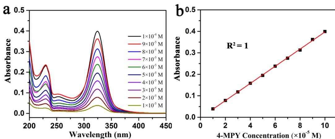
**Fig. S7** (a) UV-Visible spectra of 4-MPY solution at different concentrations. (b) Calibration curve used for the measurement of 4-MPY absorption on the SERS membrane using the peak at 325 nm.
