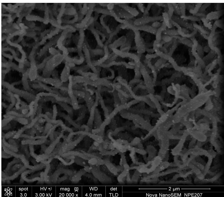
**Fig. S4** SEM image of the AgNPs-deposited SiO<sub>2</sub> NW membrane prepared with a AgNO<sub>3</sub> concentration of 0.5 mg mL<sup>-1</sup>.
