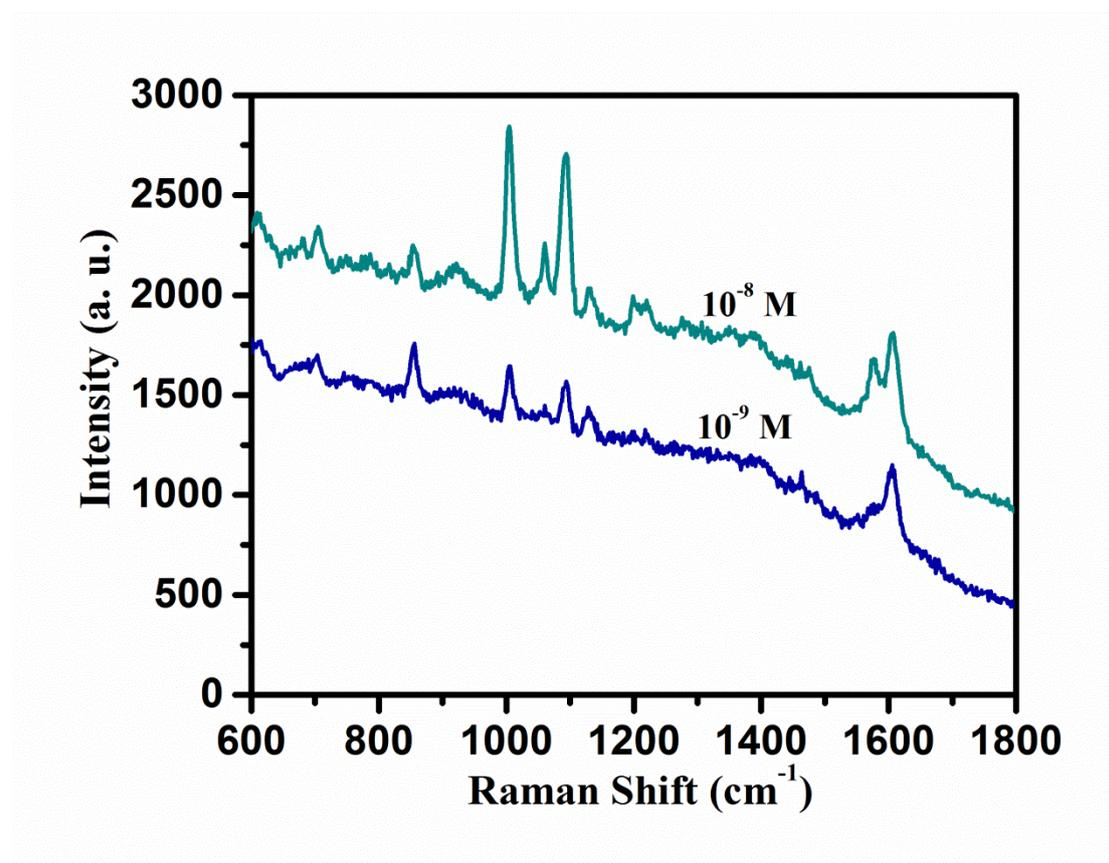
**Fig. S8** SERS spectra of 4-MPY solution  $10^{-8}$  and  $10^{-9}$  M on a AgNPs-deposited SERS membrane.
