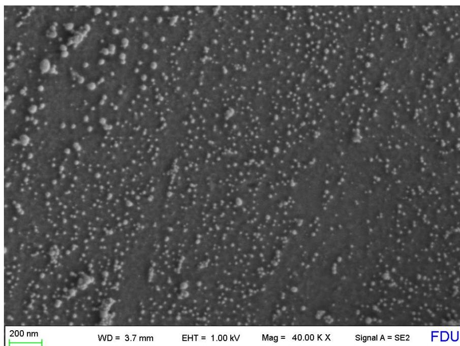
**Fig. S6** SEM image of the AgNPs-deposited glass slide, which was pretreated with 0.01 M NaOH for 2 h.
