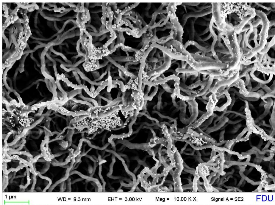
**Fig. S3** SEM image of the AgNPs-deposited SiO<sub>2</sub> NW membrane without annealing treatment to remove the C<sub>18</sub> alkyl groups from the as-prepared SiO<sub>2</sub> NWs.
