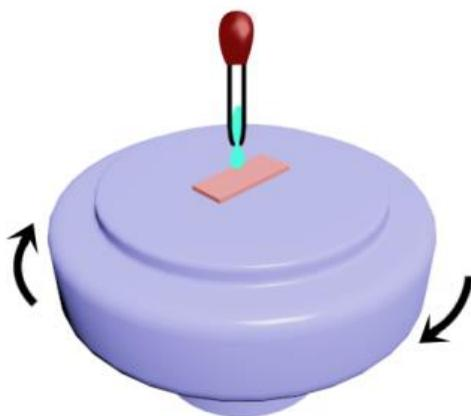
**Fig. S2** The experimental setup used to assemble the Scotch tape-supported SiO<sub>2</sub> NW film.
