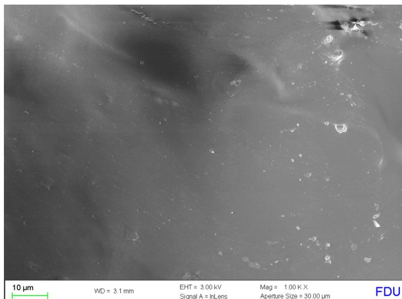
**Fig. S9** SEM image of the sticky side of the Scotch tape.
