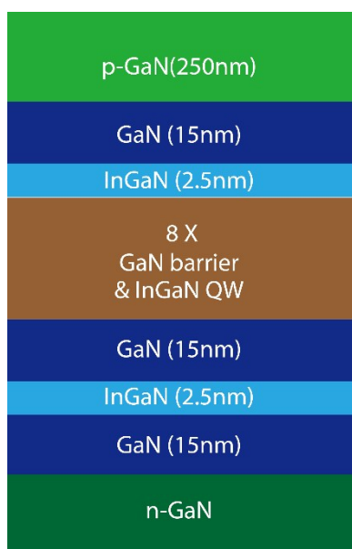
Figure S1. Layer description of the planar sample InGaN/GaN MQW (InGaN QWs with 18% In content).
