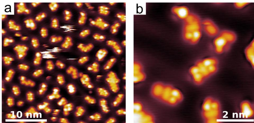
**Figure S2.** STM images of a low coverage sample of AMC on Au(111). Crown molecules assemble into small clusters of different size and shape. Since the first stages of deposition no order can be observed in the AMC assembly. Image parameters: (a, b)  $V_s = -0.2$  V,  $I_t = 0.02$  nA.
