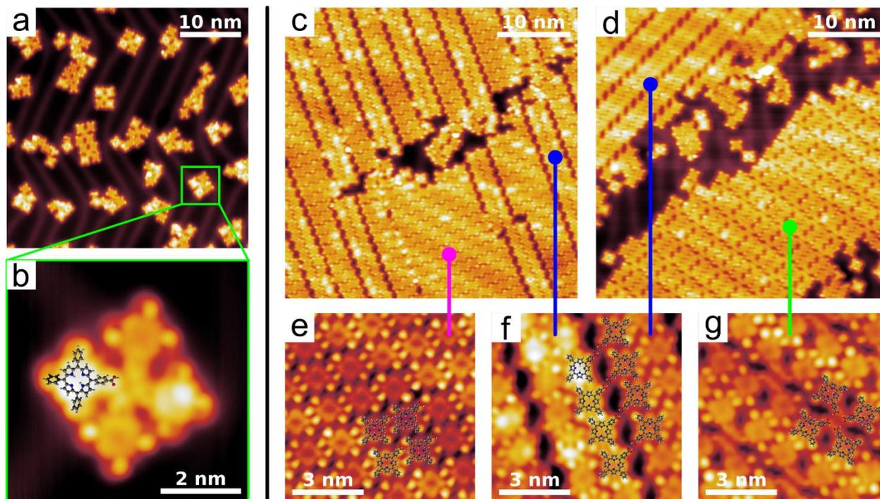
**Figure S3.** STM images of CTPP on Au(111) at low (a-b) and high coverage (c-g). (a) At low coverage, CTPP assembles in complexes of (b) four molecules via their carboxylic terminations, which can be easily identified because of their flatter appearance compared to the phenyls. The latter (b) resembles the high coverage phase in (g). (c-d) Large images showing the three coexisting different phases of the self-assembly of CTPP. The relative
