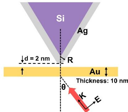
**Fig. S1** Calculation model for TERS
