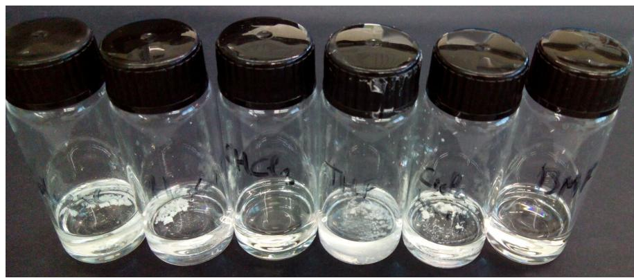
**Fig. S4.** P2HEB solubility in different solvents has been evaluated. From left to right: hexane, toluene, chloroform, tetrahydrofuran (THF), cyclohexane and dimethylformamide (DMF). Best solvents are chloroform and DMF.
