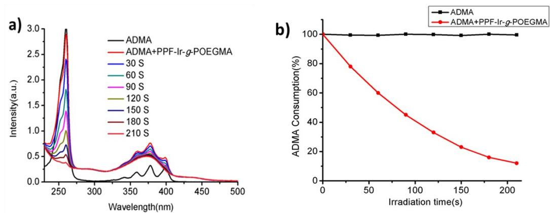
**Fig. S12** (a) Absorption spectra of ADMA (10 µg/mL) with PPF-Ir-g-POEGMA (0.1 mg/mL) in water under white light irradiation with power density 300 mW/cm<sup>2</sup> for different times (0-210 s). (b) Absorbance of ADMA at 259 nm as function of irradiation time under different irradiation intensity.
