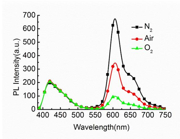
**Fig. S9** PL spectra of PPF-Ir-g-(POEGMA-*b*-PGal) aqueous solution under N<sub>2</sub>, air, and O<sub>2</sub>.
