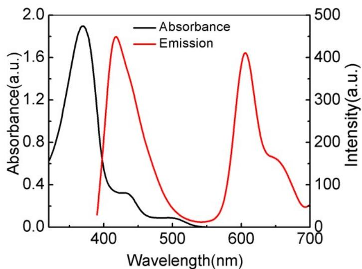
**Fig. S11** UV-vis-absorbance and fluorescent spectra of PPF-Ir-g-POEGMA in aqueous solution (1.0 mg/mL).
