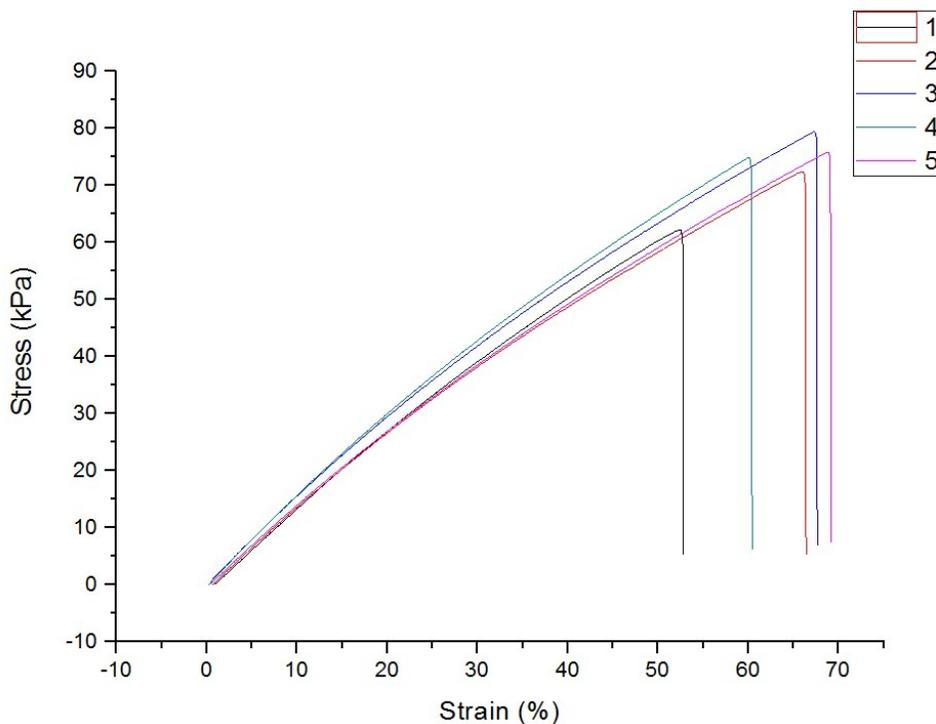
**Figure S10.** Tensile test (with a crosshead speed of 10mm/min) of the vitrimer network prepared with 5 eq. / polymer chain of bis-vinylous urethane crosslinker **2**. "Dumbbell" shape specimen of 10 mm × 2 mm with a thickness of approximately 2 mm.
