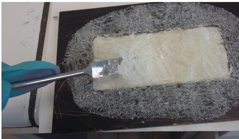
**Figure S3.** Photograph of the material obtained after pressing the network containing 5 eq. of bisacrylate-PEG crosslinker **3** in heated press for 1 h at 100°C with 3 tons of pressure. The resulting material is brittle and full of fractures.
