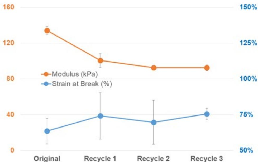
**Figure S11.** Evolution of the mechanical properties over three remolding cycles of a vitrimer network prepared with 5 eq. / polymer chain of bis-vinylogous urethane crosslinker **2**. Same test parameters as Fig. S10.
