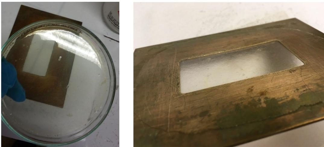
**Figure S2.** Photograph of 5 eq. network material after solution casting (left) and after subsequent remolding in Carver heated press for 1 h at 100°C with 3 tons of pressure (right) to a thickness of approximately 1.8 mm.
