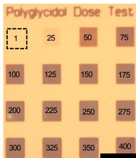
**Figure S3.** Left: Bright field microscopy image of semi-branched polyglycidol dose test from 1-400  $\mu\text{C}/\text{cm}^2$  captured at 20 x magnification. black bar represents 20  $\mu\text{m}$ .
