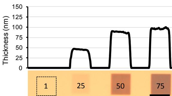
**Figure S4.** Atomic force microscopy plot (top) which indicates crosslinked polyglycidol film thickness post-development at varying electron beam irradiation doses ( $\mu\text{C}/\text{cm}^2$ ). Corresponding dose squares (bottom) were captured with a bright field microscope equipped with a camera, and the black bar represents 10  $\mu\text{m}$ .
