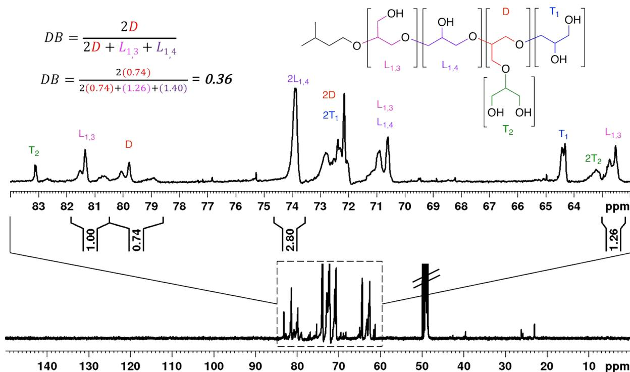
**Figure S1:** Full labeled inverse-gated  $^{13}\text{C}$ -NMR (600 MHz) spectrum of semi-branched polyglycidol homopolymer in deuterated methanol with inset (top) of 62-84 ppm region. Relaxation time ( $D_1$ ) was 10 sec, and number of scans (NS) was 1024. Degree of branching was calculated as 0.36 (semi-branched) based on relative integration values of dendritic units (D) compared with linear backbone units ( $L_{1,3}$ ,  $L_{1,4}$ ) as described in the literature.<sup>1 2 3 4</sup>
