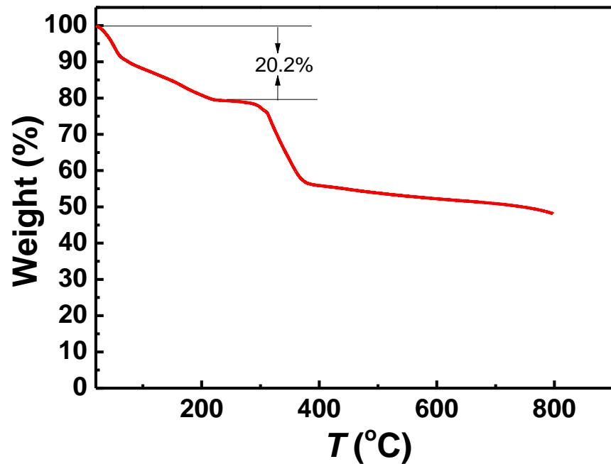
**Fig. S2** TGA curve of the as-synthesized **ZJNU-62** under  $\text{N}_2$  atmosphere
