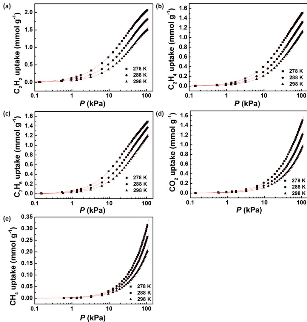
**Fig. S7** Comparison of the pure-component isotherm data for (a)  $\text{C}_2\text{H}_2$ , (b)  $\text{C}_2\text{H}_4$ , (c)  $\text{C}_2\text{H}_6$ , (d)  $\text{CO}_2$ , and (e)  $\text{CH}_4$  in **ZJNU-62a** with the fitted isotherms (shown by continuous solid lines) at 278 K, 288 K and 298 K.
