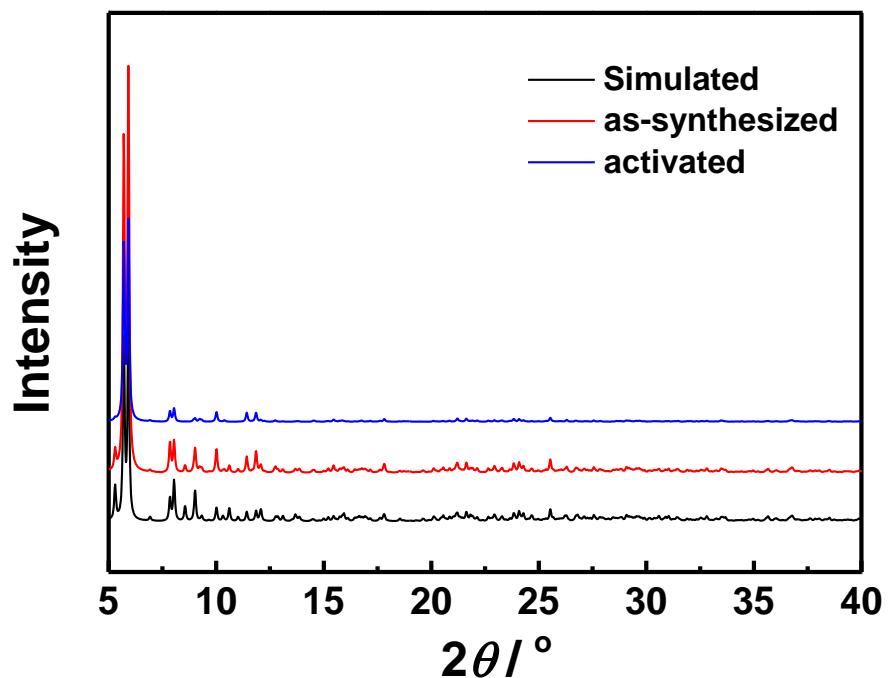
**Fig. S1** PXRD patterns for as-synthesized **ZJNU-62** (red) and activated **ZJNU-62a** (blue) together with the simulated one (black).
