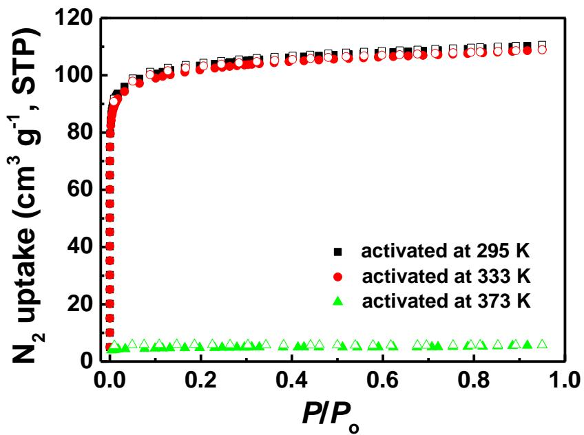
**Fig. S4** N<sub>2</sub> adsorption-desorption isotherms at 77 K of **ZJNU-62** after activation under dynamic vacuum at 295 K, 333 K and 373 K. The solid and open symbols represent adsorption and desorption, respectively. STP = standard temperature and pressure.
