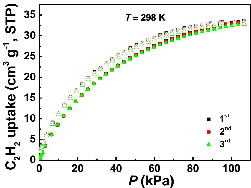
**Fig. S6** Three cycles of  $\text{C}_2\text{H}_2$  isotherms at 298 K of **ZJNU-62a**. The reactivation process was not applied between each run. The solid and open symbols represent adsorption and desorption, respectively. STP = standard temperature and pressure.
