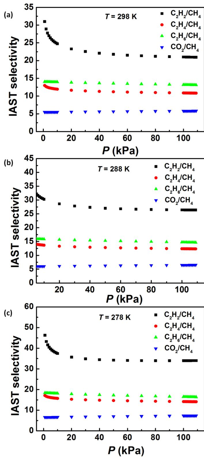
**Fig. S9** The IAST-predicted adsorption selectivities for the equimolar  $\text{C}_2\text{H}_2/\text{CH}_4$ ,  $\text{C}_2\text{H}_4/\text{CH}_4$ ,  $\text{C}_2\text{H}_6/\text{CH}_4$  and  $\text{CO}_2/\text{CH}_4$  gas mixtures at 298 K (a), 288 K (b) and 278 K (c).
