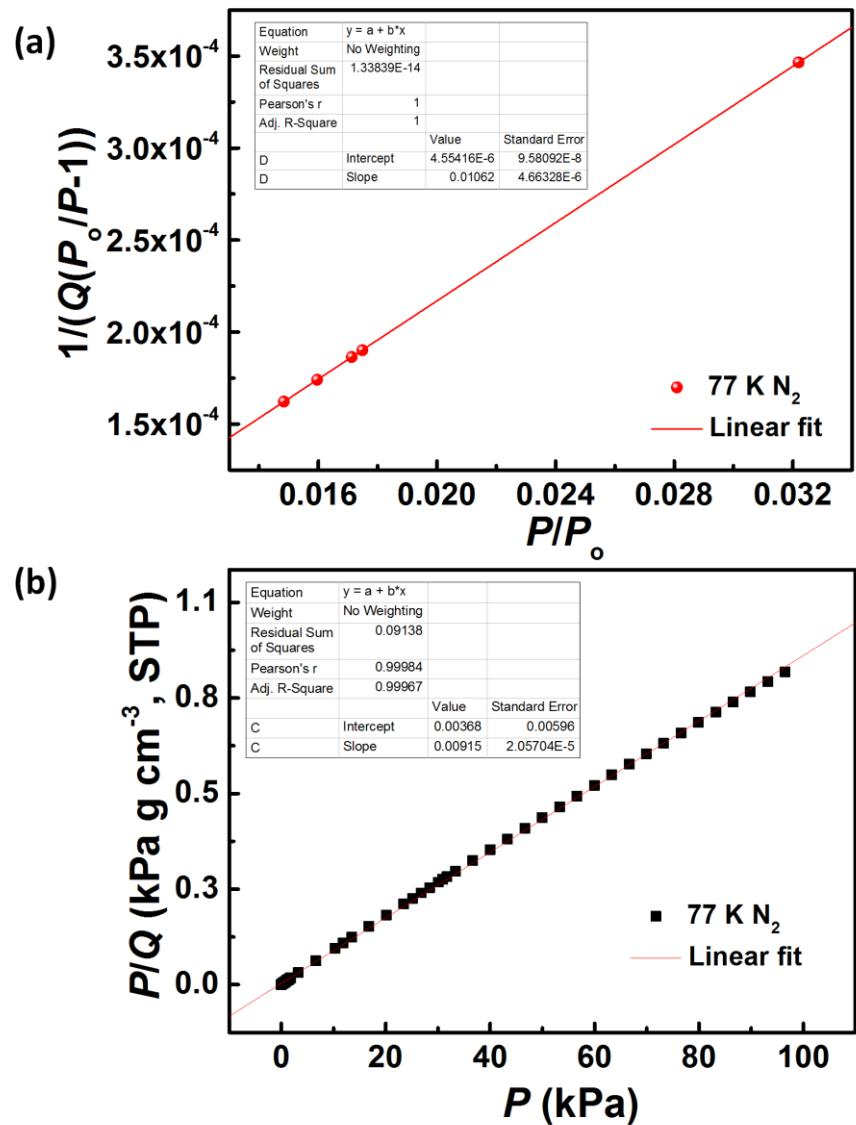
$$S_{\text{BET}} = 1 / (4.55416 \times 10^{-6} + 0.01062) / 22414 \times 6.023 \times 10^{23} \times 0.162 \times 10^{-18} = 410 \text{ m}^2 \text{ g}^{-1}$$
