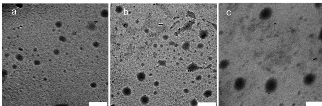
**Figure S20** TEM images of nanoparticles for compounds **1** in different water / THF (fw) and the concentration is  $2 \times 10^{-5}$  mol/L. (a) fw = 95%, (b) fw = 85%, (c) fw = 80%. Scale bar = 200nm.
