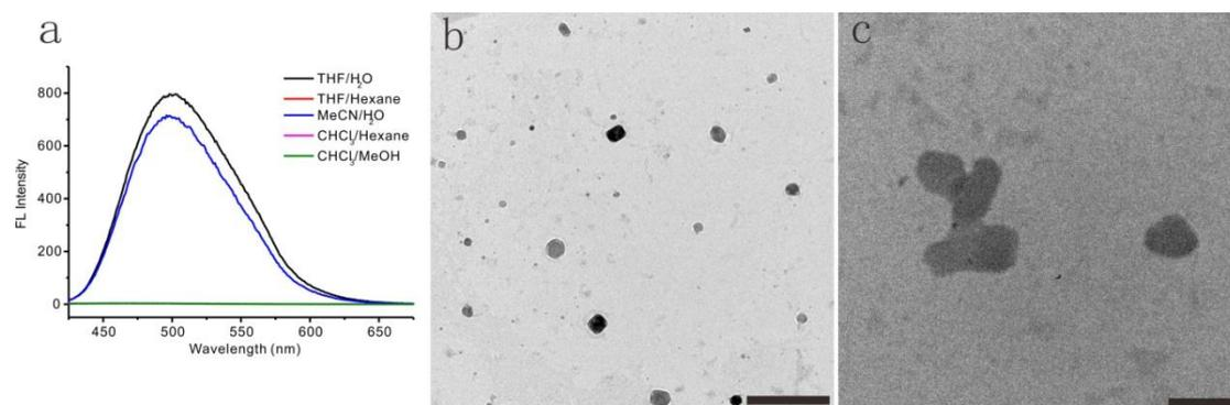
**Figure S17** Fluorescence spectra and TEM images of compound **2** in different kinds of complex, the concentration is  $2 \times 10^{-5}$  mol/L. (a) Emission of compound **2** in different complex (fp = 95%, p = Poor solvent), (b) **2** in Water / THF (fw = 95%, scale bar = 500 nm), (c) **2** in Water / Acetonitrile, (fw = 95%, scale bar = 200 nm).
