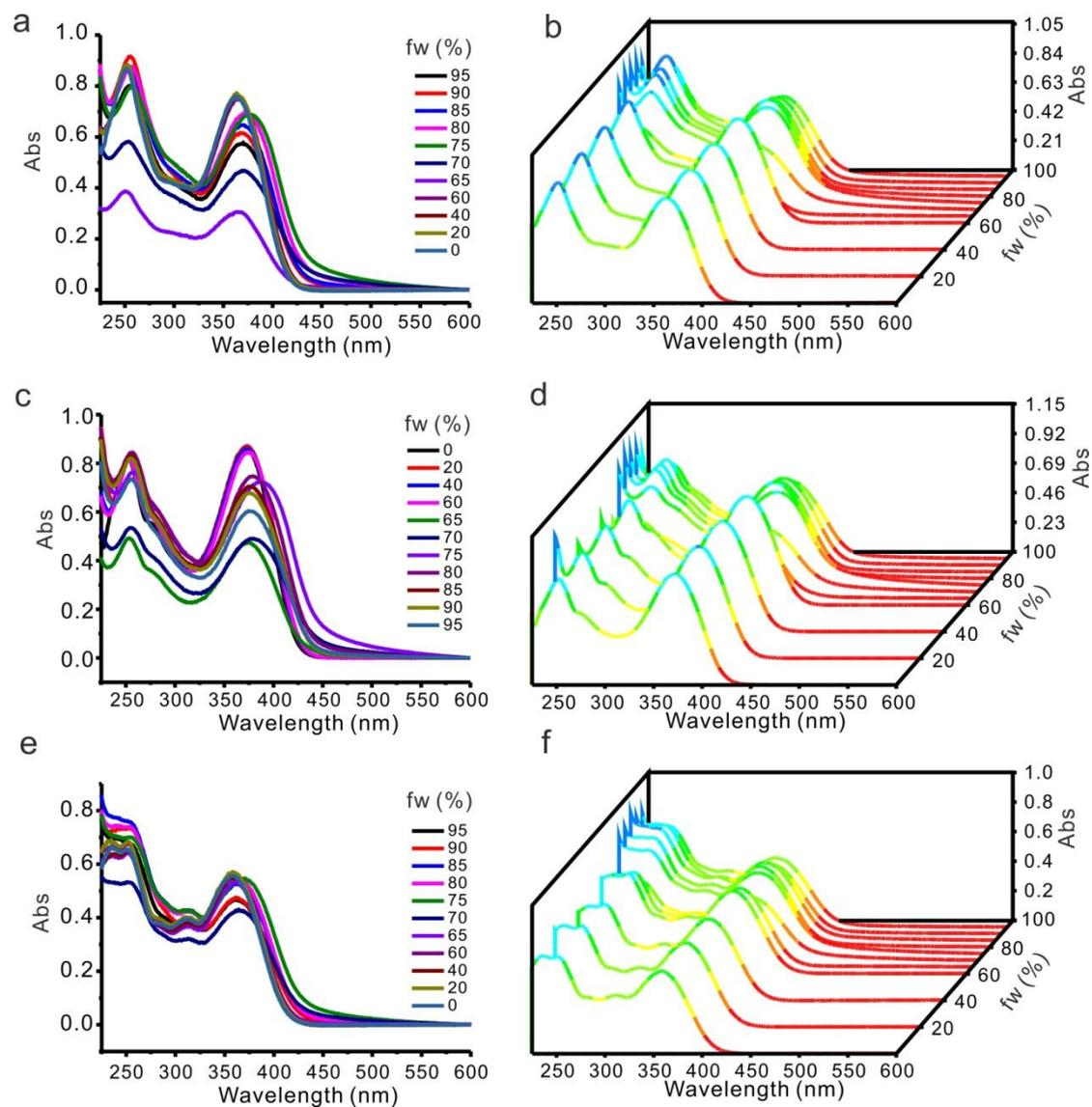
**Figure S23** Absorption of compound **1**, **2**, **3** in different water / THF (fw). (a), (c), (e) 2D diagram of absorption of compound **1**, **2**, **3** at varying  $f_w$ , respectively; (b), (d), (f) 3D diagram of absorption of compound **1**, **2**, **3** at varying  $f_w$ , respectively.
