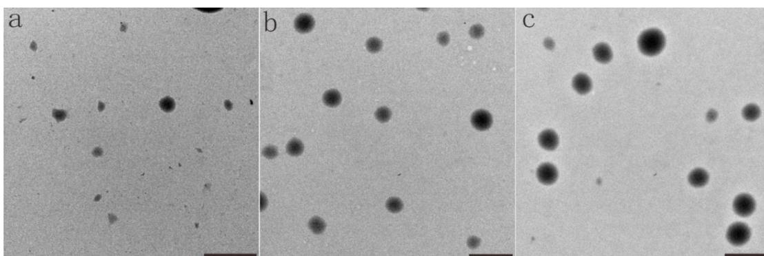
**Figure S22** TEM images of nanoparticles for compounds **3** in different water / THF (fw) and the concentration is  $2 \times 10^{-5}$  mol/L. (a) fw = 95%, (b) fw = 85%, (c) fw = 80%. Scale bar = 1  $\mu$ m.
