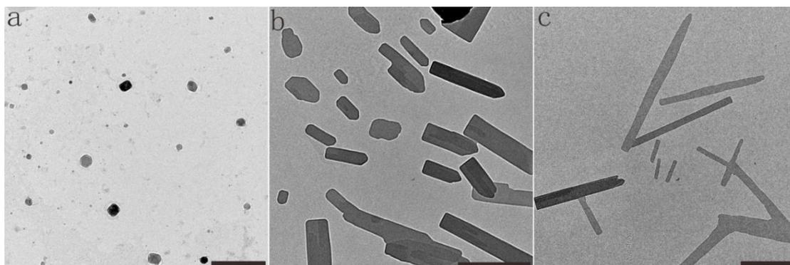
**Figure S18** TEM images of compound **2** in Water / THF ( fw = 95% ), the concentration is different. (a)  $C = 2 \times 10^{-5}$  mol/L, scale bar = 500 nm; (b)  $C = 1 \times 10^{-4}$  mol/L, scale bar = 1  $\mu\text{m}$ ; (c)  $C = 1 \times 10^{-3}$  mol/L, scale bar = 2  $\mu\text{m}$ .
