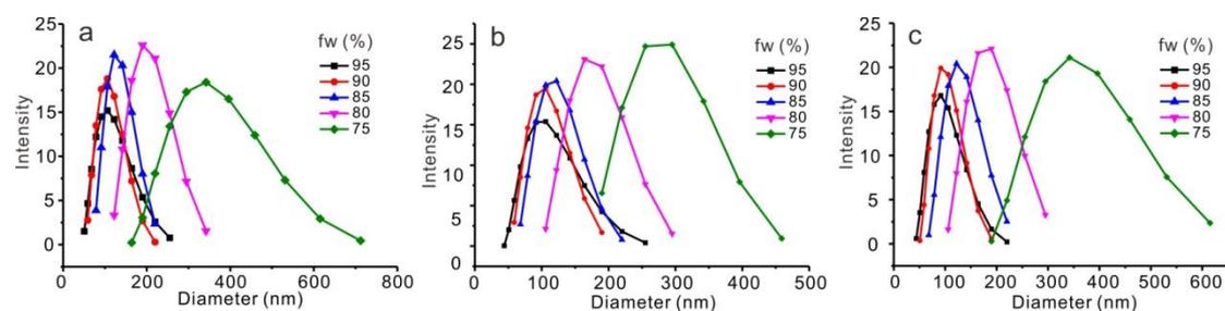
**Figure S19** The size distribution of nanoparticles in different water / THF (fw) by DLS. (a) nano-particles size distribution of compounds **1**, (b) nano-particles size distribution of compounds **2**, (c) nano-particles size distribution of compounds **3**.
