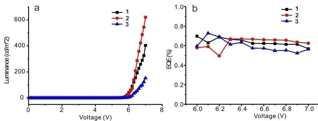
**Figure S30** Voltage–luminance and EQE. (a) Voltage – Luminance curve, (b) Voltage – EQE curve. **1**, **2**, **3** represents compound **1**, **2**, **3**, respectively.
