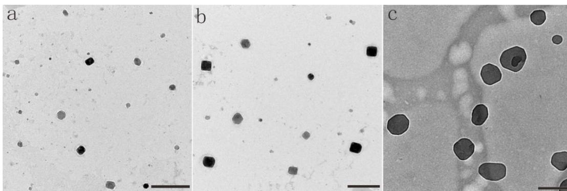
**Figure S21** TEM images of nanoparticles for compounds **2** in different water / THF (fw) and the concentration is  $2 \times 10^{-5}$  mol/L. (a) fw = 95%, (b) fw = 85%, (c) fw = 80%. Scale bar = 500 nm.
