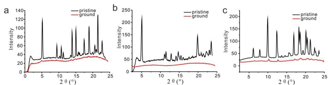
**Figure S26** XRD before and after grinding of compound **1**, **2**, **3**. (a) compound **1**, (b) compound **2**, (c) compound **3**.
