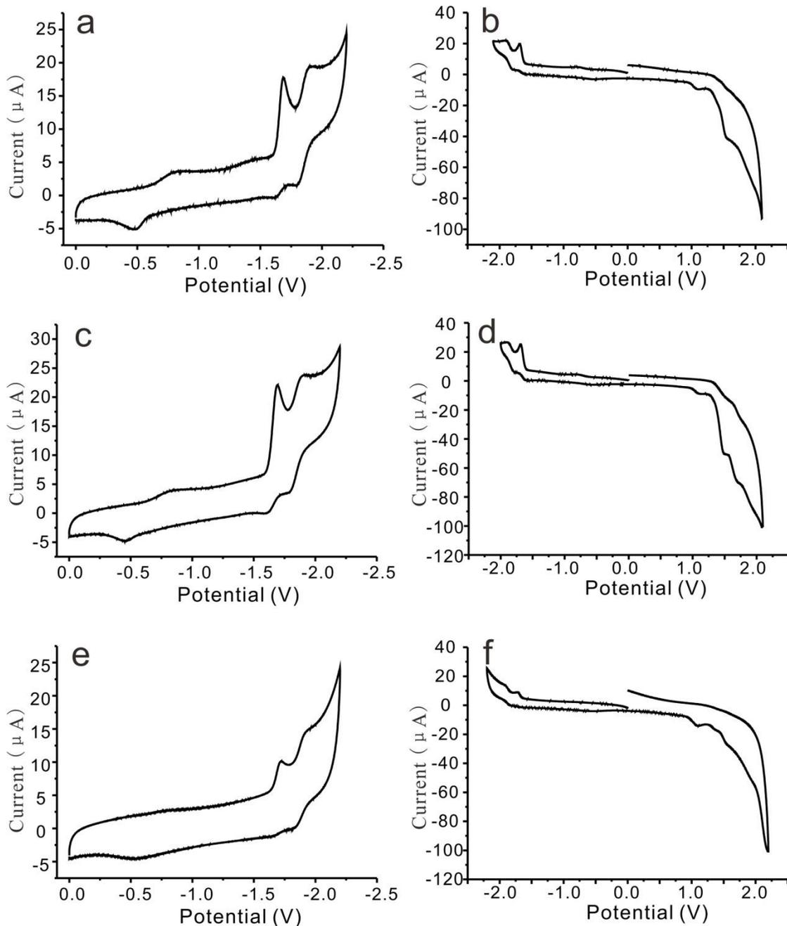
**Figure S27** Cyclic voltammograms of compounds **1**, **2**, and **3**. (a), (c), (e) only negative voltage part of compound **1**, **2**, **3** respectively, (b), (d), (f) whole CV curve of compound **1**, **2**, **3** respectively.
