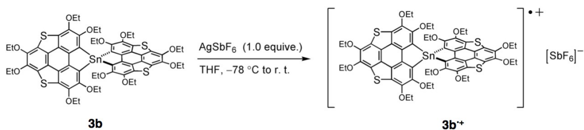
Scheme S1 Chemical oxidation of 3b using AgSbF 6 as an oxidant.
