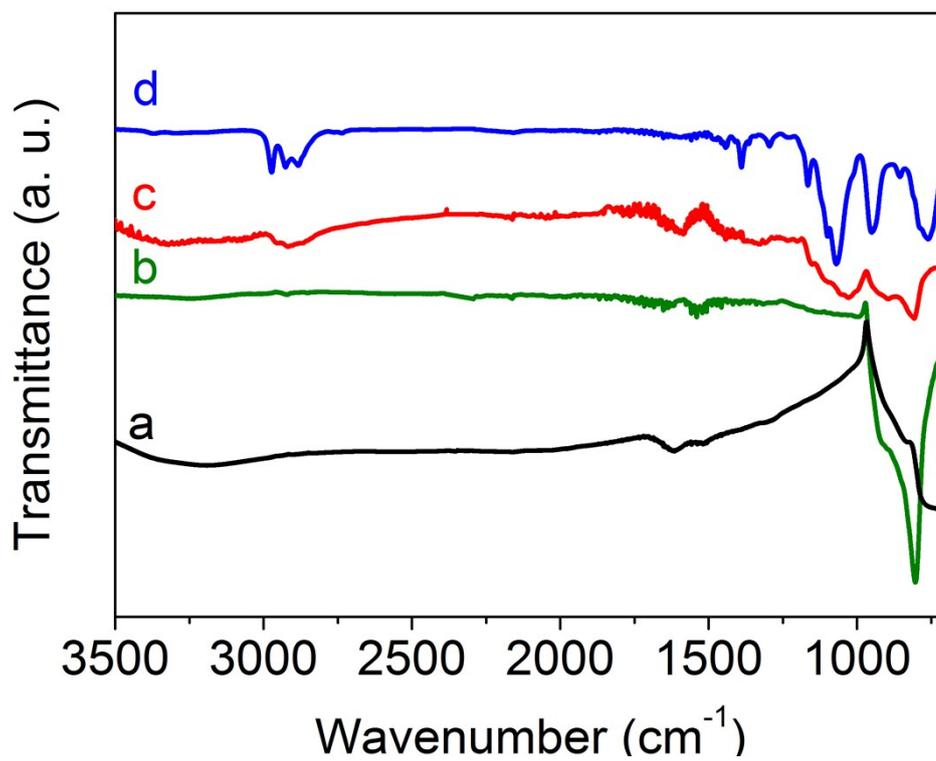
**Fig. S2.** Full infrared transmission spectra of KOH treated (a), APTES-1 (b), APTES-2 modified SiC nanoparticles (c) and APTES (d).
