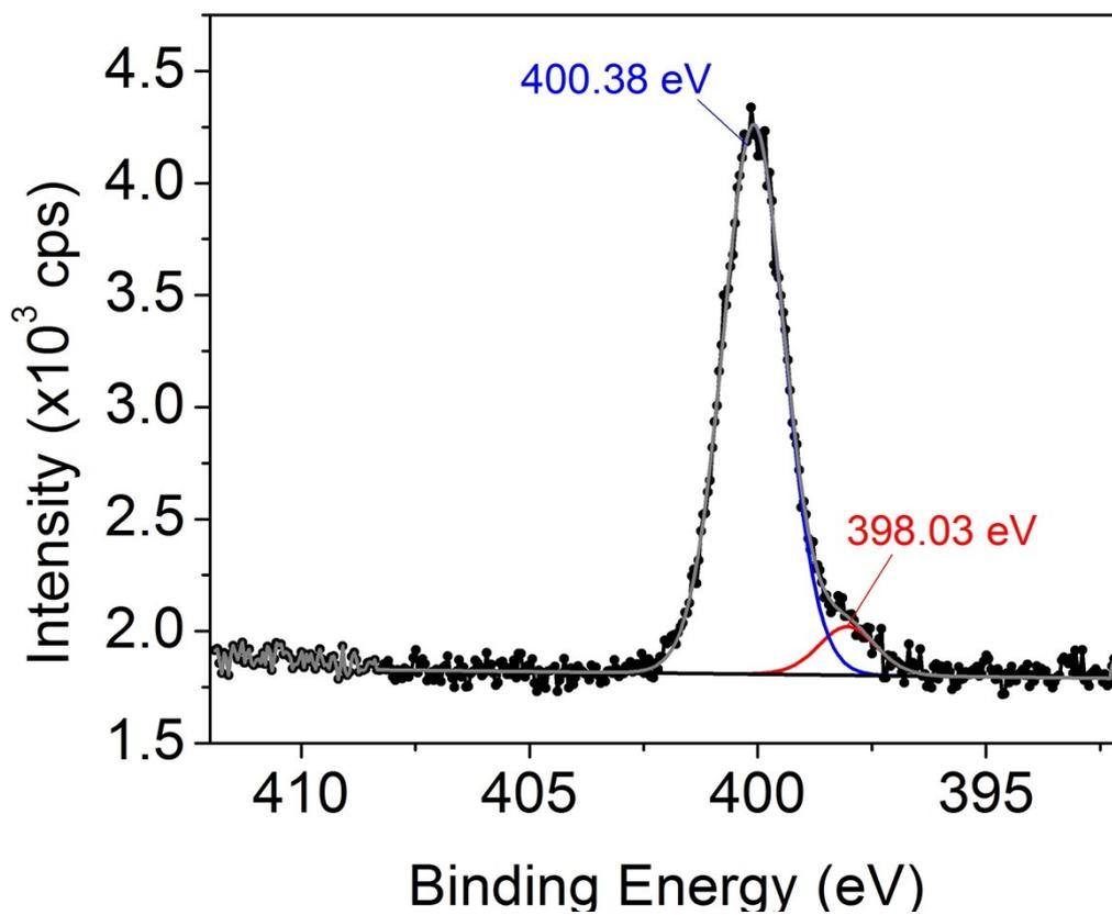
**Fig. S3.** N1s level XPS spectrum of APTES-2 modified SiC nanoparticles.
