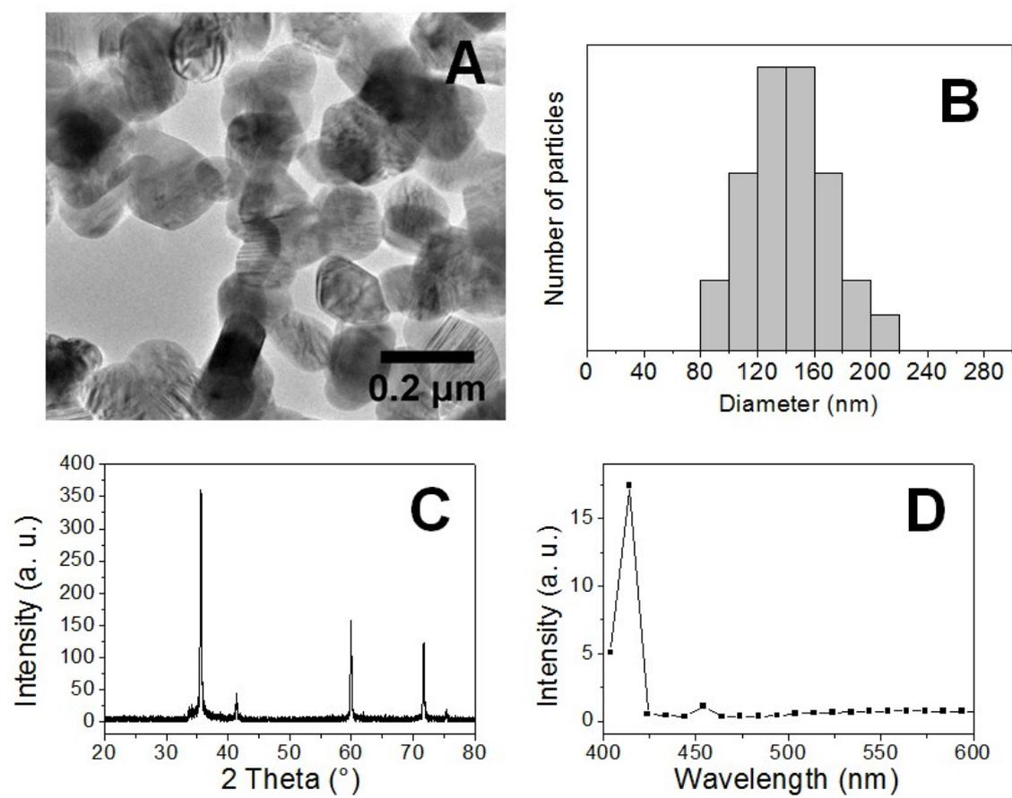
**Fig. S1.** TEM image (A), corresponding size histogram (B), XRD diffractogram (C) and SHG emission spectra at 820 nm excitation (D) of KOH treated SiC nanoparticles.
