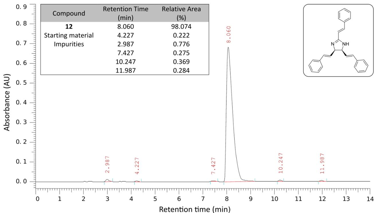
**Fig. S107** Chromatogram of **12** after recrystallisation at 250 nm with the table of peaks and the structure in insert. The compound was monitored with Method 1.
