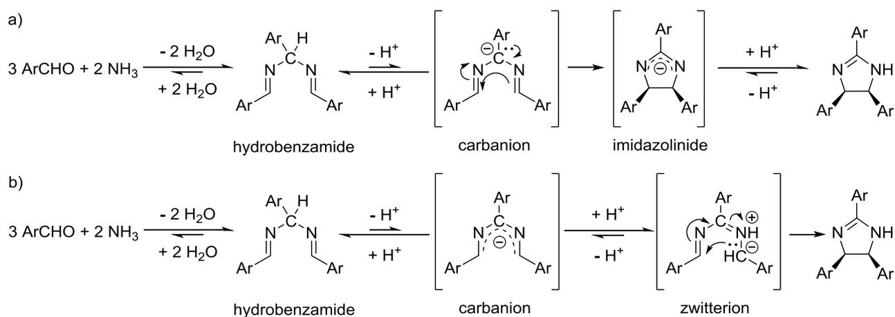
**Scheme S1** (a) Earlier proposed mechanism of the reaction between aromatic aldehydes[4] and an ammonia source and (b) the mechanism found in this work.
