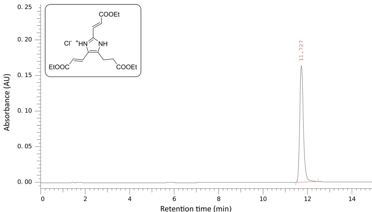
**Fig. S110** Chromatogram of **13** at 250 nm with the structure in insert. The compound was monitored with Method 2.
