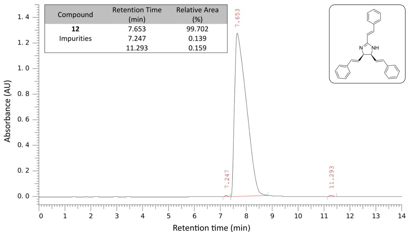
**Fig. S108** Chromatogram of **12** after preparative HPLC purification at 250 nm with the table of peaks and the structure in insert. The compound was monitored with Method 1.
