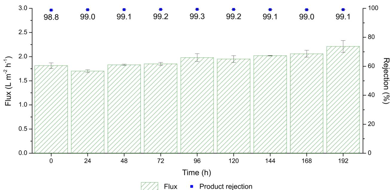
**Fig. S118** Long term stability of Duramem 300 membrane at 20 bar.
