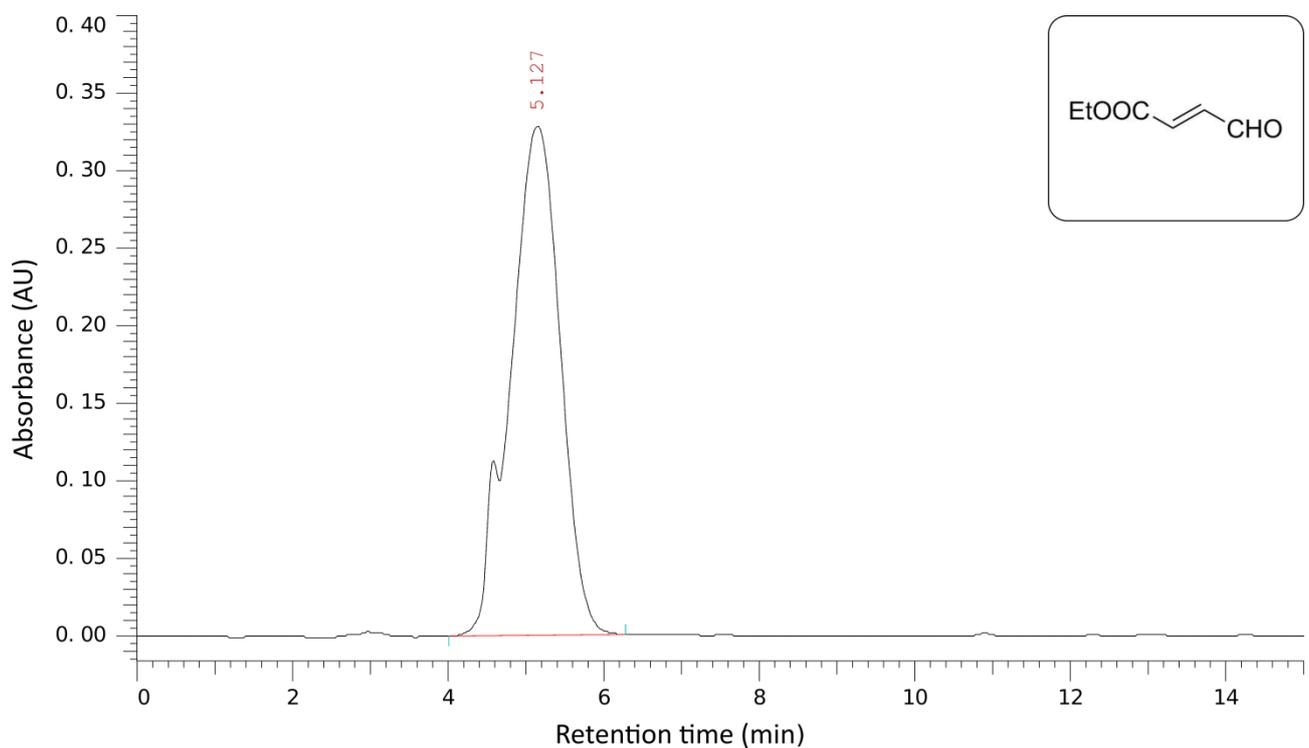
**Fig. S109** Chromatogram of ethyl 4-oxobut-2-enoate at 250 nm with the structure in insert. The compound was monitored with Method 2.
