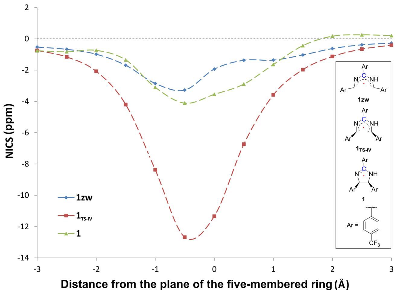
**Fig. S113** NICS values calculated in function of distance from the plane of the five-membered ring in **1zw**, **1<sub>TS-IV</sub>** and **1**. The ghost atoms for the calculation were placed in the middle of the rings, perpendicularly to it as shown in insert. The red dots illustrate the positions of the 0 Å ghost atoms which were placed 1.19 Å away from the blue carbon atoms.
