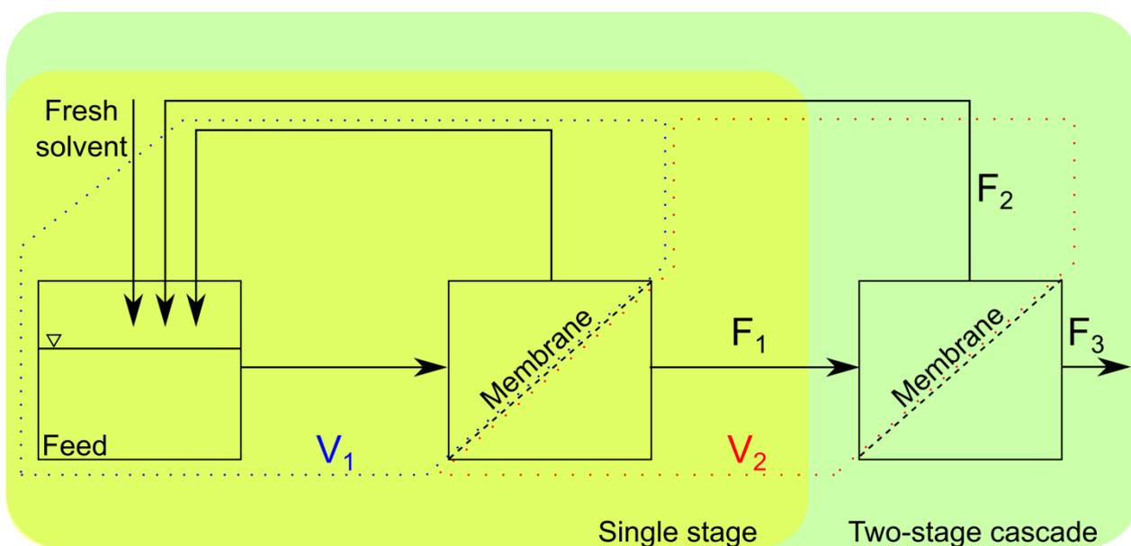
**Fig. S119** Schematic system setup used for the process modelling. The yellow and green areas show the single stage and the two-stage setups, respectively.  $F_1$  represents the permeate flow rate from the first stage, while  $F_3$  is the permeate flow rate from the second stage.  $F_2$  shows the flow rate of the recycle line from the second stage.  $V_1$  and  $V_2$  are the system volumes for the first and second stage, respectively.
