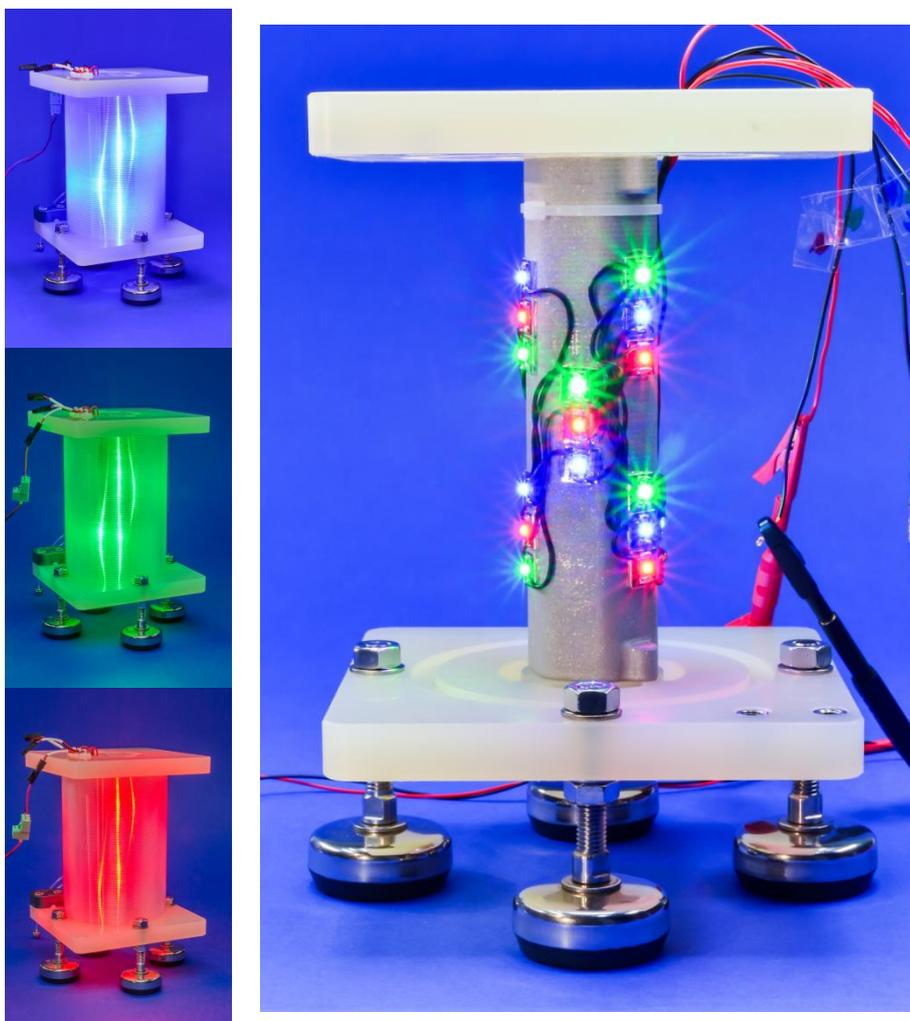
**Figure S4** 1<sup>st</sup> Generation of the capillary photoreactor with blue, green and red LED.
