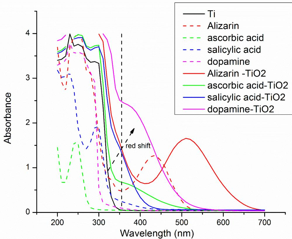
**Figure S4.** UV-vis spectra of solutions of different bidentate binding ligands, TiO<sub>2</sub> nanoparticles, and bidentate binding ligand-modified TiO<sub>2</sub> nanoparticles.
