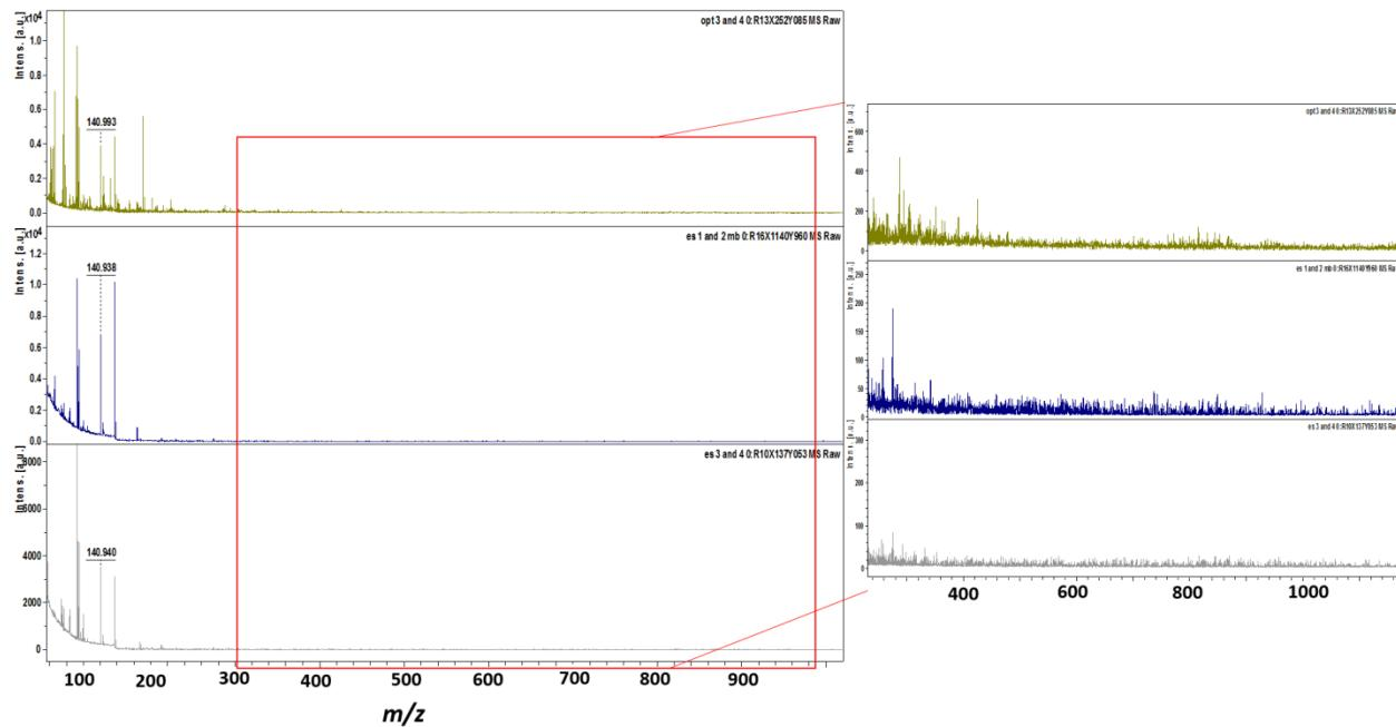
**Figure S2.** Representative mass spectra acquired from mouse brain tissues using different amounts of  $\text{TiO}_2$  nanoparticles. No lipid signals were observed when using the  $\text{TiO}_2$  nanoparticles. (top)  $100 \mu\text{g}/\text{cm}^2$ ; (middle)  $500 \mu\text{g}/\text{cm}^2$ ; (bottom)  $2000 \mu\text{g}/\text{cm}^2$ . The inset shows the enlarged spectra for  $m/z$  300–800.
