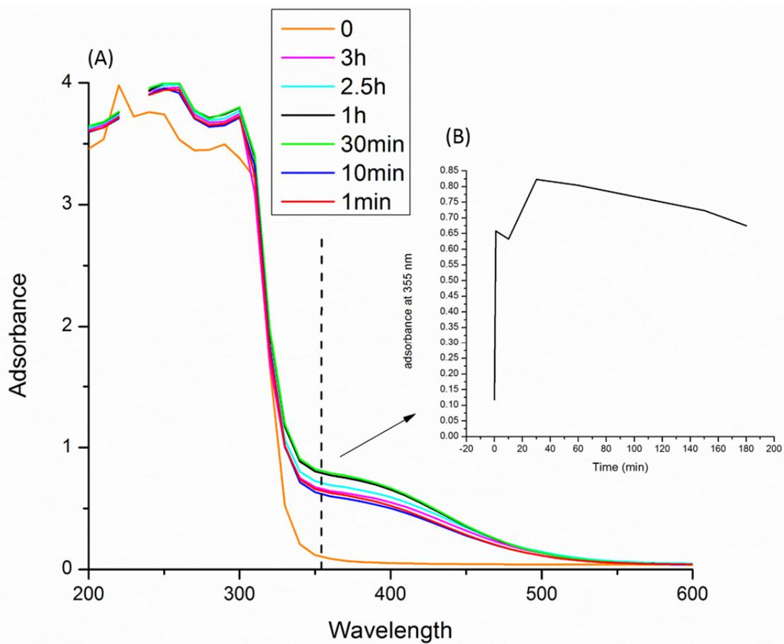
**Figure S6.** Time dependence of UV-vis absorption of  $\text{TiO}_2$ -DA particle suspensions. UV-vis absorption spectra of DA-modified  $\text{TiO}_2$  with (A) different incubation times and (B) its UV absorbance kinetic curve at a wavelength of 355 nm.
