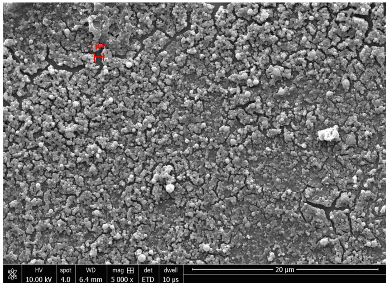
**Figure S10.** Scanning electron microscopy image of the TiO<sub>2</sub>-DA monolith surface with low magnification ( $\times 5000$ ).
