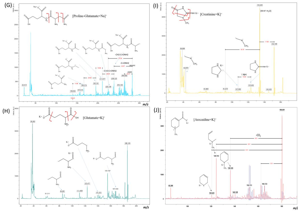
**Figure S12.** MS/MS spectra of different endogenous compounds detected in mouse brain tissues during TiO<sub>2</sub>-DA monolith-assisted LDI MSI experiments. (A) PE, phosphatidylethanolamine; (B) PC, phosphatidylcholine; (C) M(IP)2C, mannose-(inositol-P)2-ceramide; (D) DAG, diacylglycerol; (E) Cer, ceramide; (F) docosahexaenoic acid; (G) proline-glutamate; (H) glutamate; (I) creatinine; (J) arecaidine.
